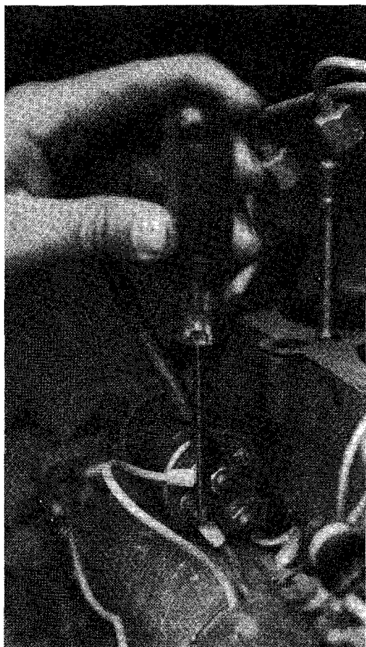
By-passing the ignition switch by jumping out the two smaller wires.
