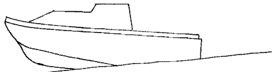
The boat is now moving at, say, 12 knots. It has moved up onto the surface of the water and ahead of its own wave formation.
