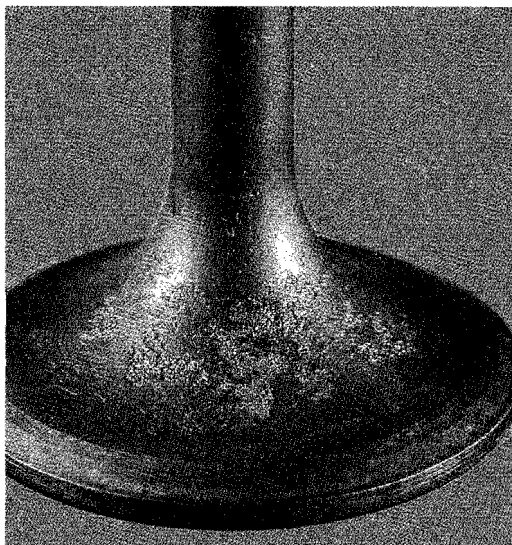
Figure 11-19. Valve failure: corrosion from moisture and acids. (Courtesy Caterpillar Tractor Co.)
