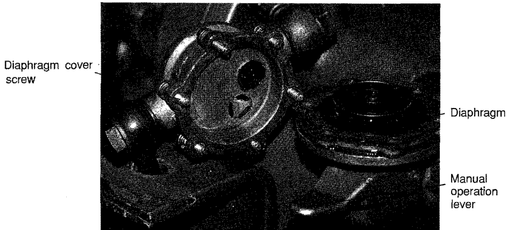
Figure 9-17. Diaphragm on a lift pump.
