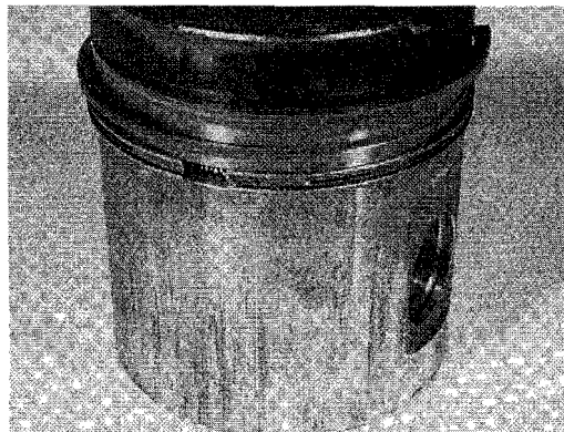
Figure 11-37. The skirt (base) of this piston has been skuffing (rubbing without lubrication) on the cylinder as a result of overheating. The skirt is beginning to break up and the piston is not re-usable. (Courtesy Caterpillar Tractor Co.)
