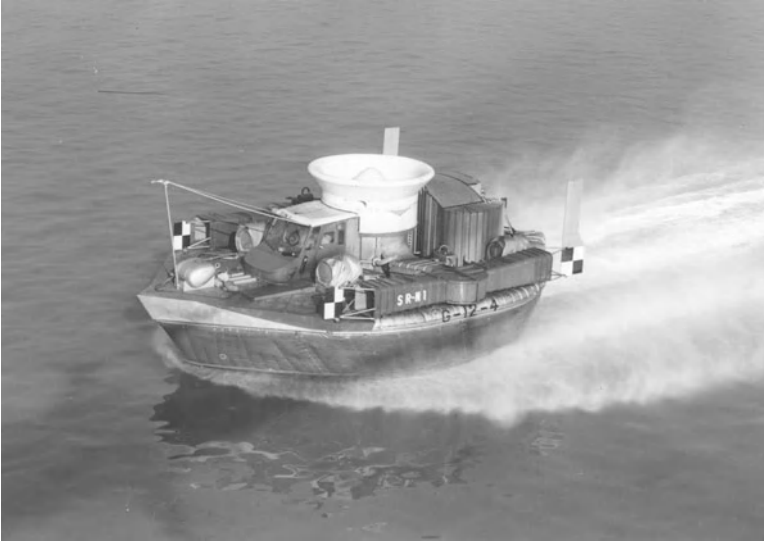
Fig. 2.4 SR-N1 deep skirt and jet propulsion
