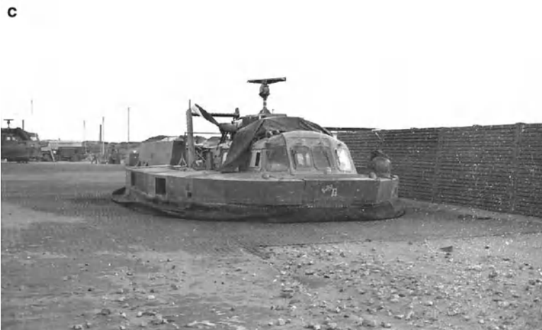
Fig. 2.22 (a) Bell SK-5 PACV. (b) SK-5 leaving USS Gunstan Hall. (c) US Army PACV showing armour protection
