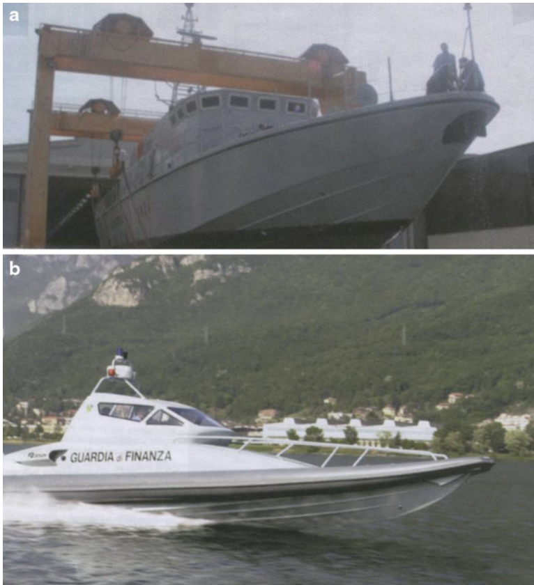
Fig. 4.8 (a) Spray rails. (b) Spray rails deep Vee craft
