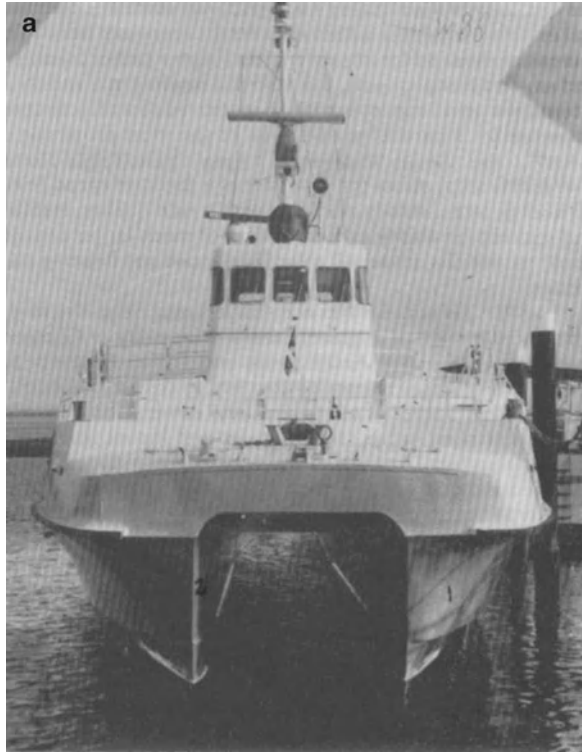
Fig. 6.3 (a) Asymmetric hulls. (b) Symmetric round bilge hulls. (c) Symmetric planing hulls
