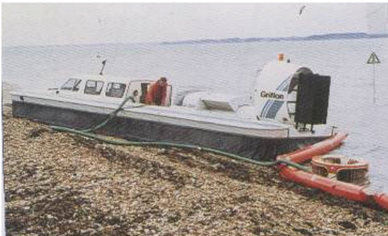
Fig. 2.38 Craft performing pollution control deploying floating containment boom
