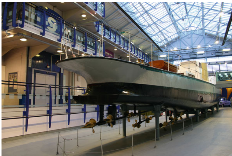
Fig. 1.7 A Stern view showing the three propellers on each of three shafts of Turbinia
