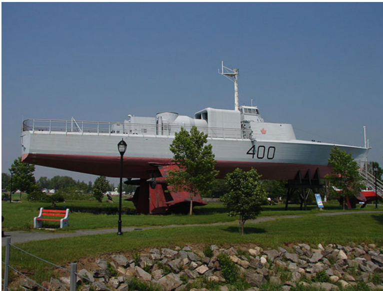
Fig. 5.10 Single main lifting foil configuration—Bras D'Or
