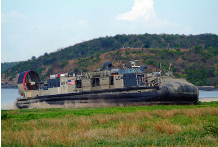
Fig. 2.43 LCAC over land showing secondary segments for spray control
