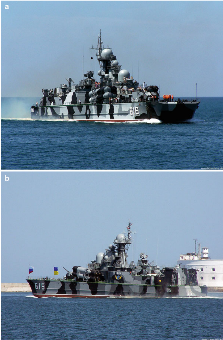
Fig. 2.64 SES Bora patrol frigate based in Russian Black Sea fleet. (a) SES Frigate Samum returning to port. (b) SES Frigate Bora leaving port
