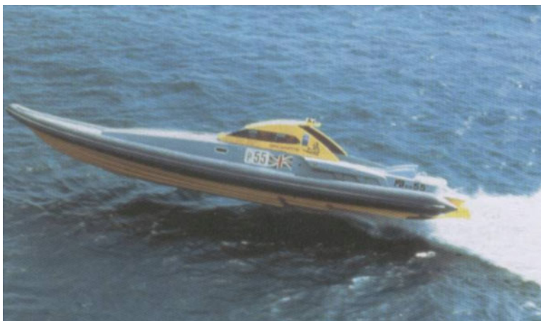
Fig. 4.9 Stepped hull craft at high speed
