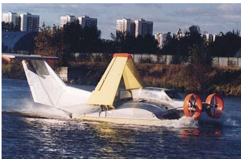
Fig. 3.21 Ivolga with wings retracted
