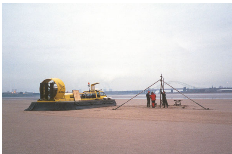
Fig. 2.42 G2000TD seismic survey on tidal sandbank, preparing a shot
