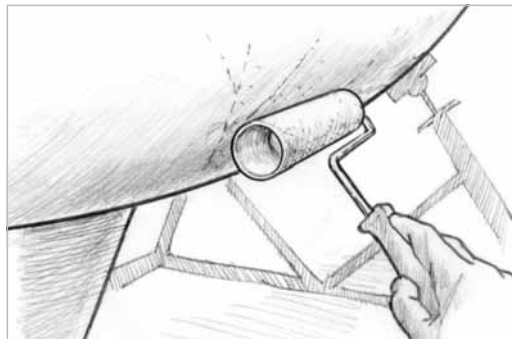
Figure 1. Apply a coat of unthickened epoxy to the hull.
