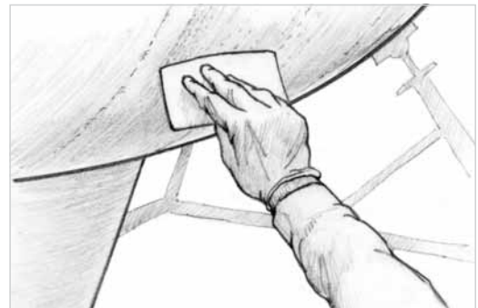
Figure 4. Use a plastic squeegee to press the fabric securely against the hull.
