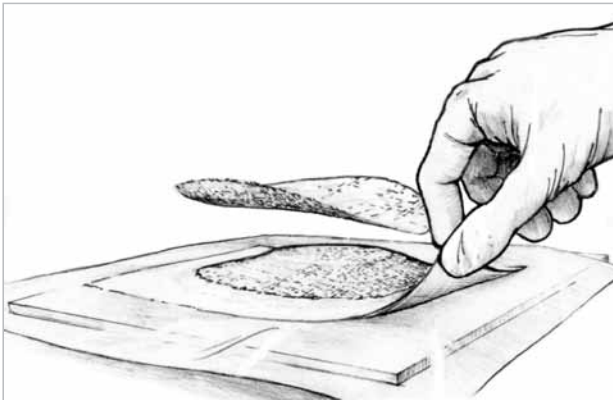
Figure 4-7 Build up a plug of wet-out fabric approximately the size, shape and depth of the hole.
