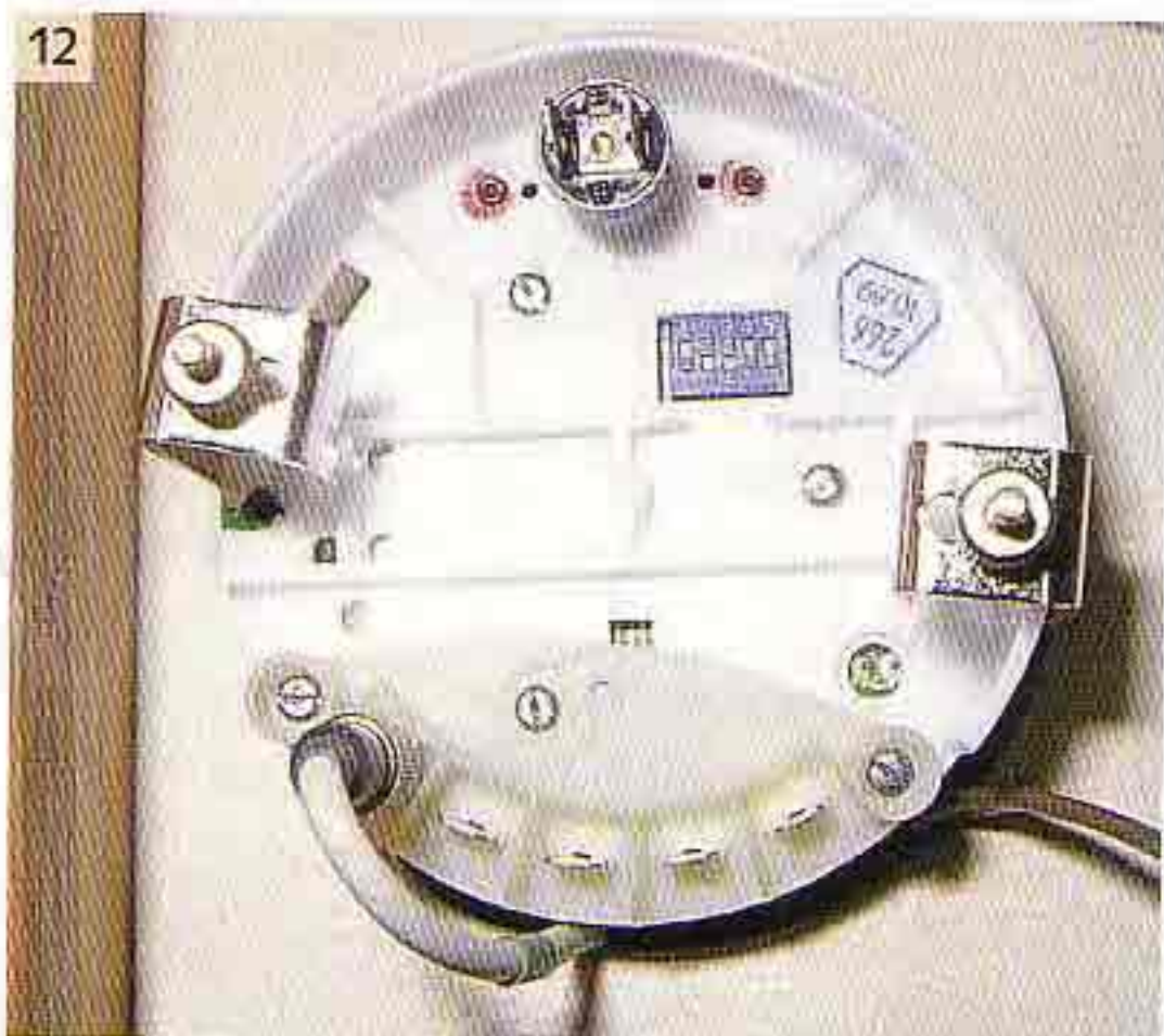
8 The connector in the lead is watertight, but it should still not be laid directly in the bilges.
