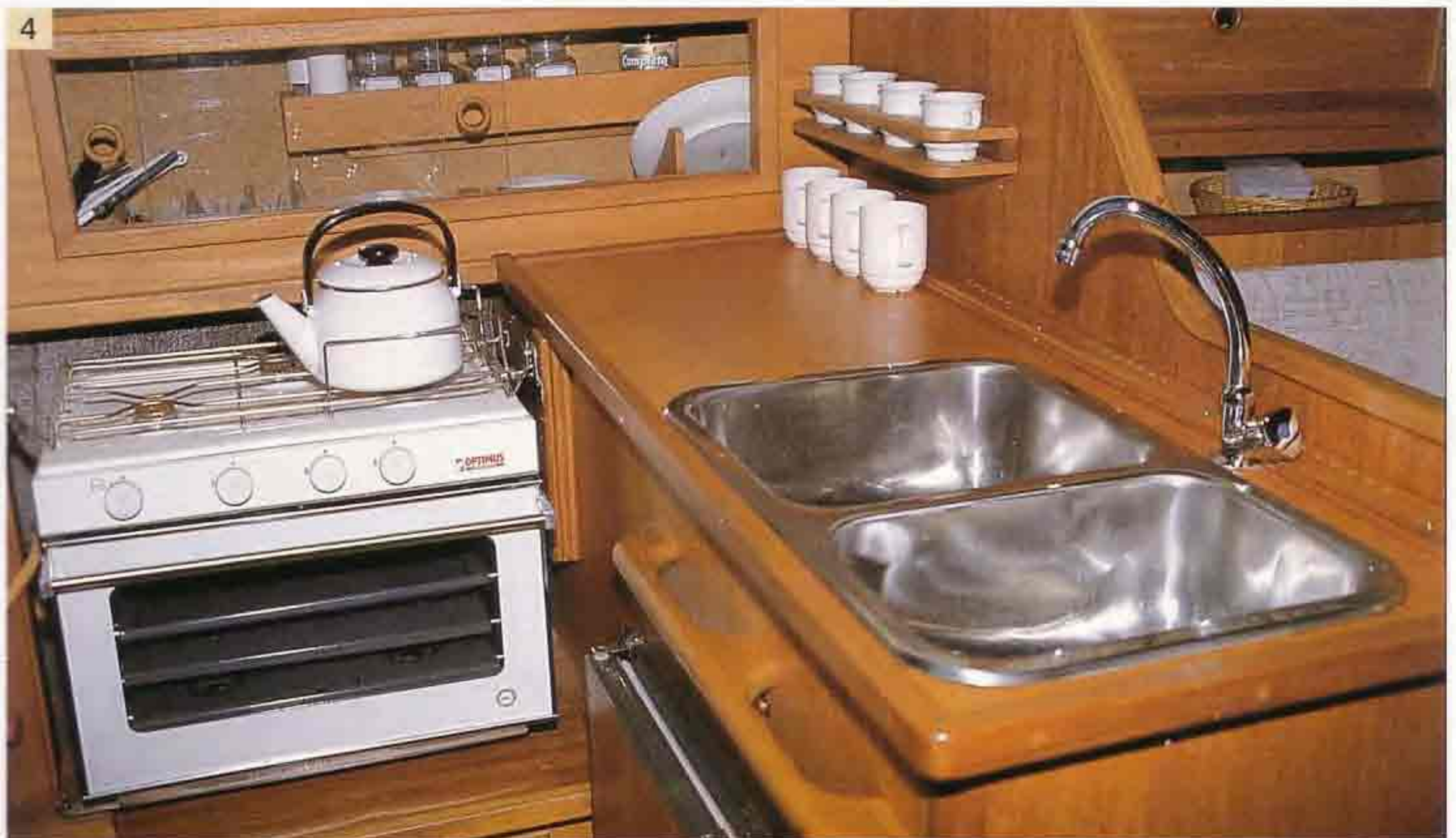
4 This is how the finished galley should look, with a double sink and a freezer fitted underneath, gimballed gas stove and dedicated stowage for crockery, cups and glasses.
