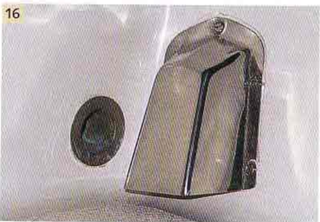
17 This is how badly sited fittings look after just one season. Corrosion caused by salt water and sea air is well advanced.
