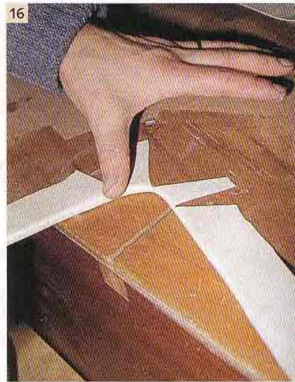
15 Radiuses (curves) are cut to shape and glued to the back. If the glue isn't holding yet, use adhesive tape for a temporary fix.
