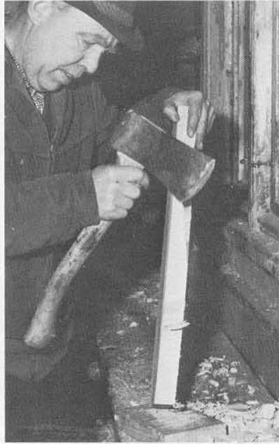
The futtock is shaped with an axe.
