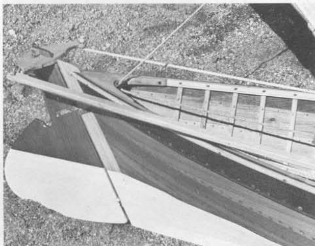
Rudder and tiller rigged and ready. Note the mizzen sheet lead.
