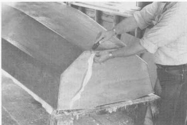
Trim the cloth overhang before your final coats of resin.
