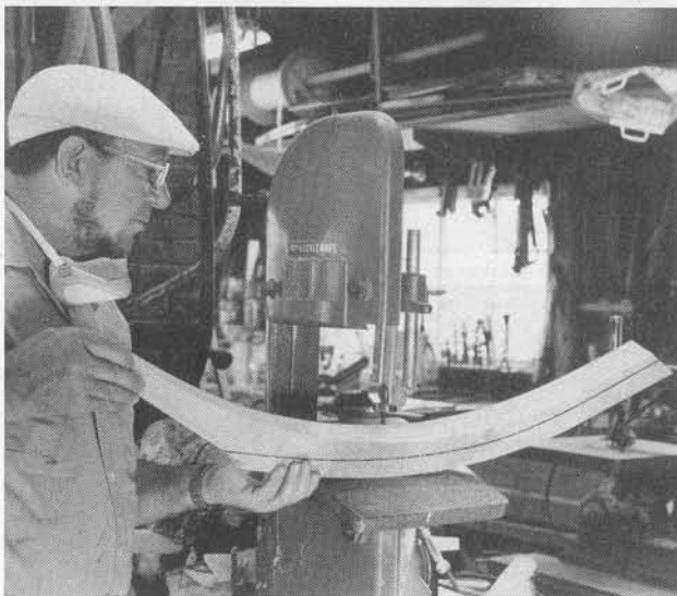
Cutting the stem bevel with a bandsaw.
