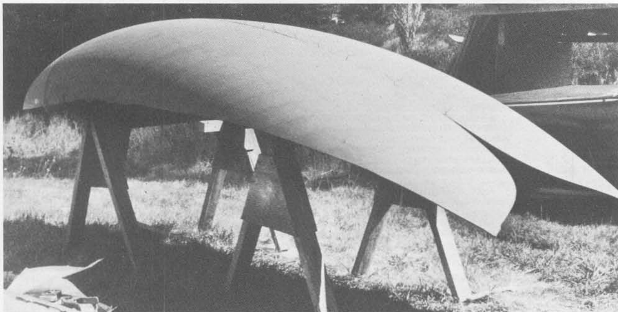
Gull's cold-molded hull will be made from these Constant Camber port and starboard panels by joining them together along the keel as shown, then "torturing" them into the shape of a boat by bringing the stem portions of the panels together.
