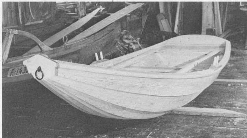
With the inwales, rubrails, thole pins, painter ring, and thwarts fitted, the pram is ready for her finish coats.
