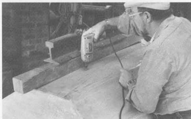
Bore from the outside for the skeg fastenings.
