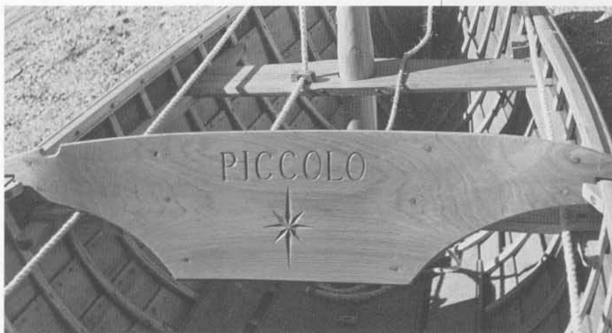
Backrests are sawn out of cedar, and four stiffeners are riveted to the after sides.
