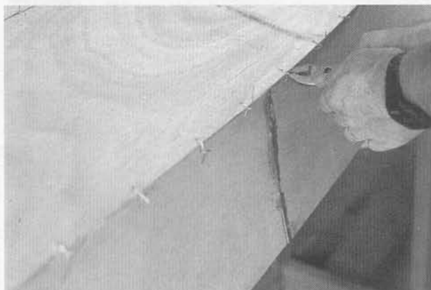
Wire the bottom panels to the sides.
