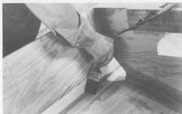
Coat the long seam fillets with resin, position the tape, and wet it out thoroughly with more resin.
