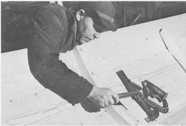
Riveting the futtock. Note the limbers just above each strake.
