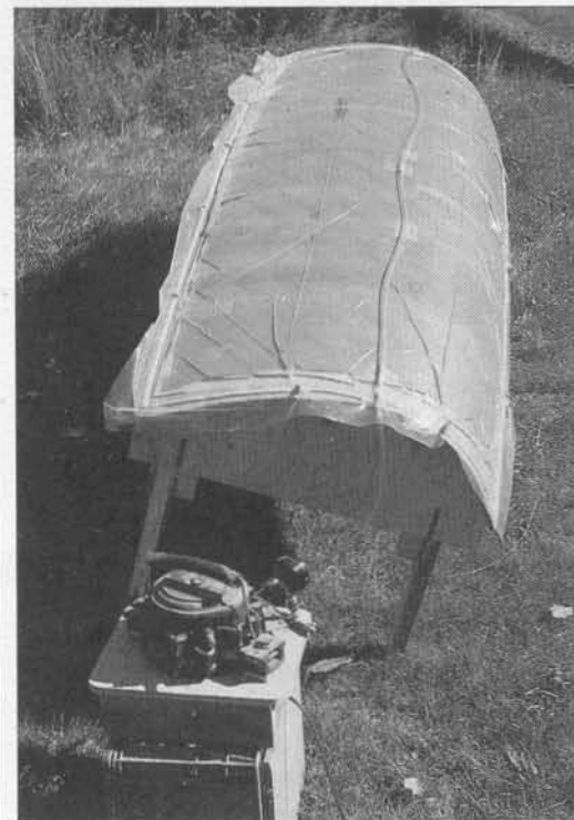
Old "fridge" compressor, scavenged for free, proudly pulls 15-inch Hg vacuum — more than enough. Note where the vacuum tube leads into the bag; Dum-Dum has been packed around here to seal.
