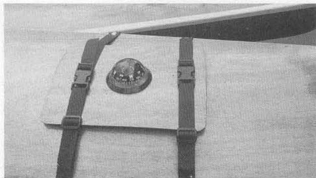
After varnishing the deck, attach the hatch hold-down straps, grab handles, compass, and other deck gear.
