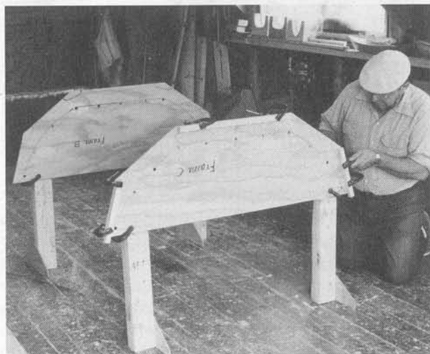
Clamping the frames to the legs.
