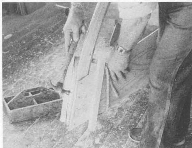
Fitting the side panels to the stem.
