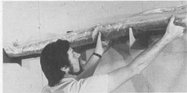
The vacuum bag likes to rest on its own custom wall rack, to minimize damage from handling. Gathers and wrinkles in the bag remain filled with Dum-Dum.
