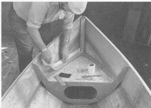
Install the bow seat, coating, puttying, and taping the seams.
