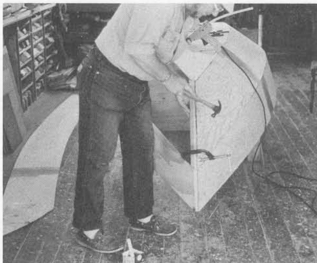
Nailing the bilge panel to the stem.
