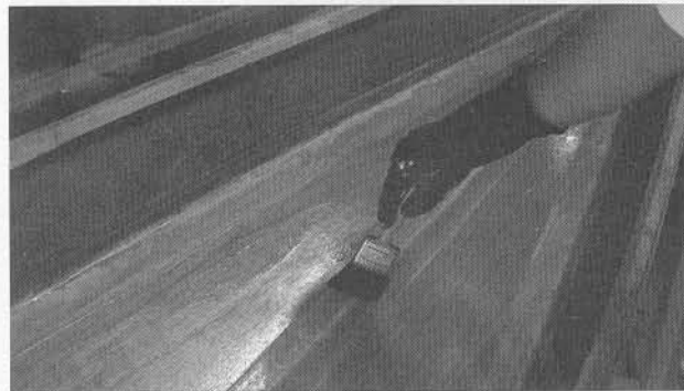
Fully saturate the tape with unthickened epoxy. Work it into the tape with a disposable brush to eliminate dry spots and air pockets.
