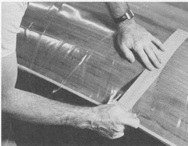
Tailoring the 4-mil polyethylene "parting film" to fit the mold. It keeps the panel from sticking to the mold, and covers the Dum-Dum until it is needed. The fabled "vacuum bag" is just another sheet of polyethylene — but not tailored.
