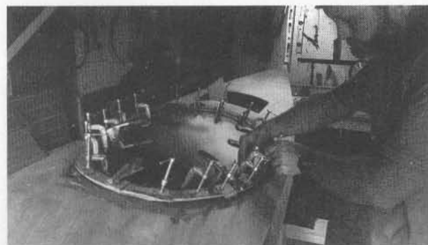
Protect the deck with masking tape when you glue on the cockpit spacer and rim.
