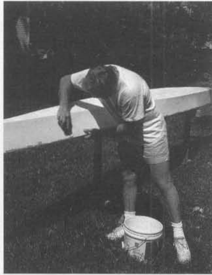
Two-part polyurethane paint leaves a hard, shiny surface. Wet-sand between coats.
