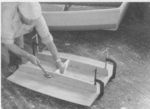
The floor platform can be built in three pieces, as shown in the drawings, or in one piece, if you have a piece of plywood large enough.
