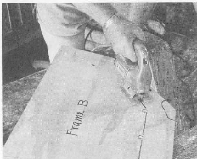
The inside of the frames is partially cut before the hull is assembled.
