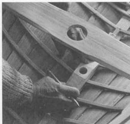
Fitting the mast step.
