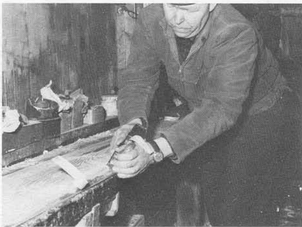
The roughed-out bevel is finished with a hand plane
