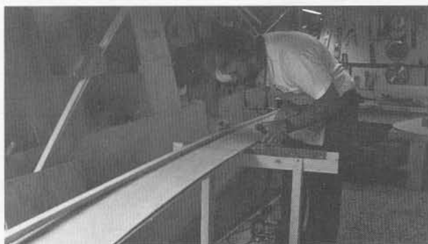
You can glue on both sheer clamps at once by laying the side planks back-to-back.
