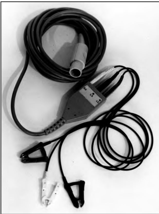
Figure 1.7: The maternal ECG cable detects the maternal ECG and transmits it to fetal monitor for analysis. The MHR will be printed on tracing. (Photographed by Barbara Gibson, Gibson Graphics, Albuquerque, NM)
