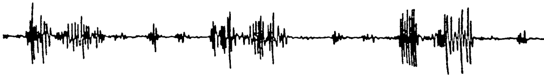
Figure 1.15: Illustration of raw ultrasound waveform received in fetal monitor prior to filtering (modified from Lewinsky, R. M., et al. (September/November 1992). Prediction of pregnancy outcome by combined analysis of the fetal electrocardiogram and systolic time intervals. American Journal of Perinatology , 9(5/6), 349).
