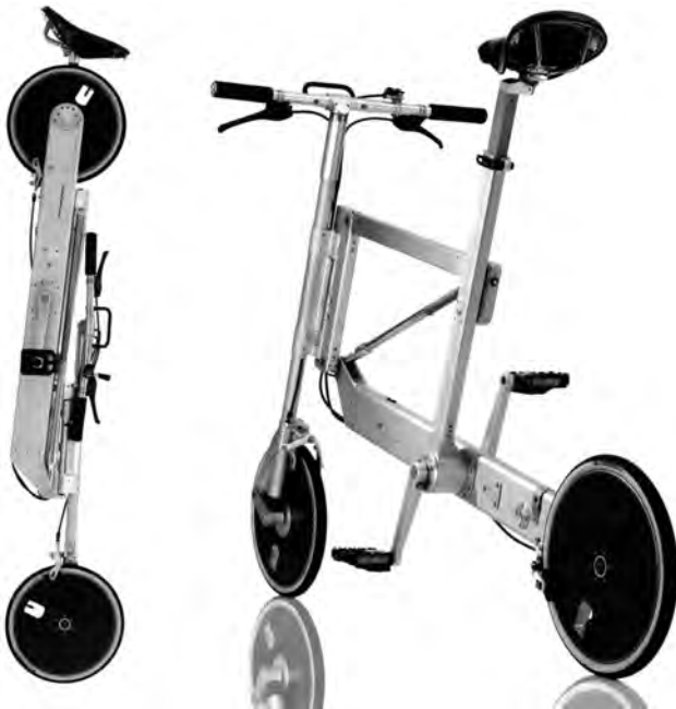
Figure 15.7 Shoji Iwai's design for a folding bike, which won second prize in a 1974 International Cycle Design Competition in Japan ( International Cycle Design Competition: Report on Prize-Winning Projects , Koichi Ishida, 1974).
