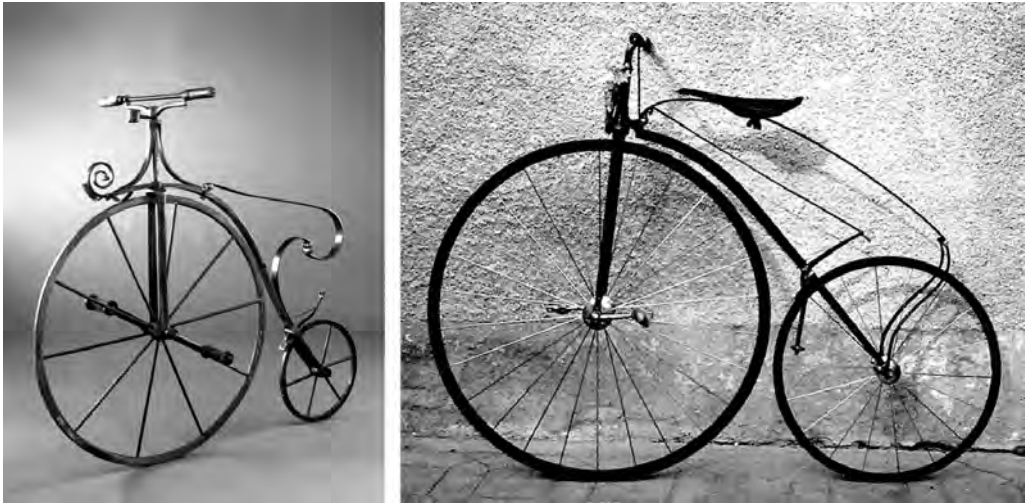
Figure 3.5 Left: Rives's bicycle, with wooden wheels circa 1869 (Robert Sterba). Right: Meyer's all-steel bicycle, circa 1869 (Keizo Kobayashi).
