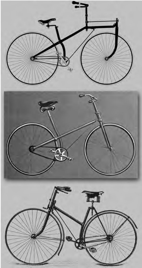
Figure 5.9 Above: An 1887 cross-frame Rudge with bridle-rod steering (Alan Osbahr). Middle: A cross-frame Ivel (R. John Way). Below: An 1889 Universal Rover (catalog picture).
