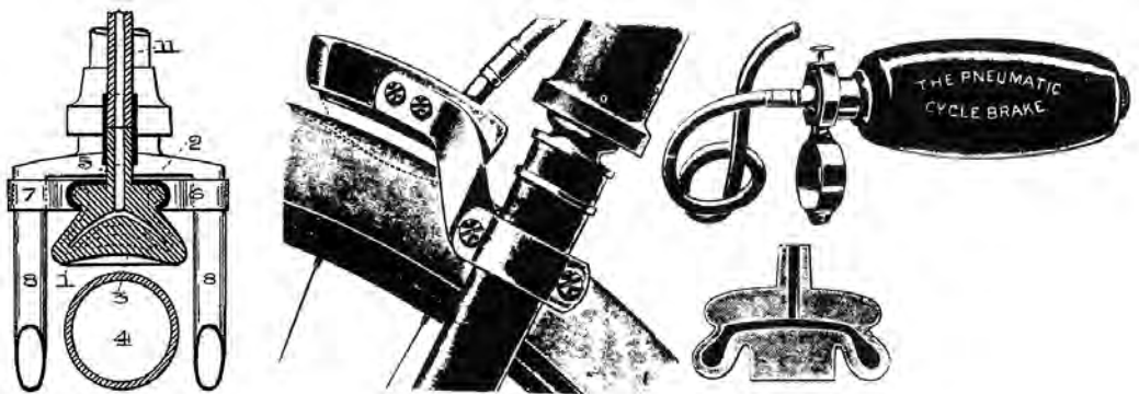
Figure 8.6 Left: A vertical section through the inflatable brake pad of Kitchen's pneumatic brake (patent drawing). Right: A contemporary advertisement for the Pneumatic Cycle Brake showing the inflatable brake pad and the squeeze bulb.
