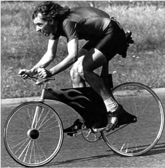
Figure 12.11 Mike Burrows on his 1986 carbon-fiber Windcheetah monocoque (Hugh Swire).
