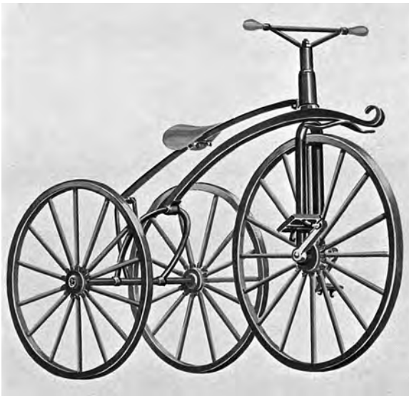
Figure 6.10 An 1818 French velocipede with leaf-spring seat suspension (Deharme 1874).
