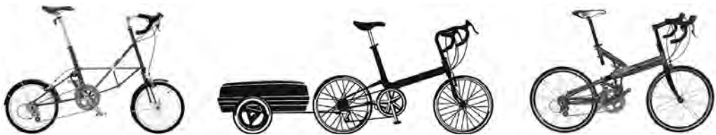
Figure 15.11 Left: A space-frame Moulton (Alex Moulton). Center: An H-frame Bike Friday, with a trailer doubling as a transit case for the folded bike (Bike Friday). Right: An Airnimal (Airnimal).
