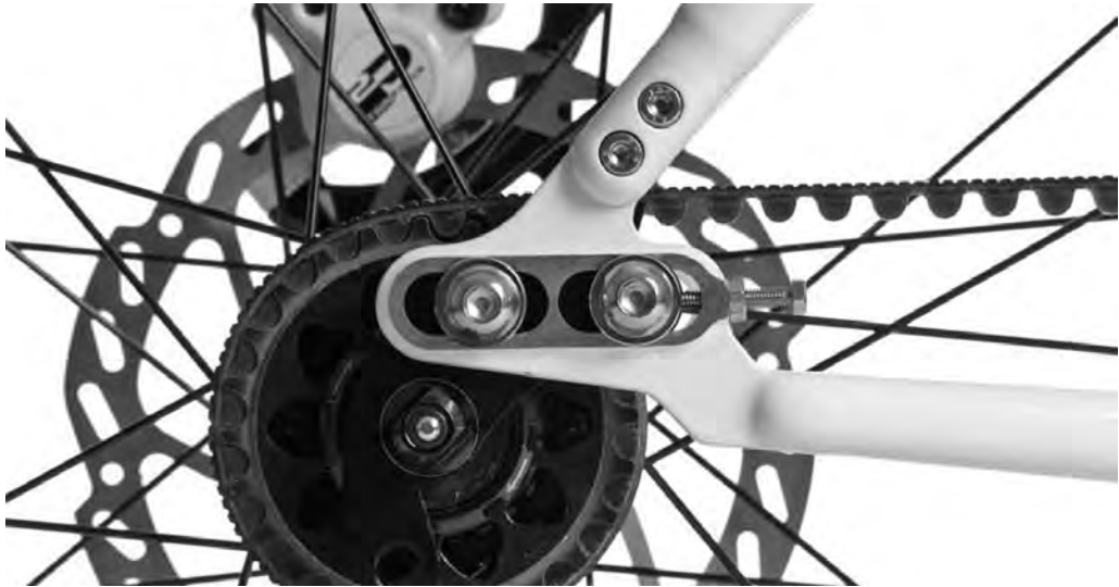
Figure 4.3 A Gates Carbon Drive system. Note the provision for separating the seat stay from the wheel dropout for replacement of the belt (Gates Corporation, photo by Robert Gebler).
