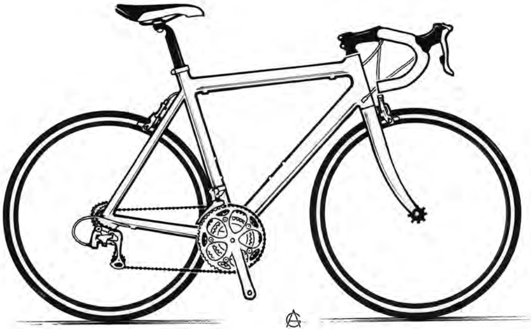
Figure 12.10 A typical aluminum-framed racing bike of the early 2000s (Geoff Apps).
