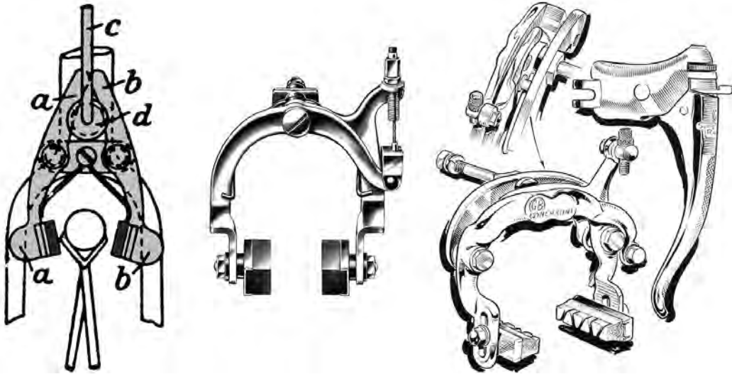
Figure 8.12 Left: Browett and Harrison's 1876 dual-pivot caliper (patent drawing). Center: A Webb steel caliper of the 1930s (National Cycle Library). Right: A GB Synchron dual-pivot caliper of the 1960s (R. John Way).
