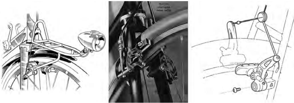
Figure 8.16 Left: Mafac Criterium cantilevers, here used as mounting points for a front rack (R. John Way). Center: A 1934 catalog illustration of the Resilion cantilever brake (National Cycle Library). Right: A cantilever brake of the sort used on mountain bikes in the 1980s (Geoff Apps).
