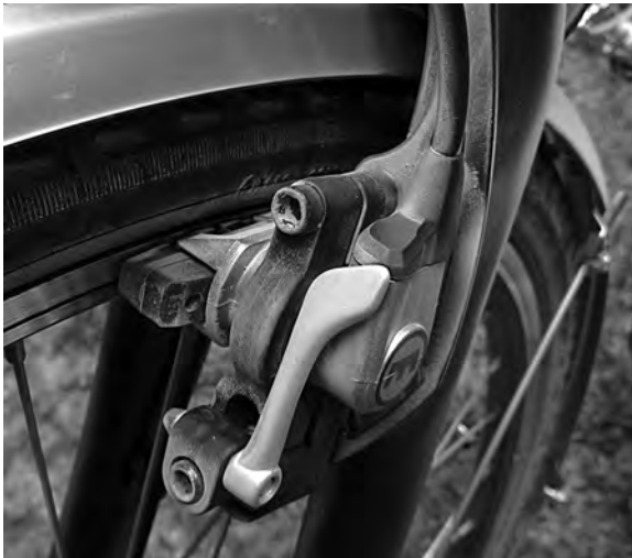
..... Figure 8.18 A well-used Magura hydraulic rim brake (Christoph Eckert).
