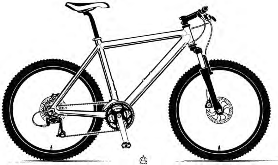
Figure 14.6 A typical mountain bike of the early 2000s with a telescopic front fork (Geoff Apps).
