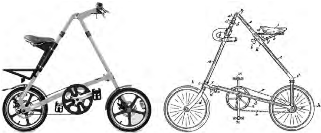
Figure 15.9 Left: A 2011 Strida (catalog photo). Right: A remarkably similar design by Otto Spiess of Berlin (German patent 110,963 of 1897).
