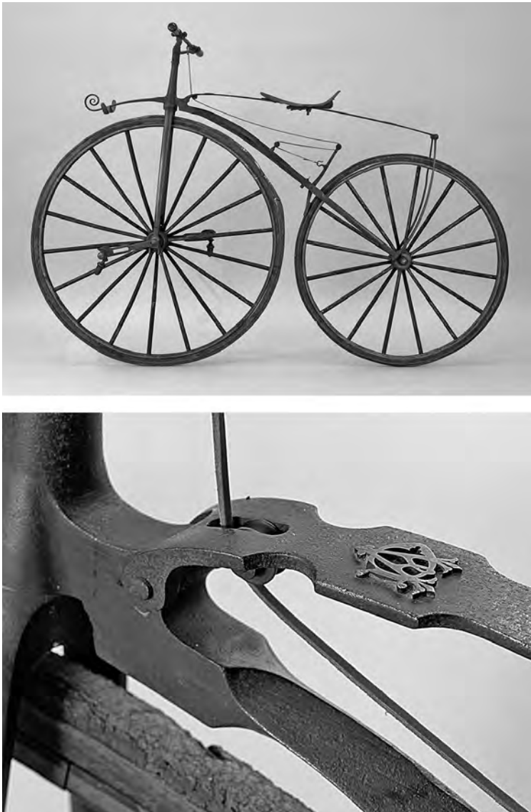
Figure 6.1 Above: A rubber-tired Michaux velocipede of 1868 or 1869 (Jean-Pierre Pradères). Below: A close-up showing a tire, a leather brake cord, and the owner's monogram (Musée d'Art et d'Industrie, Saint-Etienne).
