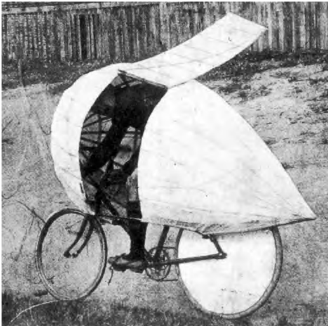
Figure 12.17 The Vélo Torpille with a disc rear wheel (Arnfried Schmitz).
