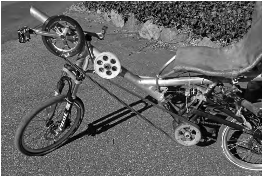
Figure 4.4 Wilson's recumbent, with Browning belt and conventional chain drive (David Gordon Wilson).
