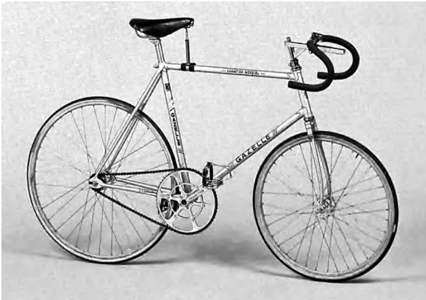
Figure 12.6 A Gazelle stayer bike, circa 1980, with saddle brace and adjustable handlebar reach (Raleigh).
