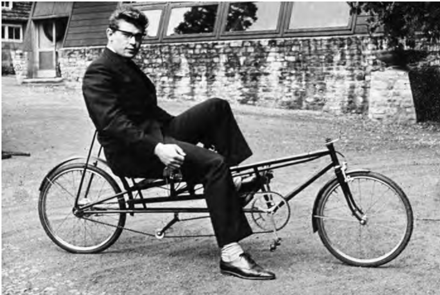
Figure 16.7 A Grubb recumbent of the 1930s being ridden by Brian Cottrell during Alex Moulton’s research into riding positions, circa 1960 (Alex Moulton).
