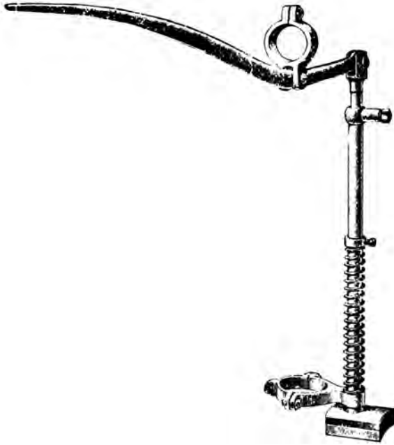
Figure 8.7 A simple plunger brake, circa 1900, with direct rod linkage and a rubber “shoe” acting on the top of the tire (Noguchisan 1998).
