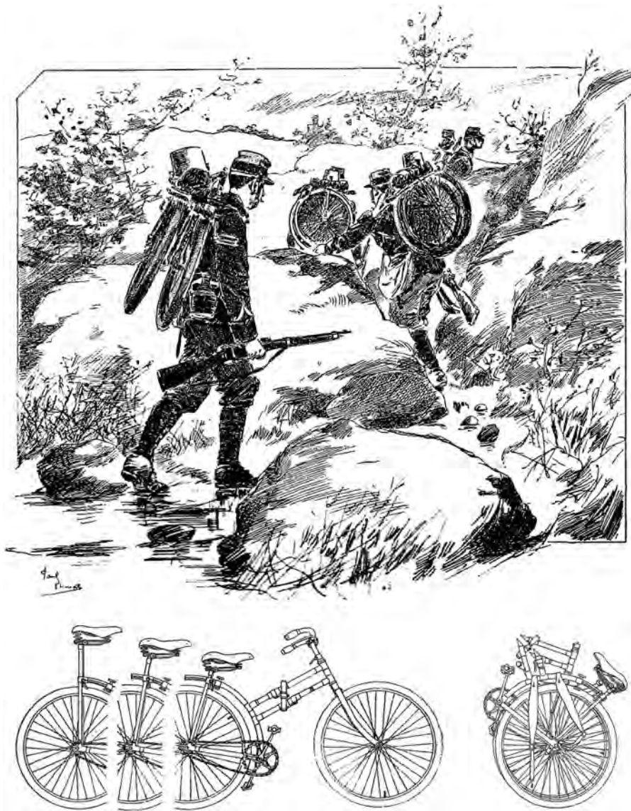
Figure 13.8 Depictions of French soldiers carrying folding Capitaine Gérard bicycles, of the variable geometry of the Capitaine Gérard, and of a folded Capitaine Gérard with shoulder straps (National Cycle Library).
