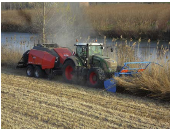
Figure 4.9 Harvest yard formed by a mulcher (Nobili S.r.l.) and baler (Kuhn S.A.). © http://www.nobili.com .
