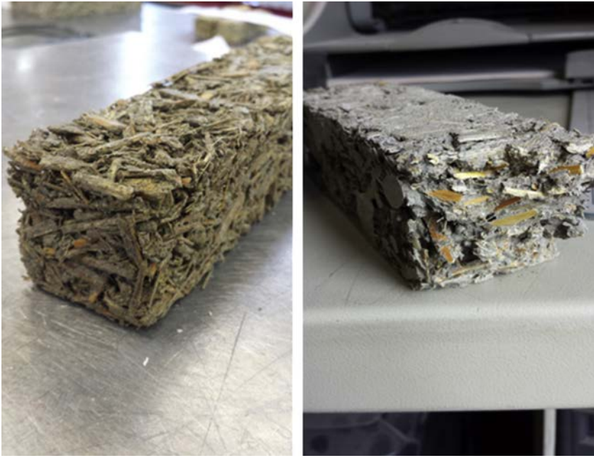
Figure 2.6 Lightweight concrete based on miscanthus biomass. Photo: Danièle Waldmann, Universität Luxemburg.
