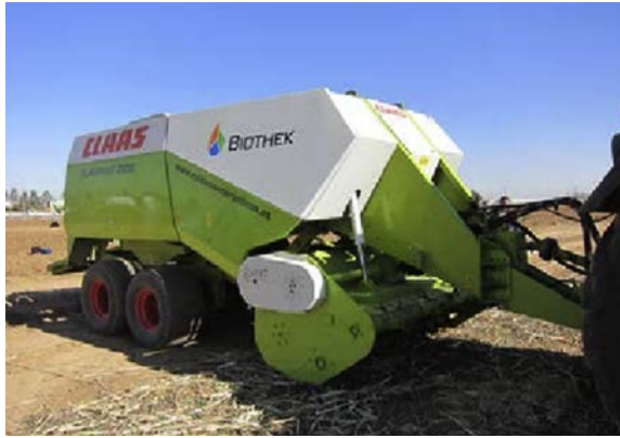
Figure 4.12 Modified Class Quadrant 2100 baler used to collect Arundo. © UPS.
