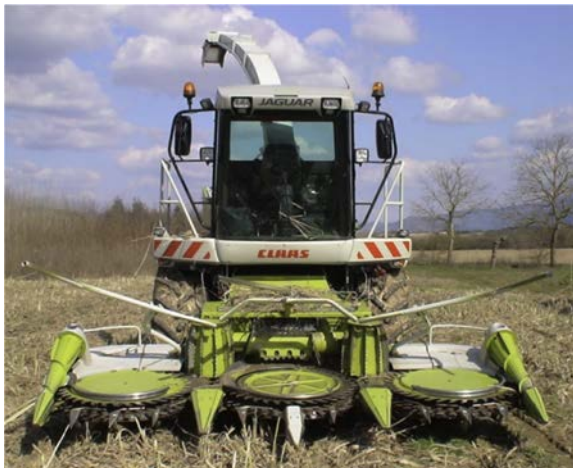
Figure 4.7 Front view of the Claas Jaguar 850 equipped the OrbisRU 450XTRA. © CREA-IT.
