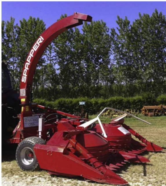
Figure 4.8 Spapperi Ltd. prototype of Arundo harvesting system.
