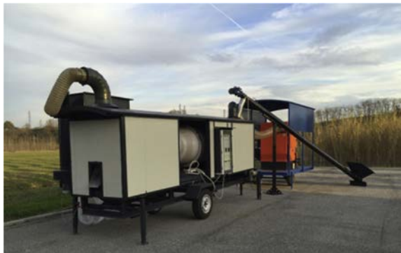
Figure 4.15 Mobile experimental drier tested at CREA-IT powered by a pellet boiler. © http://www.essiccatoremobile.it .
