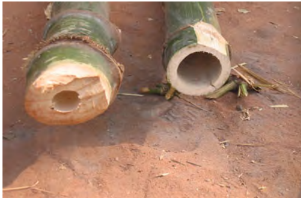
Figure 2- Dendrocalamus strictus - upper and lower section of the same culm. Notice variance in wall thickness
