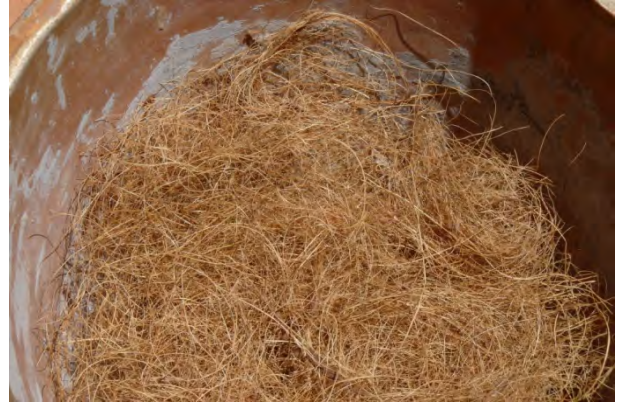
Figure 8 - Coconut fibre density – Fibres are firmly hand compacted and left to rise to level.
