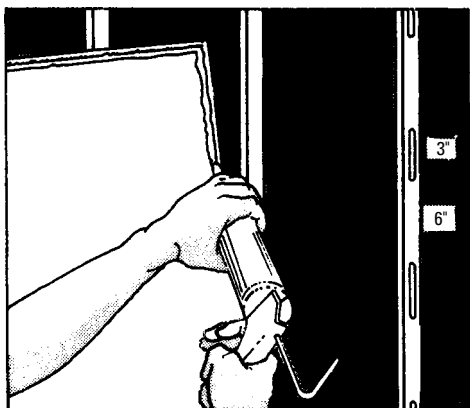
Figure 18-61 Apply adhesive as shown.
