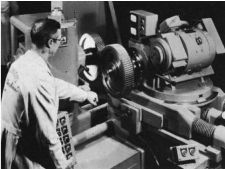
Figure 4-22 Power inspection of helical gears with shafts parallel on a Gleason Universal Tester. (Courtesy Illinois Gear)
