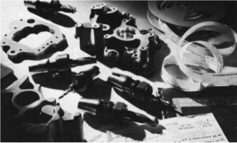
Figure 18-1 Programming and preparing tape is simple and time saving. It involves deciding on the number of workpieces per load and their location on the subplate, preparing the tool and program sheets from the piece part drawing with coordinate dimensions, and punching tape using conventional tape preparation equipment.
