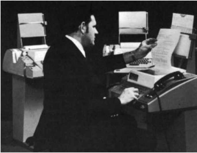
Figure 16-4 Tape containing the setup instructions and operation program is transmitted by dataphone terminal. (Courtesy Sheldon Machine Co.)
