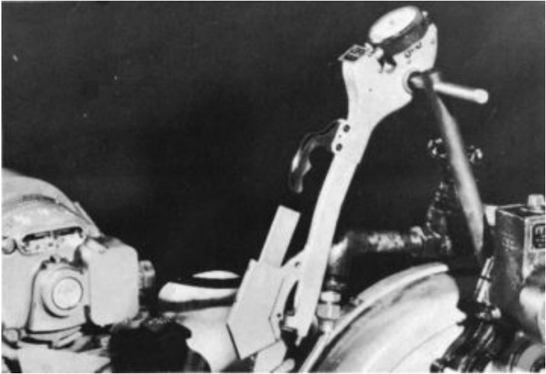
Figure 7-8 Grinding gage retracted for replacing workpiece. (Courtesy Federal Products Corp.)
