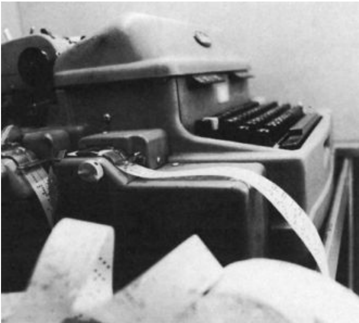
Figure 18-4 Conventional tape preparation unit. This unit is usually located away from the machining area. (Courtesy Moog Hydro-Point)
