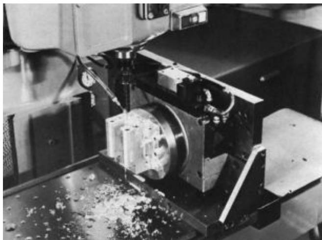
Figure 18-12 Peck drilling. A pecking action is used to facilitate deep hole drilling. The cutting time between pecks is preset on a timer, eliminating the necessity to program each peck depth. At each peck, the tool is withdrawn (at 300 ipm) to clear the chips and returns (at 300 ipm) to 0.015 inch above the previous cut. This ensures maximum tool life and gives accurate deep holes, as small as 0.014 inch in diameter, without tool breakage. (Courtesy Moog Hydro-Point)
