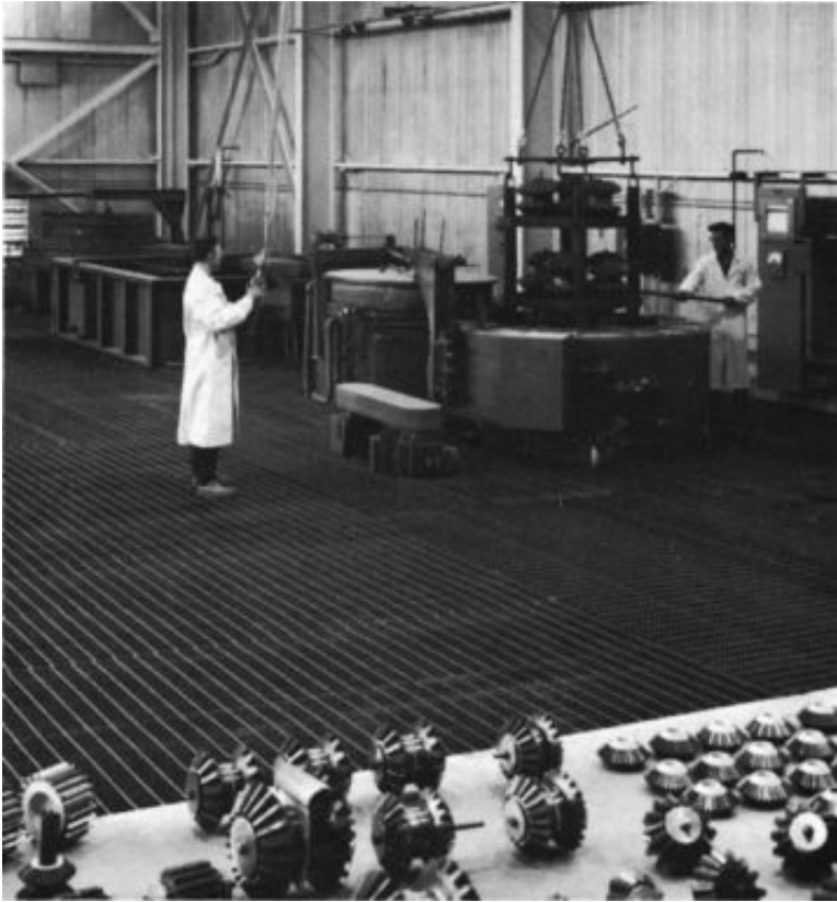
Figure 10-5 Deep pit furnace being loaded with bevel gears.
