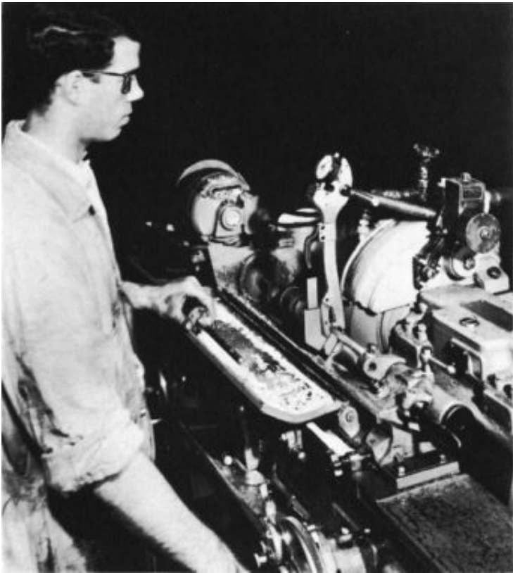
Figure 7-7 Grinding gage measuring work during grinding.
