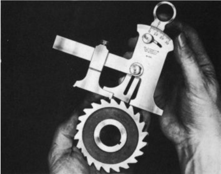
Figure 7-30 Checking milling cutter clearance angle. (Courtesy L. S. Starrett Co.)
