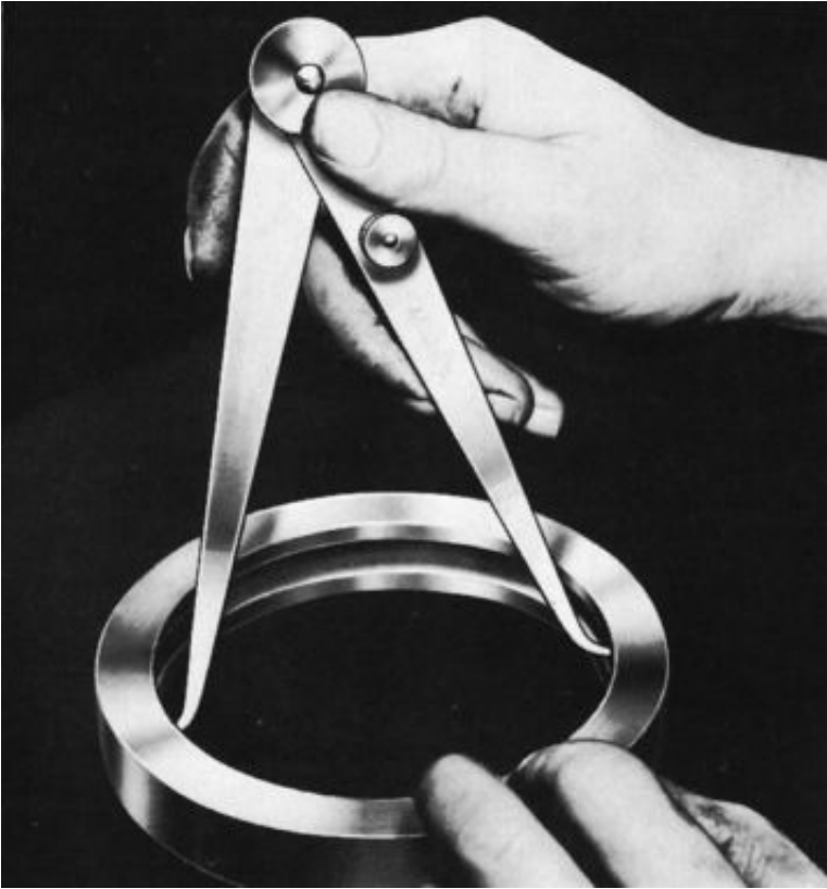
Figure 9-2 The proper way to hold an inside caliper. (Courtesy L.S. Starrett Co.)
