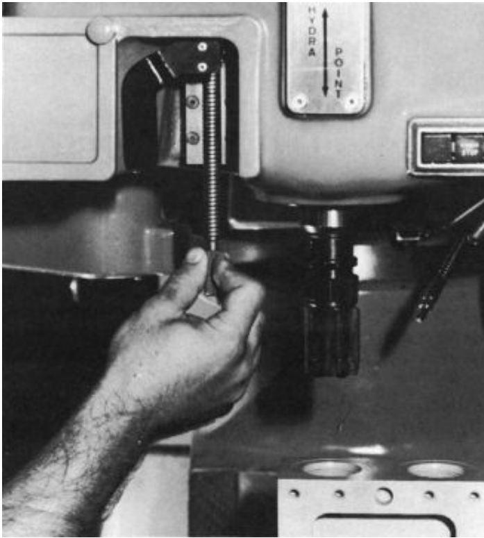
Figure 18-19 The lead-screw tapping operation will produce class 3 threads with very accurate depth control. A precision-ground lead screw is hydraulically traced, and it controls the feed rate of the tap in relation to the pitch and spindle speed. The only load applied to the tap is the torque required for cutting. (Courtesy Moog Hydro-Point)
