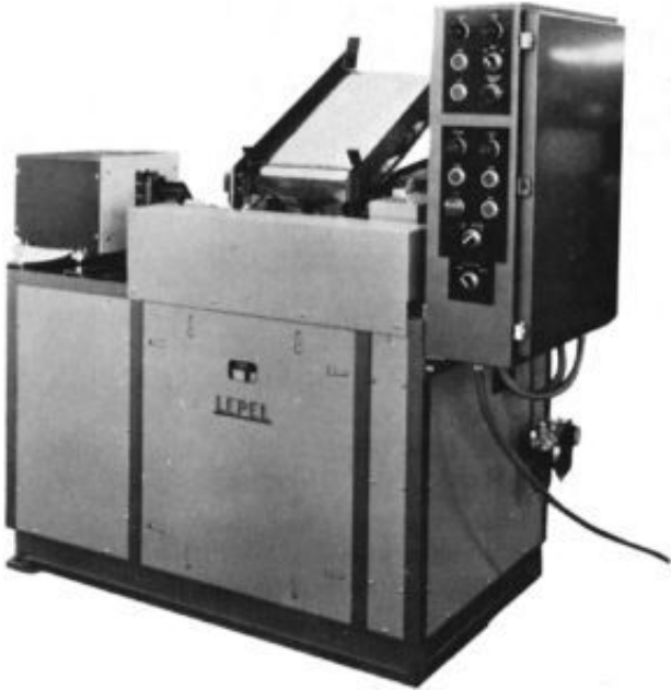
Figure 12-7 An automatic rod-heating device, using radio-frequency induction heating. (Courtesy Lepel Corporation)
