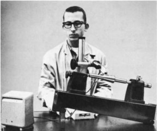
Figure 9-35 Sine bar with head and tailstock. (Courtesy DoAll Co.)
