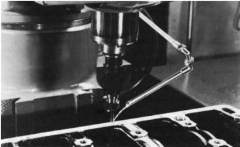
Figure 18-17 Coordinated tapping provides a fast tapping cycle, where spindle speeds and feeds are coordinated under tape control, to match the pitch of the thread. A compensating tension/compression tap holder is used for the operation. (Courtesy Moog Hydro-Point)
