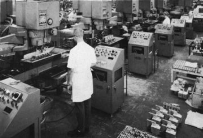
Figure 18-2 A row of numerically controlled machining centers with 24-station random-selection automatic tool changers. (Courtesy Moog Hydro-Point)
