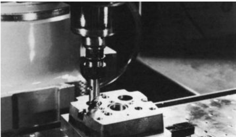
Figure 18-14 Boring. A super-precision quill fit coupled with guaranteed spindle runout less than 0.0002 in TIR and positive tool orientation ensures close-tolerance bored holes. Hole size and geometry can be held within 0.0002 inch under production conditions. This “canned cycle” allows tool withdrawal at programmed feed rate, thus eliminating taper and tool marks. (Courtesy Moog Hydro-Point)
