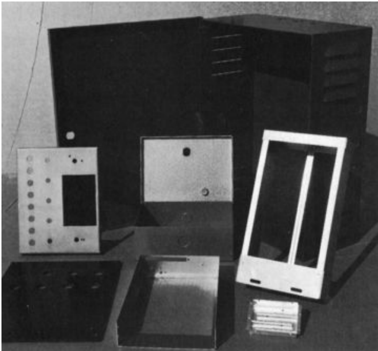
Figure 6-5 Parts that require shaping. (Courtesy Paul and Beekman, Inc.)
