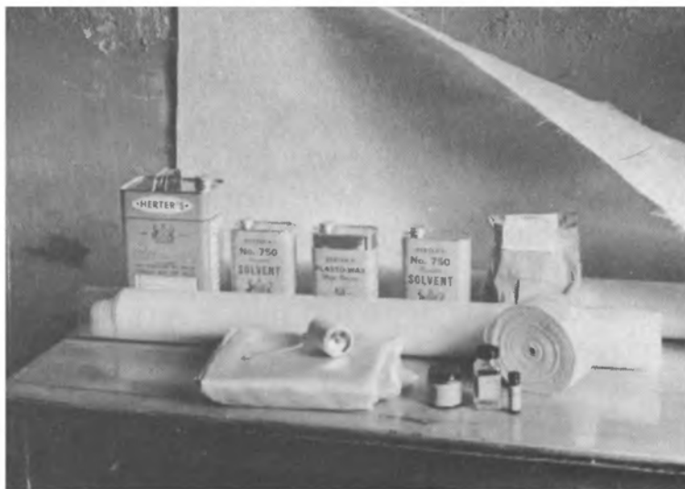
Raw materials for making a fiberglass tube. The transparent material at left is the vinyl plastic used to line the tube.
