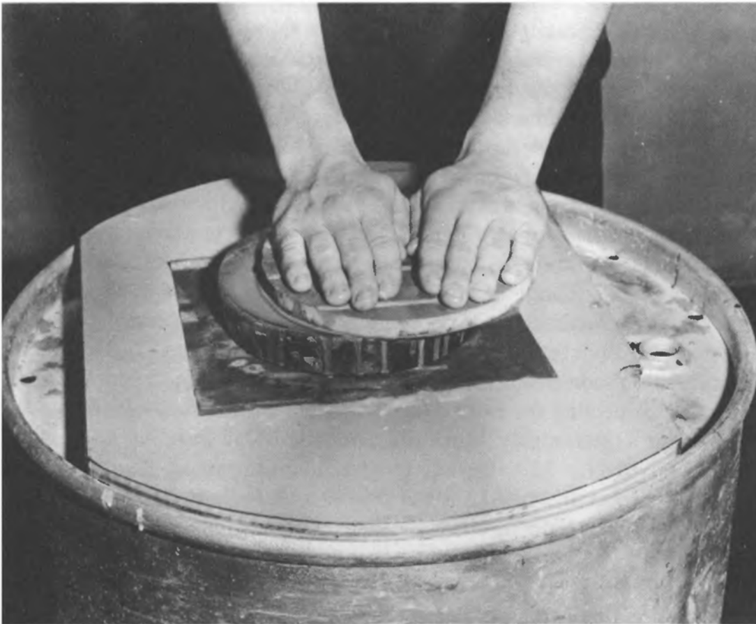
Grinding with the tool on top to lengthen radius of curvature. The serrations are typical of this kind of ceramic tool.
