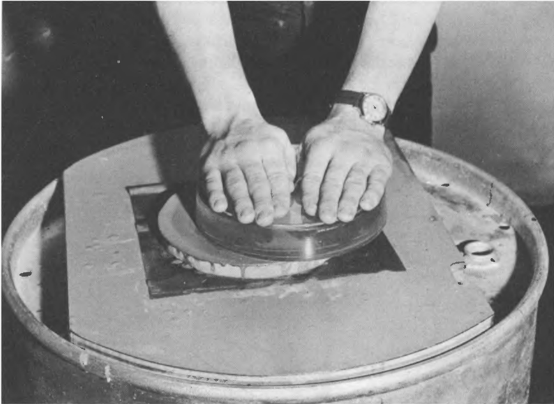
Wet paper toweling holds the mirror in place as effectively as cleats during grinding operations. Note the position of the hands on the mirror.
