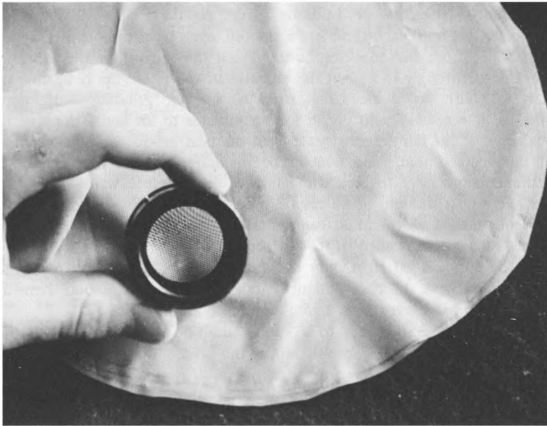
Plastic material useful for fast polishing. Note the projections seen through the eyepiece. Each one increases the polishing action.
