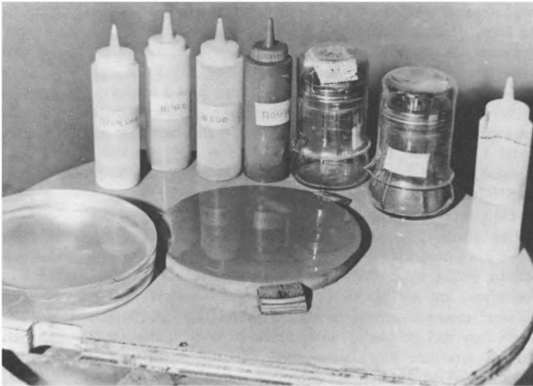
Raw materials. The tool ( center ) used for this 8-inch mirror is a ceramic material similar to pipe tile.
