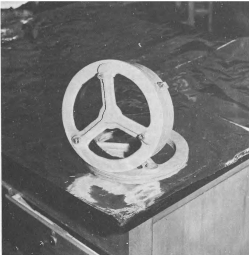
A fiberglass cell (unfinished in this picture) and the pattern from which it was made.
