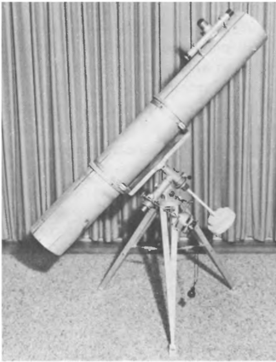
Portable mounting for an 8-inch reflector, made by John Mierzwa, of Auburn, New York. This mounting is very strong but so light that it can be carried by Mr. Mierzwa's eight-year-old daughter. The drive has a friction clutch so that the telescope may be adjusted even while the drive is running. (Tarby Photo, Auburn, N. Y.)
