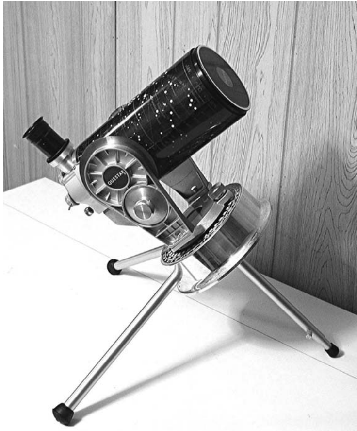
Figure 3.2. A fork-type equatorial mount.
