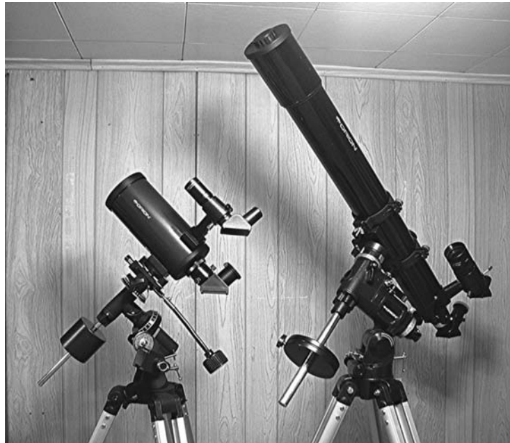
Figure 3.1. A comparison of German-type equatorial mounts.
