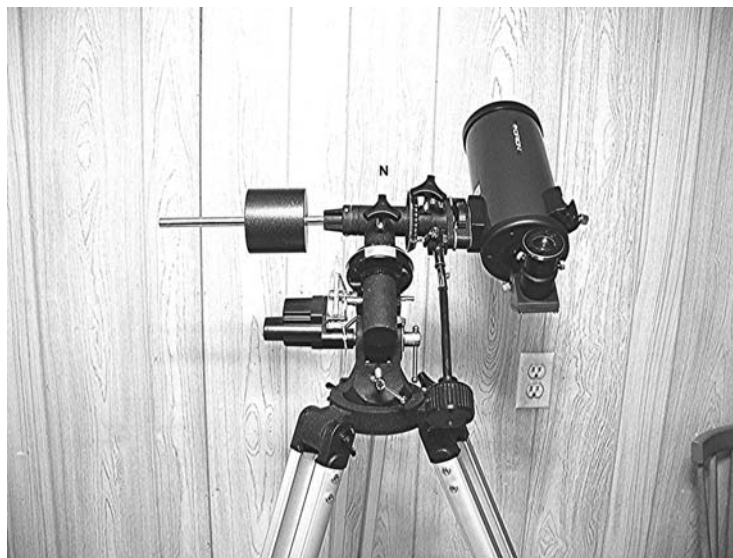
Figure 3.9. Adjusting the polar axis in azimuth.
