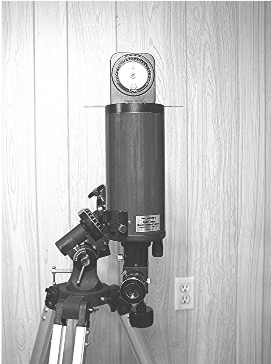
Figure 3.11. Calibrating the declination circle on a GEM mount.
