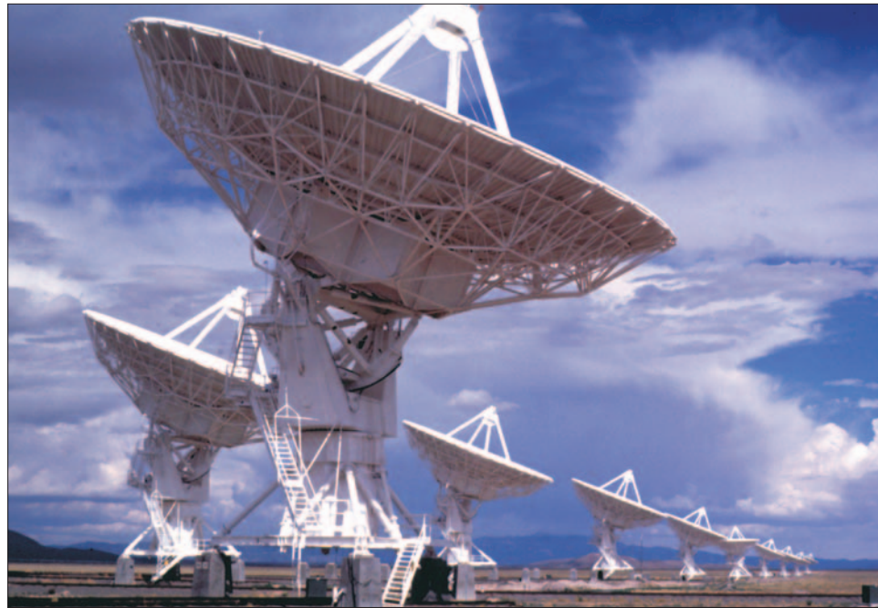
▲ The Very Large Array, in New Mexico, is one of the world's premier radio observatories. Its 27 antennae can be arranged into four different Y-shaped configurations. Each antenna is 25 m (82 feet) in diameter, but when the signals are combined electronically it functions as one giant dish, with the resolution of an antenna 36 km (22 miles) across.
