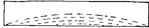
Fig. 25. How the curve is obtained by use of the conventional method of grinding the mirror.
