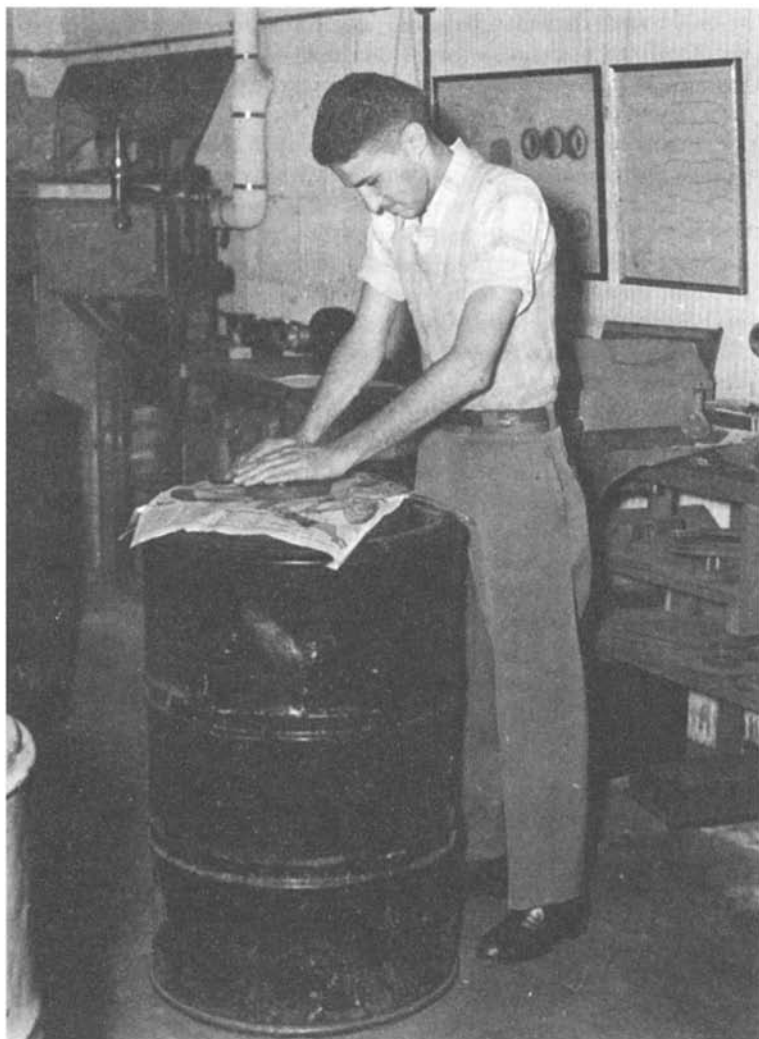
Plate III. Here is illustrated the proper position of the hands and arms, and of the body, while grinding. Pressure is the keynote for this operation.
