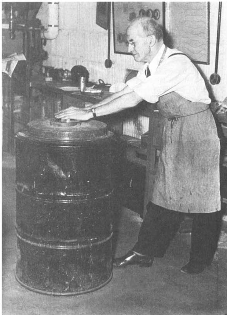
Plate IV. Polishing the mirror is a delicate operation. Note the position of the arms, and the stance, different from those used in the grinding operation in Plate III.
