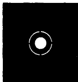
Fig. 86. Appearance of a perfect star image in a reflector. (Linear diameter of the bright ring at the focus of an f/8 telescope is 0.00057'' .)
