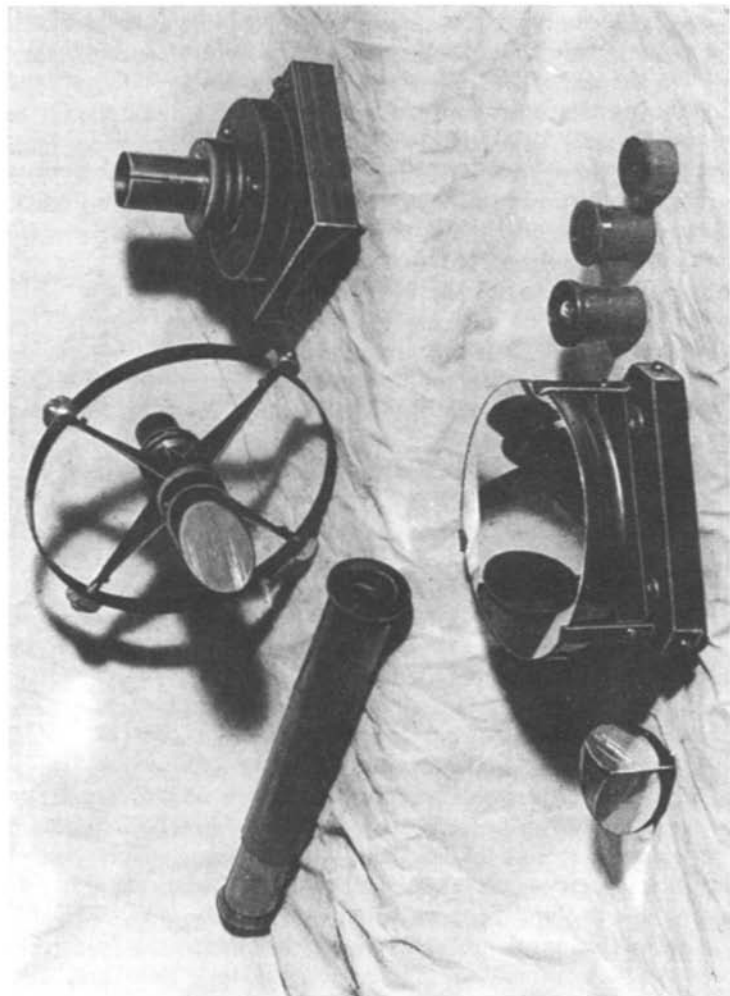
Plate V. Optical parts of a Newtonian: finder, diagonal mirror, spider support, eyepiece adapter tube and holder, prism (alternate for the diagonal), primary mirror in cell, eyepieces.
