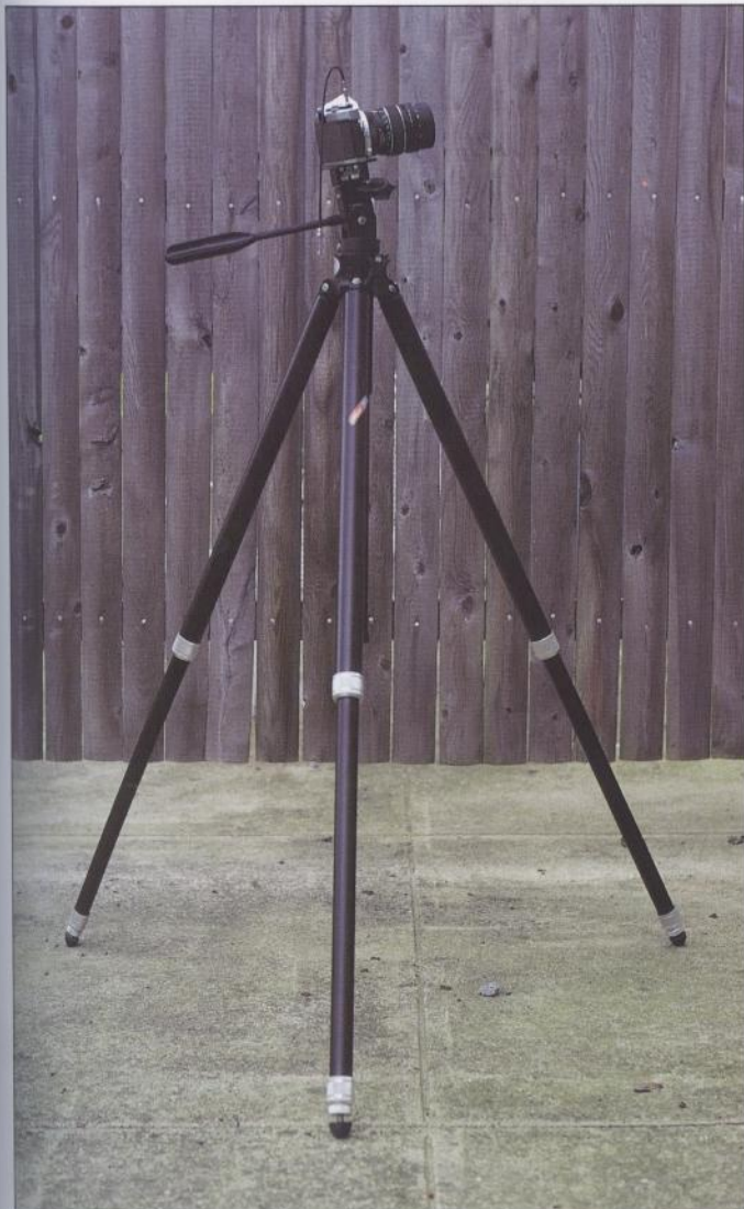
A 35 mm SLR camera mounted on a sturdy tripod for astrophotography (e.g. star trails, auroras, constellations, bright comets, etc.)
