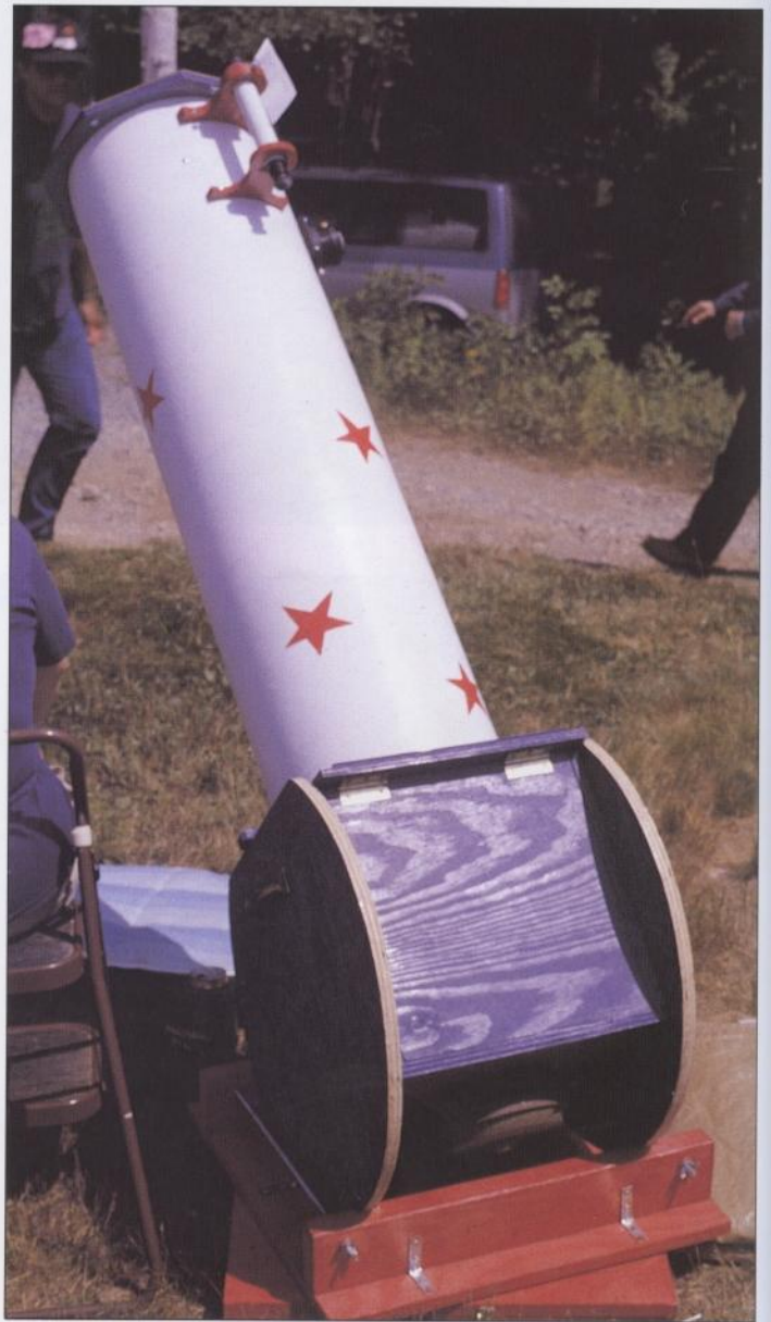
A simple variation on the Dobsonian reflector design. Note the low-to-the-ground rocker box, designed for compactness and stability, and the use of plywood in the rocker box.
