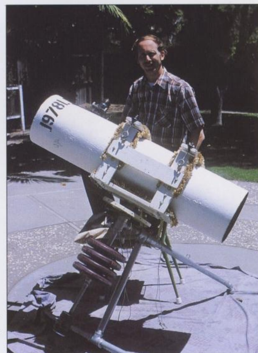
Photo by David Deremo showing his 22-inch f/5 telescope with an observer's work table. This table has a red back-lighted top surface for reading star maps and has drawers for eyepieces and accessories.
