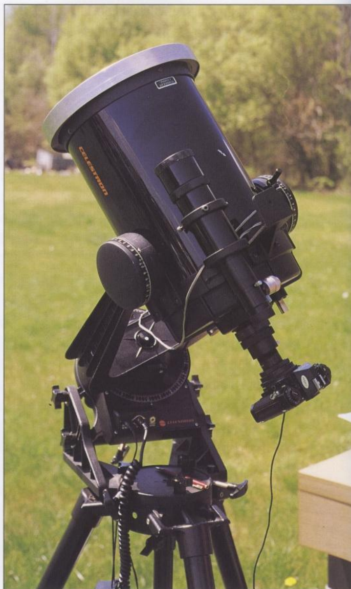
A Celestron 8-inch Schmidt-Cassegrain telescope set up for solar photography. A 35mm camera is attached to the focus at the rear with a T-mount and adapter. A full aperture solar filter covers the front end of the telescope.
