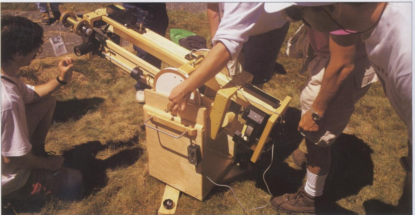
A 5-inch Dobsonian reflector exhibited at the 1994 Stellafane Convention by Jerry Wolczanski of Warrenton, Virginia. Note the wooden framework and open tube.
