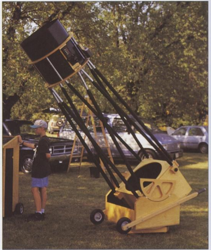
Close-up of David Deremo's telescope mirror box and altitude bearings. The two wooden wheelbarrow-like handles allows this telescope to be moved easily by one person.
