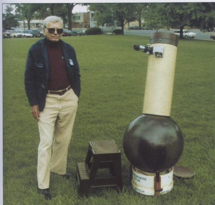
Henry Stockmar of Richmond, Virginia with his 8-inch f/6 Newtonian reflector and its unusual plastic sphere alt-azimuth mount, which glides on three nylon furniture glides.
