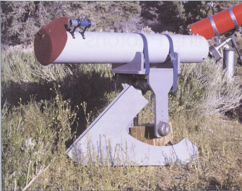
A Newtonian reflector with a simple equatorial mount made of plywood and plumbing pipe.
