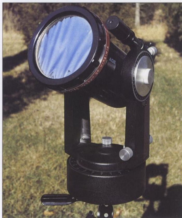
An aluminized Mylar™ solar filter mounted on a small Schmidt-Cassegrain telescope.
