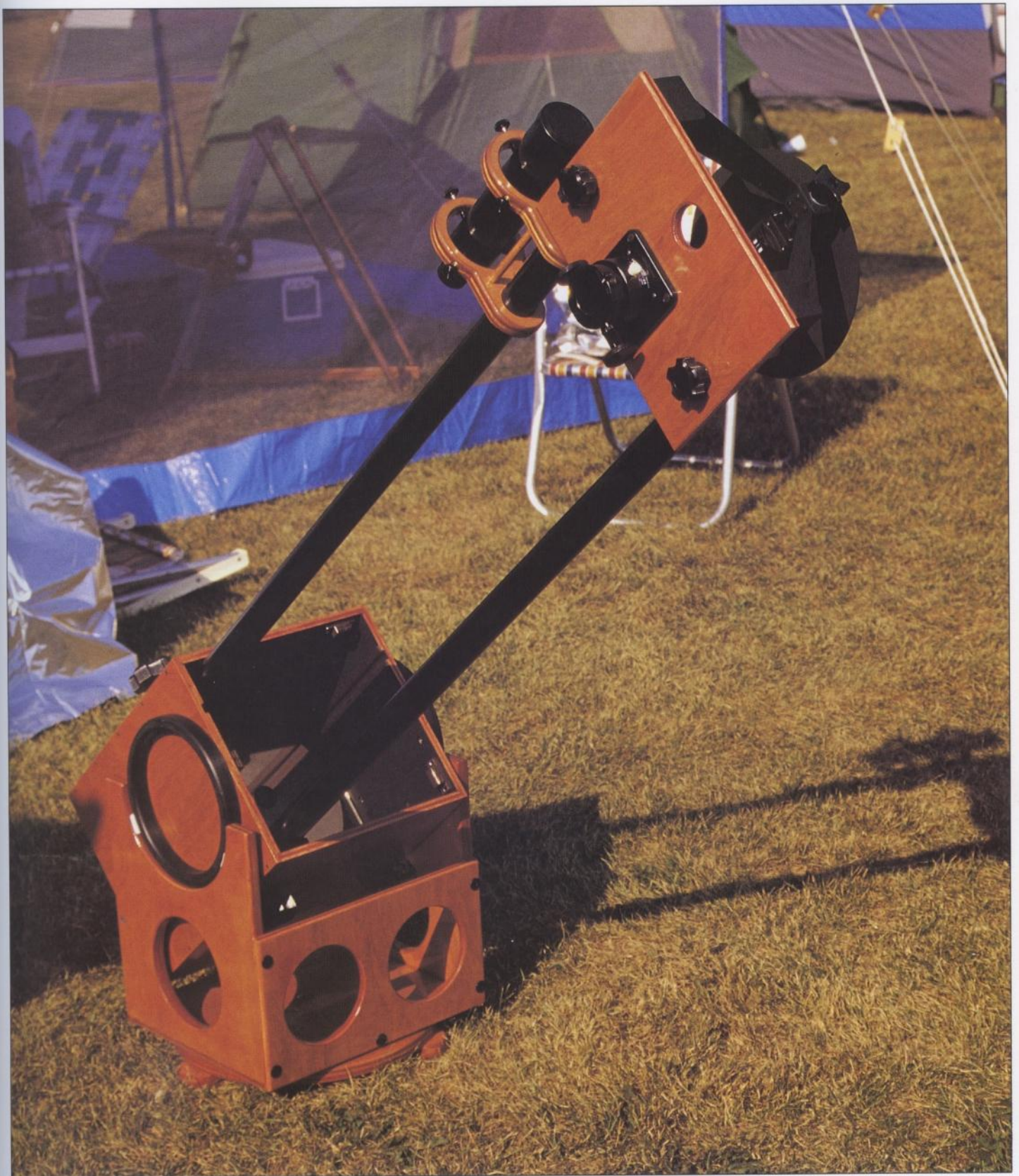
10-inch light weight, tubeless Dobsonian (a variation of Alice in this book) built by Ron Ravneberg.
