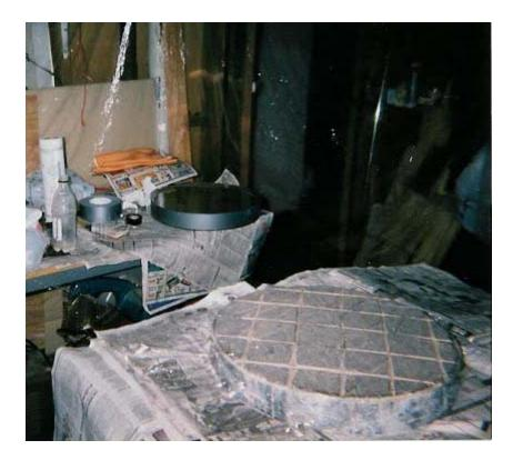
Here is the lap (foreground) and mirror (background). Small crevases and indentations in the sides of the mirror harbored grit particles that no amount of scrubbing could remove. Duct tape was wrapped around the mirror to trap the particles. A "clean room" was created in the garage workshop by lining the ceiling with plastic drop cloth and drapping it from the ceiling and around the work area.
