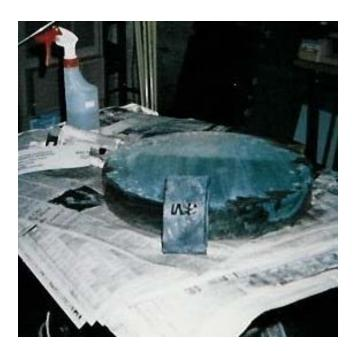
As grinding progressed, the bevel on the edges of the mirror and tool had to be maintained. I used a rubber sanding block (you can see it leaning on the mirror) with silicon carbide sandpaper to do the job. I started with 80 grit and finished with 1500 grit.
