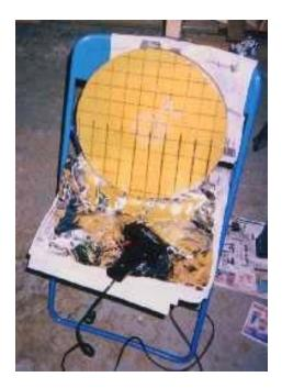
There are many ways to create the channels in the lap. I used a soldering gun and soldering iron to do the job.
