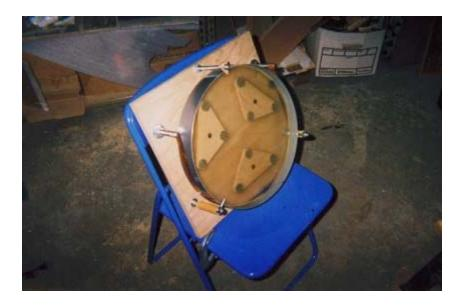
The next photo shows the mount under construction. Duct tape wrapped around the mirror was later removed. The mirror rests in on a 9 point floatation mount. The mount design is very similar to that described in Kriege and Berry's book, **"The Dobsonian Telescope - A practical manual for building large aperture telescopes"**. However, instead of using steel, I used
