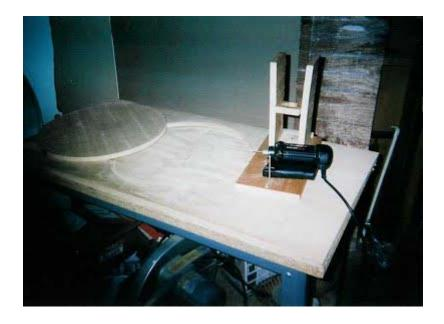
To make the mount and elevation bearings, I used a 2X4 foot sheet of plywood, 3/4 inch thick, and cut a hole 20 inches in diameter in the center with my homemade circle cutter. This disk and a duplicate were cut in half and glued together to make the elevation bearings for the scope.
