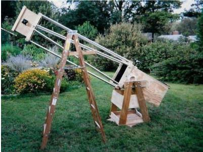
Here's the completed telescope and mount at a local park. With a tube length of 9 1/2 feet, a ladder is required for using this telescope. To help balance the telescope, the view finder was placed on the mirror box, just above the elevation bearing.
