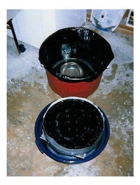
After the pitch was poured and the channels cut, the lap had to be hot pressed.
