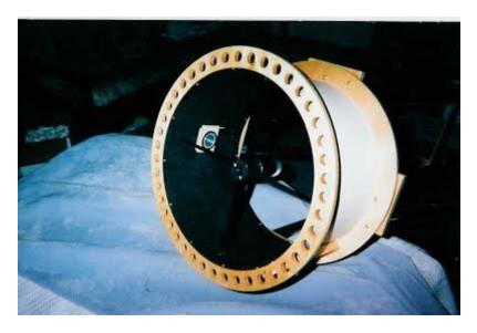
Here's the completed cage attached to the upper part of the truss. I used a rather simple helical focuser from <u>Odyssey</u>, because I wanted something light and this focuser weighs a little more than 100 grams.
