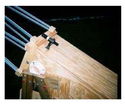
This is a close-up of the elevation bearing. The PVC plastic bearing (Toilet bowl flange - 5 inches wide) rests directly on wood. No teflon pads were necessary. To my surprise the motion turned out to be nice and smooth. However, such a small bearing results in a rather unstable mount, especially in the elevation axis. Experiments with pads (cardboard glued to a sheet of plywood) placed between the mount and the mirror box improved the stability significantly and were installed as shown.
