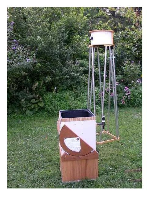
As with my earlier telescope design this one also breaks down into three parts: truss, mirror box and mount. The truss is held to the box with 4 bolts. Set-up and take down is rather easy. It typically takes less than 15 minutes to carry out the parts to the yard and assemble them. Collamination of the optics is usually a minor adjustment. Yet, there is one drawback; I can't easily transport this telescope in a car.
