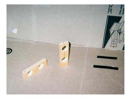
Here are the truss clamps to hold the poles to the cage. They are made of 1 3/4" wide by 3/4" thick pine and each hole was drilled at an angle of 83 degrees to properly accomodate the pole, Next, I cut a slit lengthwise and almost through to the end. A bolt was passed through on the other end to clamp the poles down tightly. Another bolt was passed through the center between the holes to clamp the poles even tighter.
