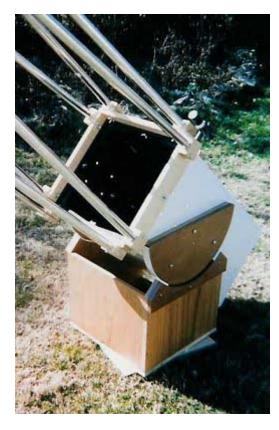
Here is the completed mount. I used the old mirror box and painted it white. If you look closely, you can see the holes for the old bearings. They were filled in later. I also used the same mirror mount as described above.
