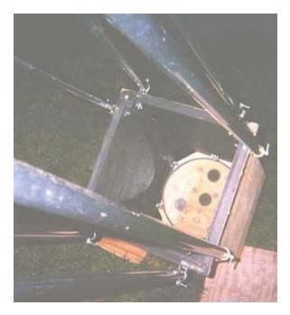
Inexpensive steel pipe clamps were used to fix the aluminum poles to the mirror box and
