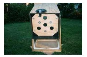
Here's the back of the scope, showing the mirror mount inside the mirror box. The three mirror adjustment knobs shown were made from steel washers affixed to the end of the bolts that
