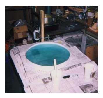
Here's the glass tool ready for liquid pitch to be poured onto it. The lap was leveled as best as possible to ensure an even thickness of pitch. Wax paper folded over many times was wrapped around the tool to trap the pitch. Before the pitch was poured, turpentine was rubbed on the tool with a paper towel so that the pitch would adhere better to the glass.
