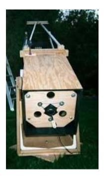
Later, a small electric fan (to cool the mirror) was placed over the central hole and suspended by rubber bands to reduce vibration. Also, by paring down the weight of the secondary cage, I later eliminated the need for the weights clamped to the back of the mirror box. Lastly, note the white shelfing brackets used to strengthen the mount. Smaller ones were used to hold the mirror box together. They are inexpensive and quite strong.
