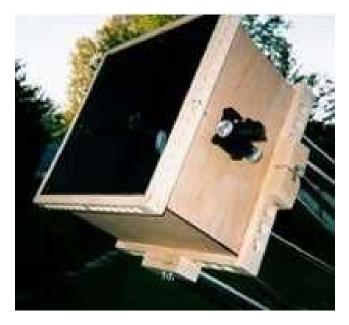
Here's a close-up of the secondary cage. It's simply a wooden box made of 3/16" plywood held togther with 3/4" thick strips of pine. To improve the balance of the telescope, I later drilled large holes in the pine strips, as shown, to lessen the weight of the cage.
