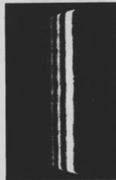
Fig. 34. Shadow fringes seen with knife inside the focus. Spherical mirror with turned-down edge of \frac{1}{3} wave ( 5 \mu slit).
