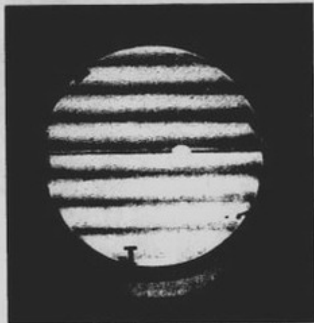
Fig. 51. Interference test on a flat mirror. Note: Reference line near the central fringe is formed by a taut wire or string. White spot is reflection of the neon lamp. The thin shim is marked T. The extreme edge is turned down.
