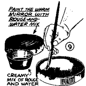
PAINT THE PITCH WITH ROUGE AND WATER. STRIP THE COLLAR AFTER PAINTING
