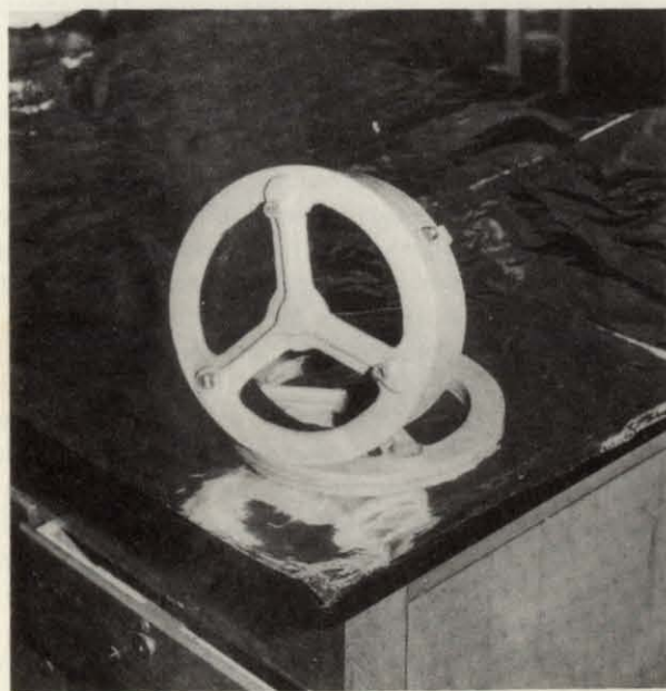
A fiberglass cell (unfinished in this picture) and the pattern from which it was made.
