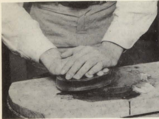
Using the chordal stroke to hollow out the mirror. The mirror shown is a short-focus 6-inch, and the hollow is deep, as you can see from the inclination of the mirror.
