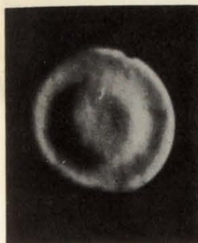
Three stages in the treatment of a 3-inch mirror, starting with an oblate spheroid whose central hill has a hole in its center. Below , mirror has "flattened" to a nearly spherical surface. (Focograms by Samuel Borrello)
