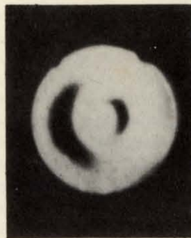
Three stages in the treatment of a 3-inch mirror, starting with an oblate spheroid whose central hill has a hole in its center. Below , mirror has "flattened" to a nearly spherical surface. (Focograms by Samuel Borrello)
