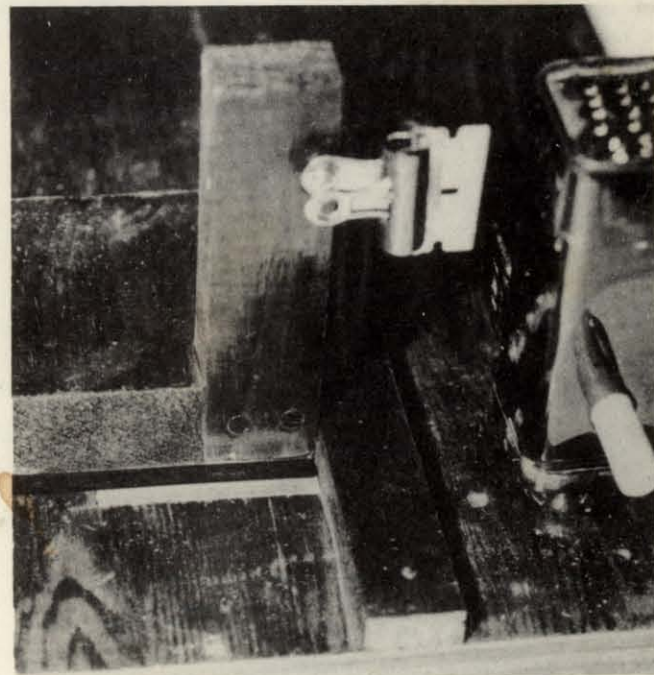
Simple Foucault tester, rear view. The white scale at lower left is part of the Barr scale.
