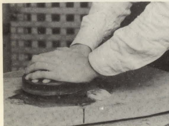
Diametral, or center-over-center, stroke.
