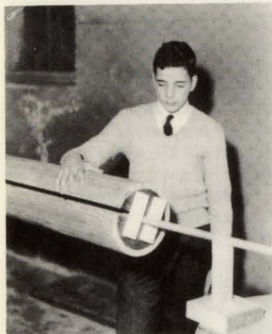
How the mold for the tube is set up. The longitudinal spreaders have not been inserted.
