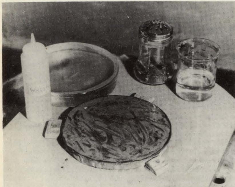
Too much abrasive soon turns into mud, as shown here.
