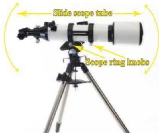
Figure 26: Balancing the scope's declination axis.
