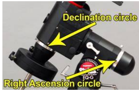
Figure 7 : Setting circles on an EQ mount.
