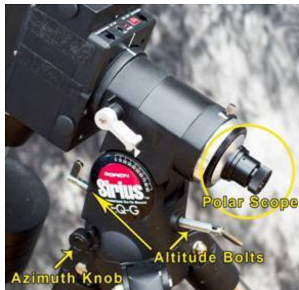
Figure 22: Location of the polar scope on an EQ mount.
