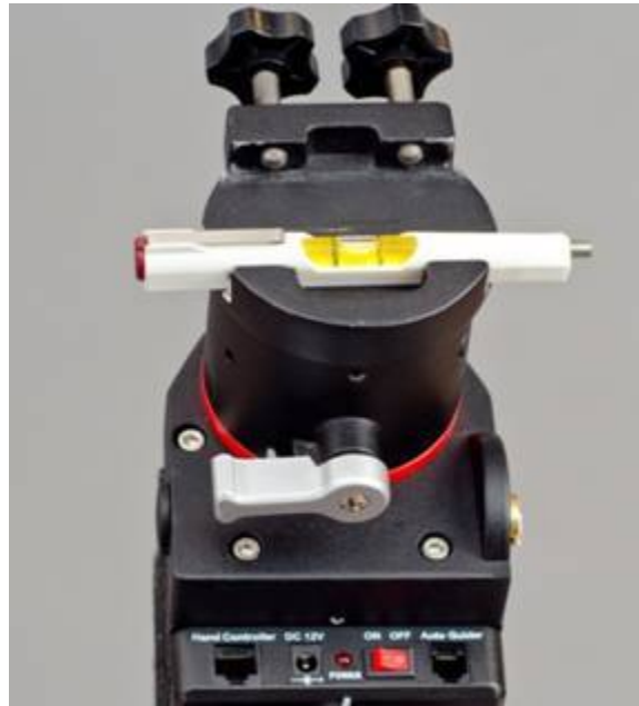
Figure 20: Making sure the declination axis is level.
