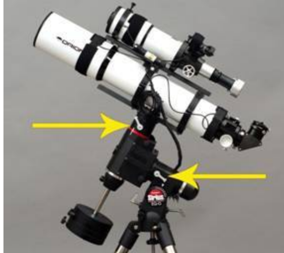
Figure 17: Declination (top left) and right ascension (lower right) clutch levers.
