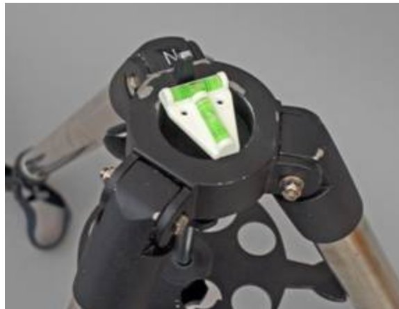
Figure 16: Dual axis level being used to level the tripod.
