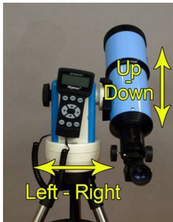
Figure 1: A typical altitude azimuth telescope mount.
