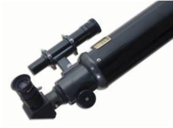
Figure 29: A typical optical finder mounted to a telescope with adjustment screws.
