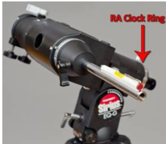
Figure 18: Making sure the counterweight bar is level.
