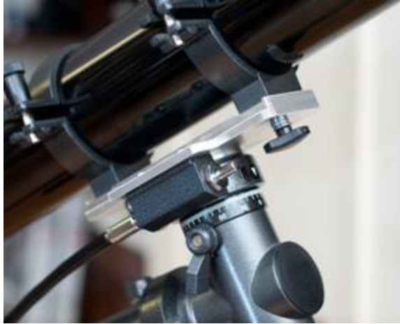
Figure 24: A proprietary telescope mount plate with rings attached.
