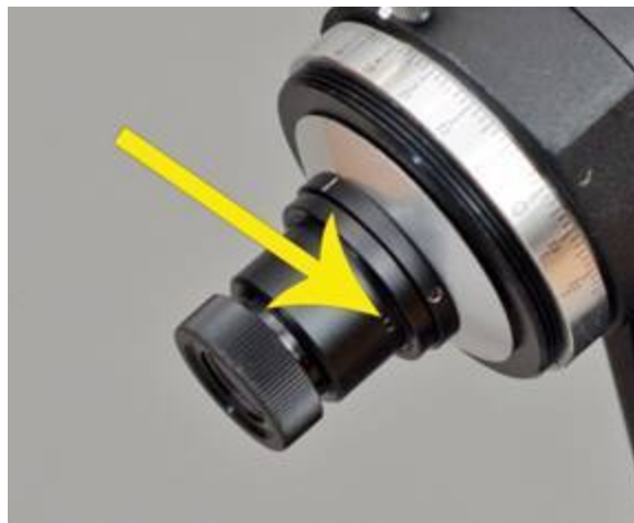
Figure 23: One of the three polar scope adjustment allen head screws.
