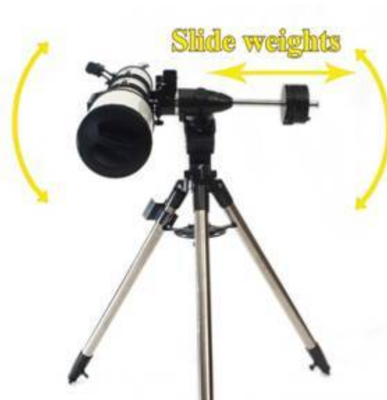
Figure 27: Balancing the scope's right ascension axis.
