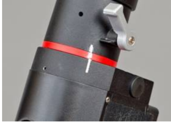
Figure 21: Marking the declination home position.
