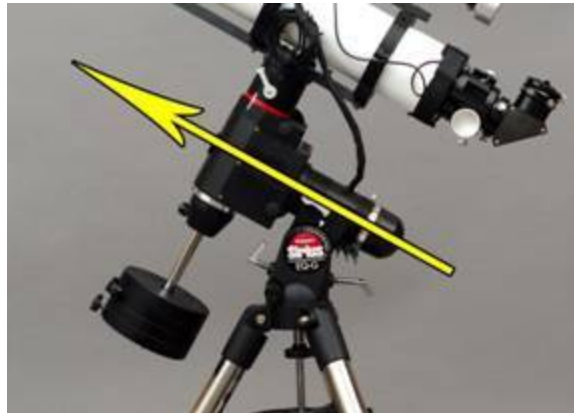
Figure 9: Direction of polar alignment with an EQ mount.
