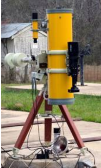
Figure 28:Balancing the nose of a reflector.
