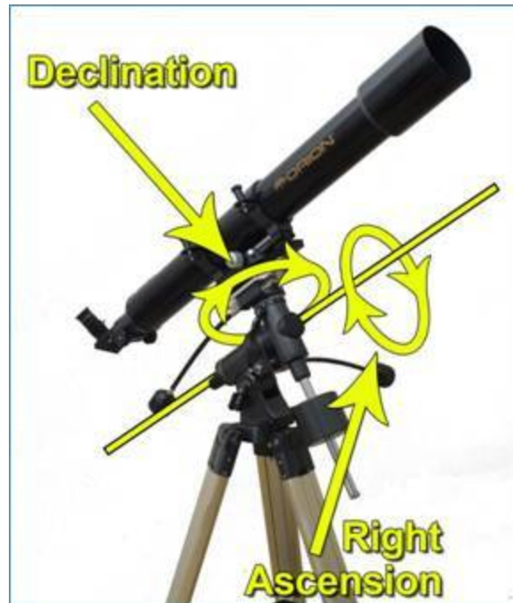
Figure 2: An EQ mount showing its rotational axes.
