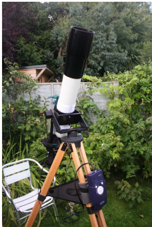
The Televue TV101 on a Gibraltar Mount with Argo Navis setting circles (Image credit: Kevin Berwick)
