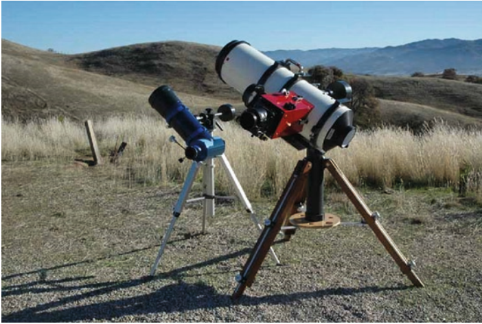
Bob Ayer's folded 6-in. F/5 and 8-in. F/6 rich-field refractors ready for action (Image credit: Bob Ayers)
