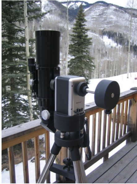
The iOptron MiniTower alt-az GoTo mount with an Astro Physics Traveler (Image credit: John Cameron)
