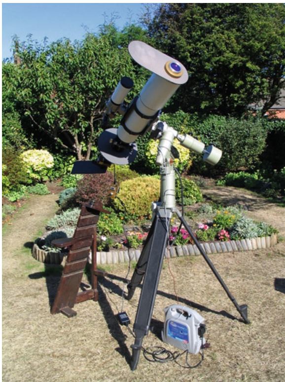
The TEC 140 triplet APO geared up for solar viewing (Credit: Chris Lord)
