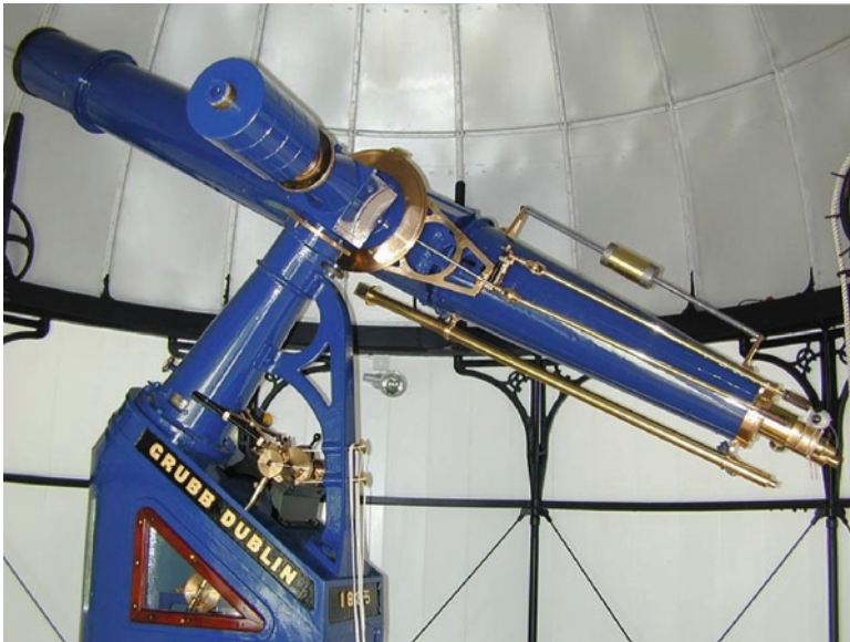
The 10-in. Grubb refractor at Armagh Observatory (Image credit: Armagh Observatory, Northern Ireland)
