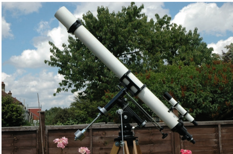
A classic Unitron 4-in. F/15 refractor on its legendary German equatorial mount (Image credit: Skylight Telescopes)
