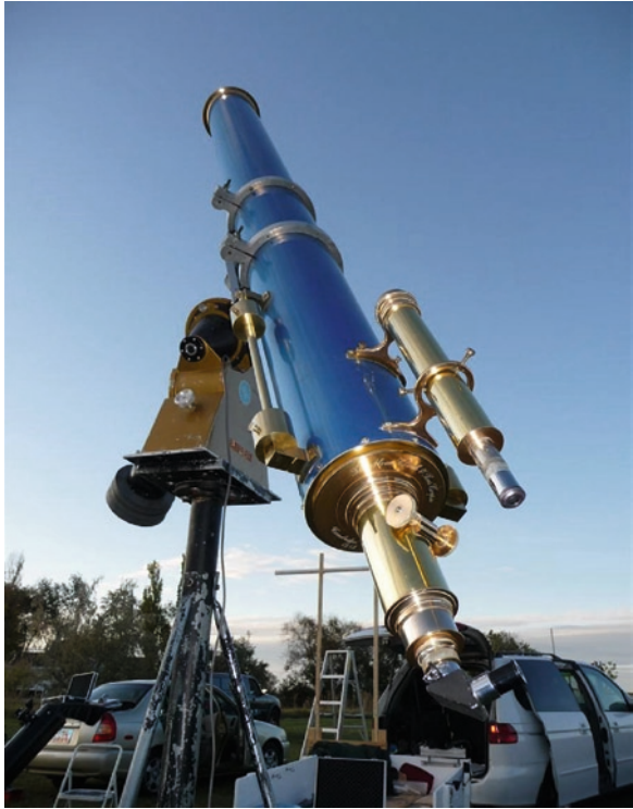
A nicely restored 9-in. Clark refractor made in 1915 (Image credit: Siegfried Jachmann)
