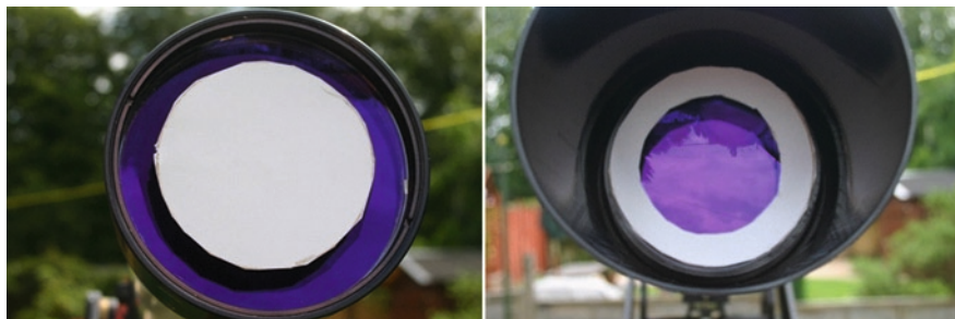
Inner (left) and outer (right) masks used to measure spherical correction (Image by the author)
