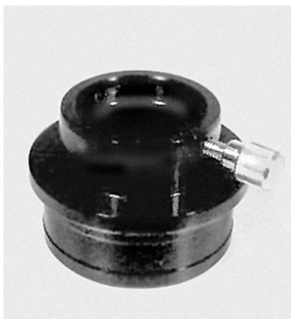
Figure 5.4. Adapters facilitate using different size oculars in the same eyepiece holder. This 2-inch to 1.25-inch (50.8 mm to 31.8 mm) unit by Tele Vue incorporates a pressure ring that grasps the accessory, centering it without marring.
