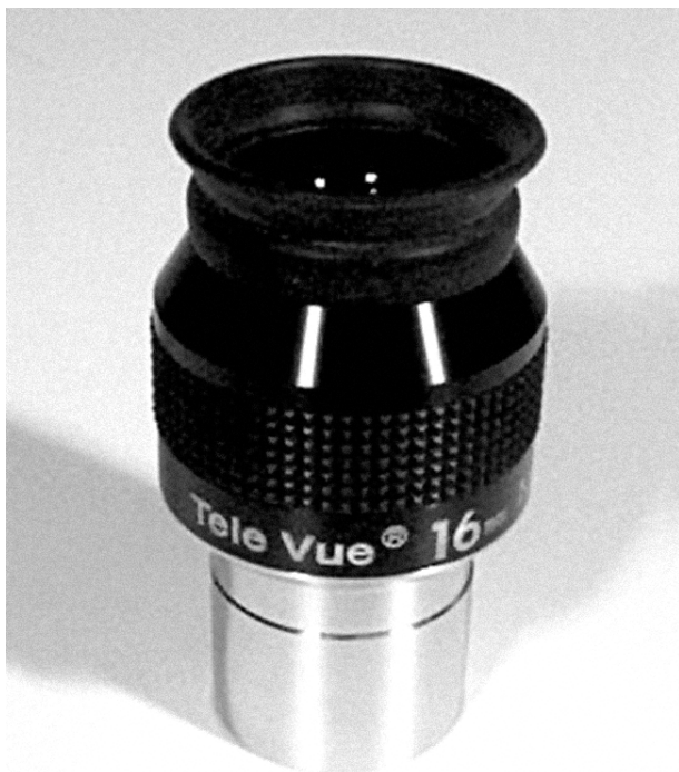
Figure 5.6. An apparent field of 82° makes the Tele Vue Nagler 16-mm Type 5 eyepiece one of the widest-field oculars yet introduced in 1.25-inch format. The design incorporates a telenegative element and has 10-mm eye relief.
