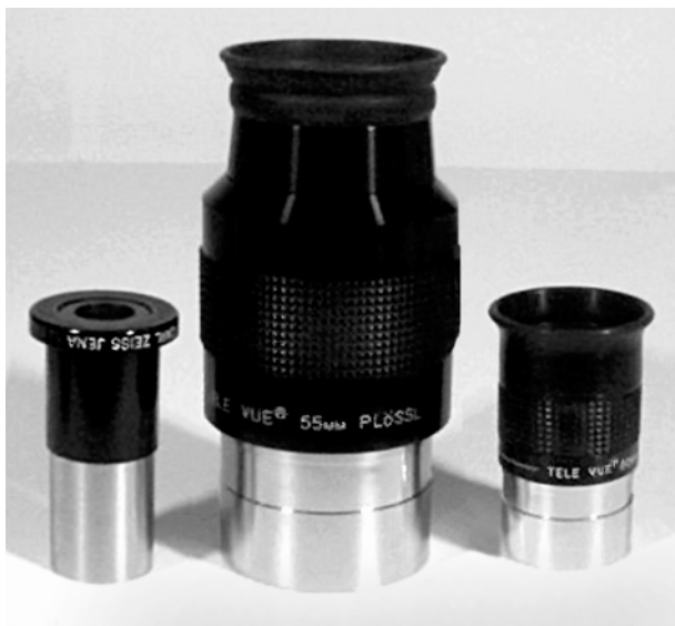
Figure 5.3. Eyepieces of the three standard barrel diameters: 0.965-inch (24.5 mm), 2-inch (50.8 mm), and 1.25-inch (31.8 mm).
