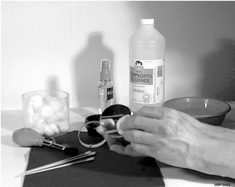
Figure 6.2. Cleaning the crown element of a small air spaced achromat, using surgical cotton and isopropyl alcohol. The selection of recommended materials shown include surgical cotton balls and swabs, an air-bulb cleaning brush, and a proprietary lens cleaning liquid.
