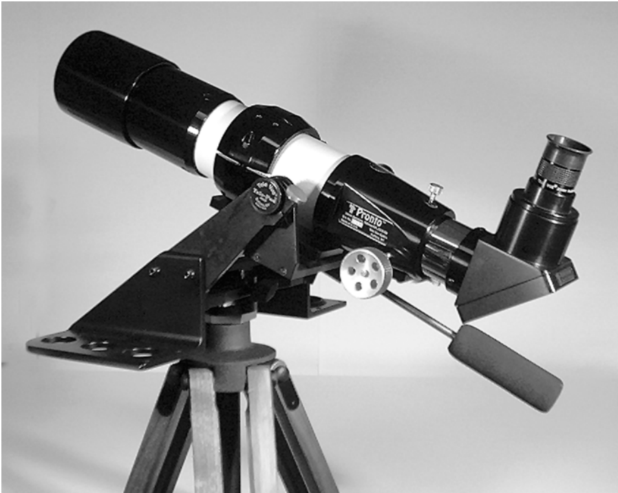
Figure 3.14. This 70-mm aperture semi-Apochromat refractor, a Tele Vue Pronto model, exemplifies the small, fast (f/6.8) new generation of refractors for learners and serious buffs that require a portable glass for air travel and photography. The Gibraltar-model altazimuth mounting is steady and intuitive to use.
