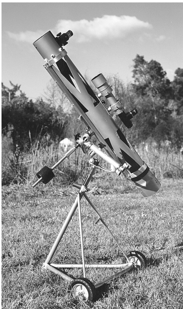
Figure 3.16. An equatorial Newtonian with a 3.4-inch (86 mm) f/14.5 spherical mirror, designed and constructed by the author, has a PVC pipe and aluminum optical tube assembly and a mounting of bicycle parts. Performance at this f /ratio is astonishingly refractor-like, but at the expense of length – the tube measures 54 inches (137 cm).
