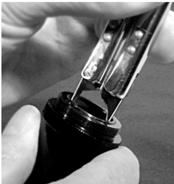
Figure 13.5. Using a small adjustable optical spanner wrench to loosen and remove the eyepiece field stop. Photo: M.D. Pepin.
