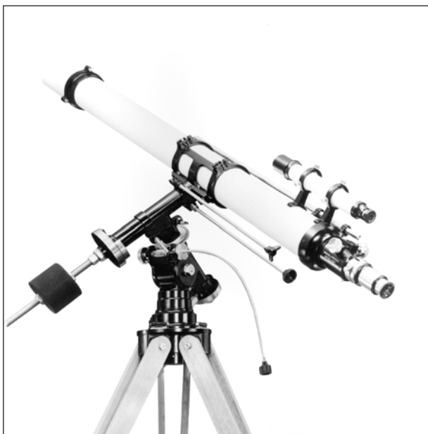
Figure 3.11. A 4-inch f/15 Unitron equatorial refractor has a well-corrected achromatic objective of the Fraunhofer type.
