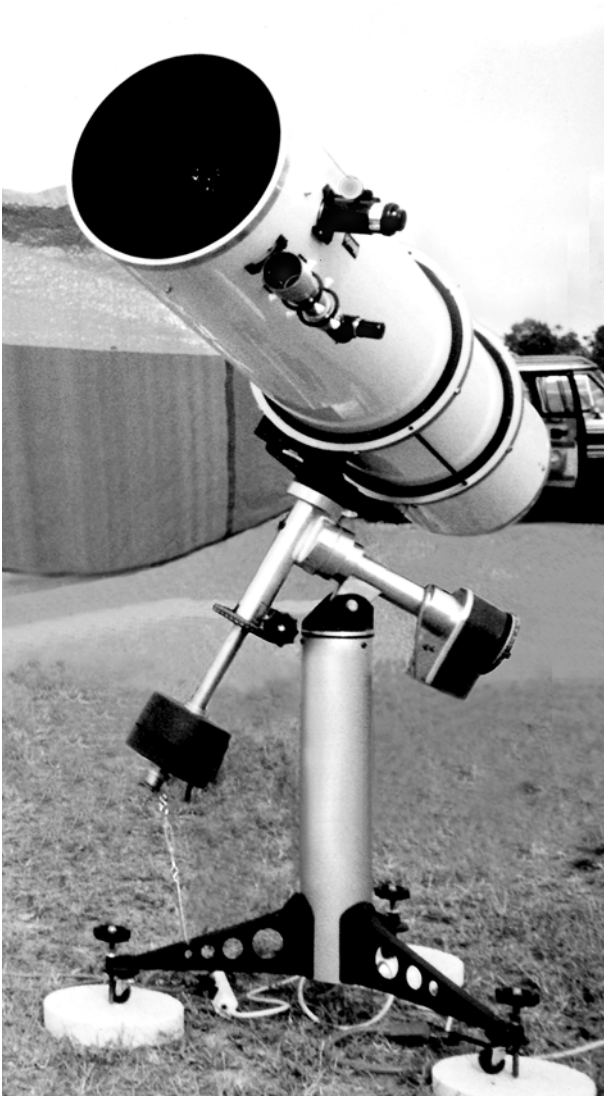
Figure 3.15. Pier-mounted Newtonians like this sidereal-drive 12.5-inch (32cm) f/6 Research-grade Meade set the standard for late 20th-century advanced amateurs. Their size and bulk confine them chiefly to permanent installations. Observers currently favor large Dobsonians for their ease of transport to dark-sky sites.
