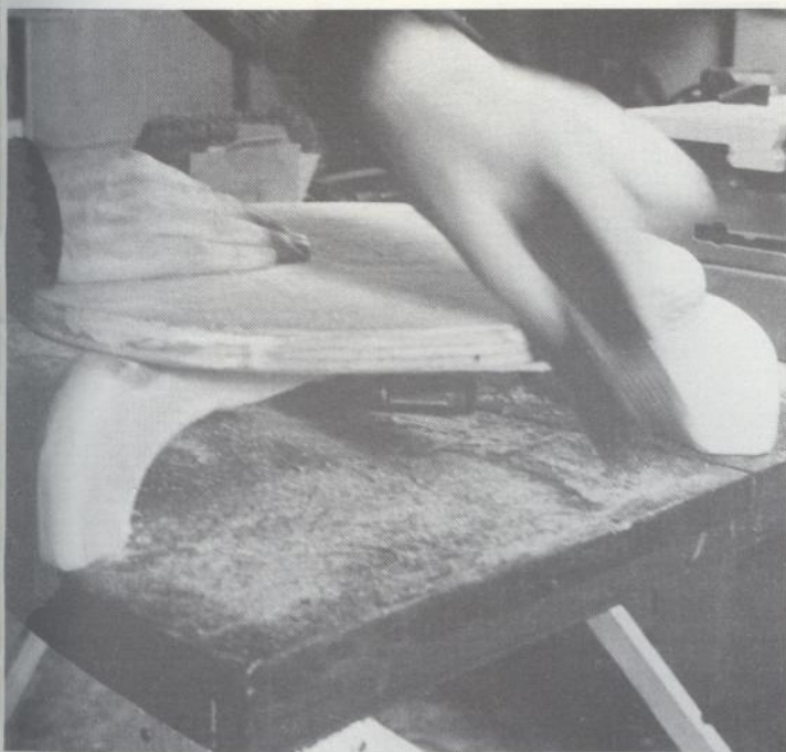
Bevel the edge of the base with a plane or surform tool.
