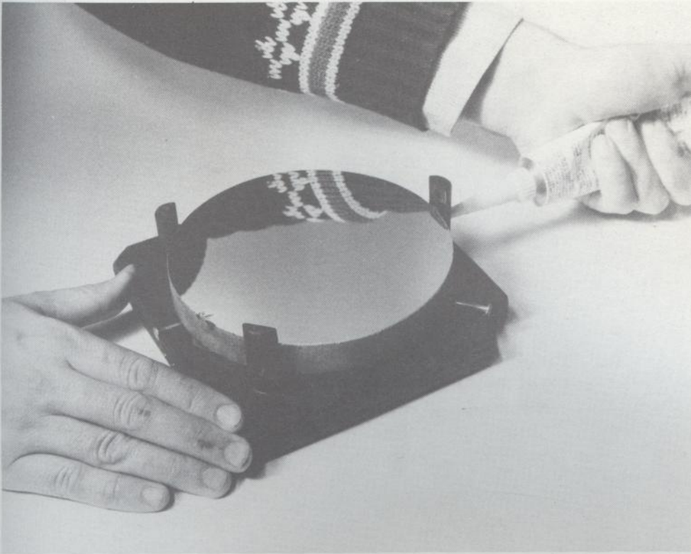
Step 3: Squeeze silicone adhesive through the holes in the mirror holders.
