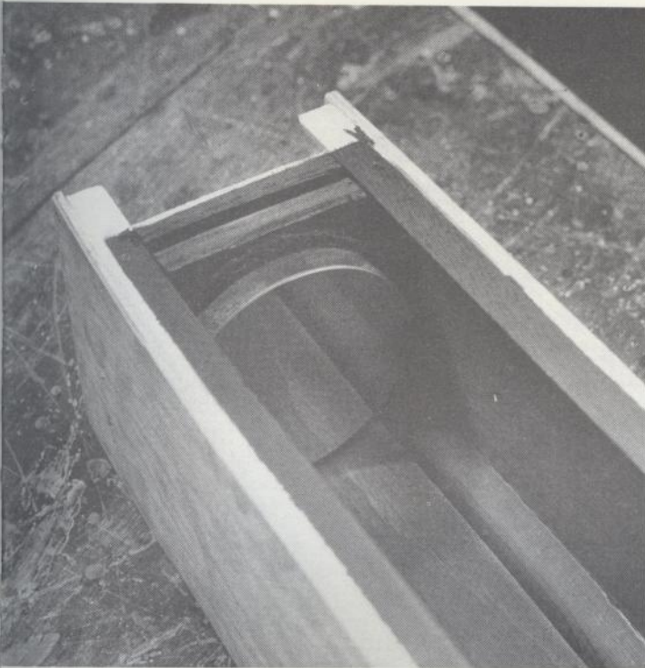
The cell and primary mirror in place at the bottom end of the tube; silicone rubber adhesive holds the mirror in the cell.
