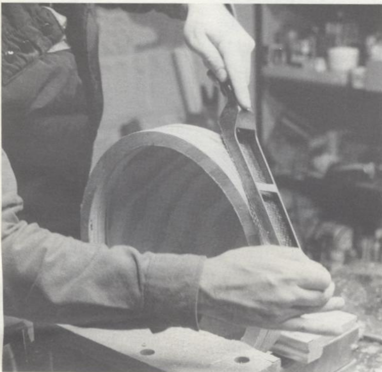
Surform or plane the mirror cell and tube rings to the same outside diameter.
