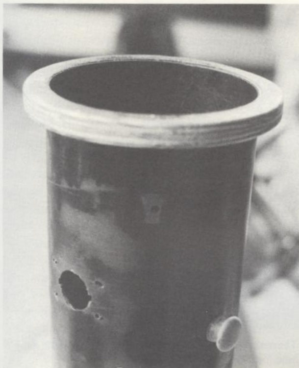
To ensure that edges are sealed, cut all openings (such as the focuser hole) before you coat the tube with primer/sealer.
