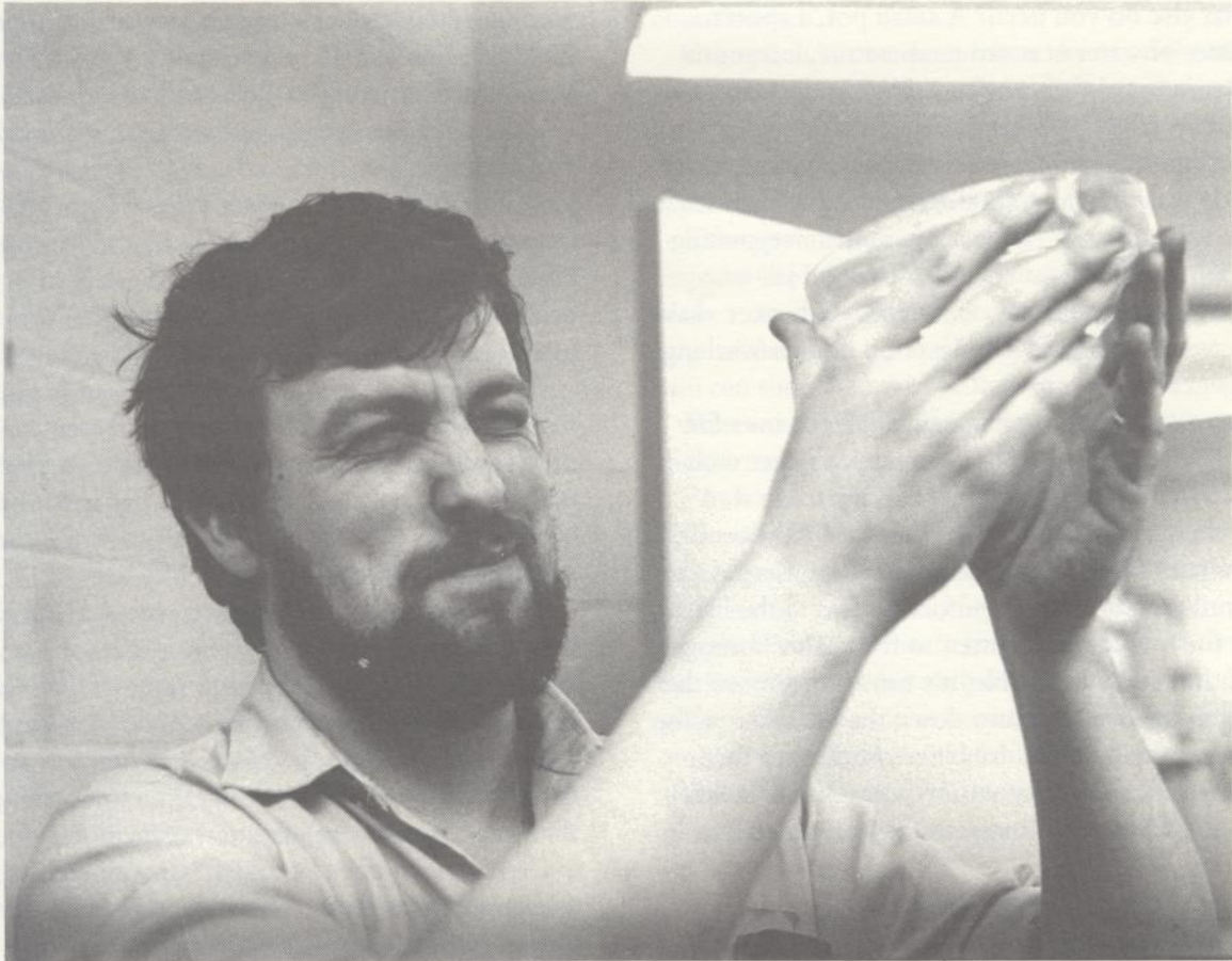
A properly fine-ground surface reflects light when viewed at a low angle.
