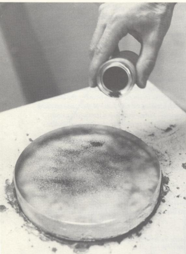
Sprinkle a moderate amount of #80 "Carbo" on the wet tool surface.
