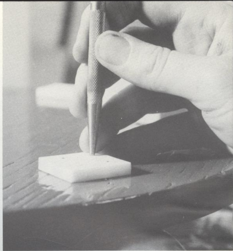
Recess the heads of the brads holding the Teflon pads by half the thickness of the Teflon. (above)
