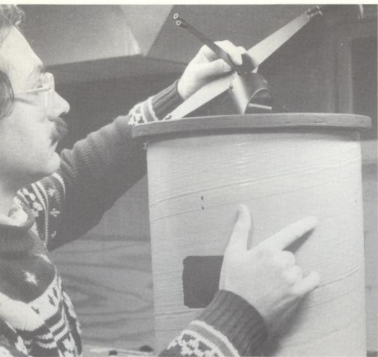
The spider and diagonal go into the front end of the tube; note the bolt holes.
