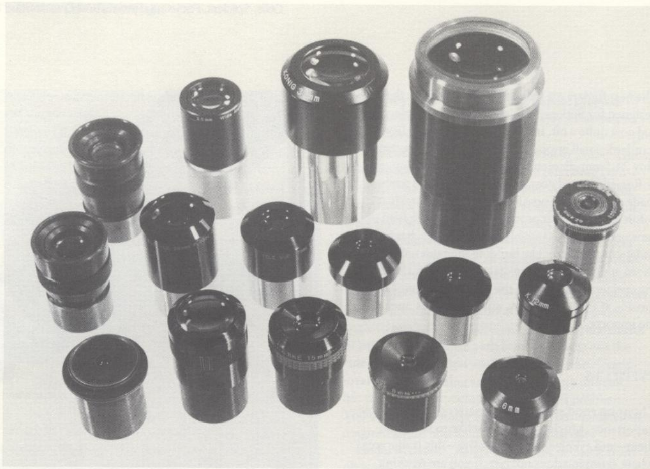
Eyepieces come in all sizes and shapes but in only three standard barrel diameters: 24.5mm, 1¼" (the most common), and 2".
