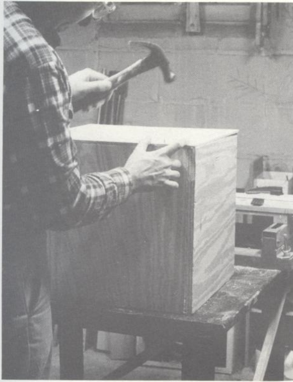
The front board steadies the sides of the rocker box and keeps them perpendicular to the bottom board.
