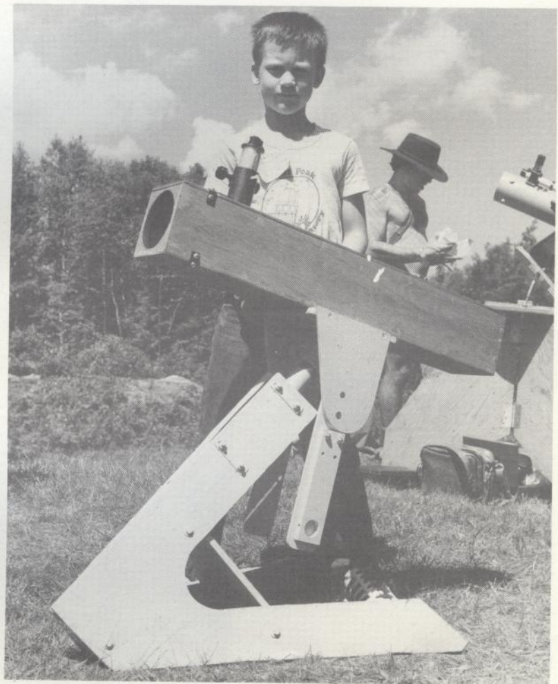
Inverted forks are excellent mounts for a first telescope. Telescope by Alan Beaman, age 8.
