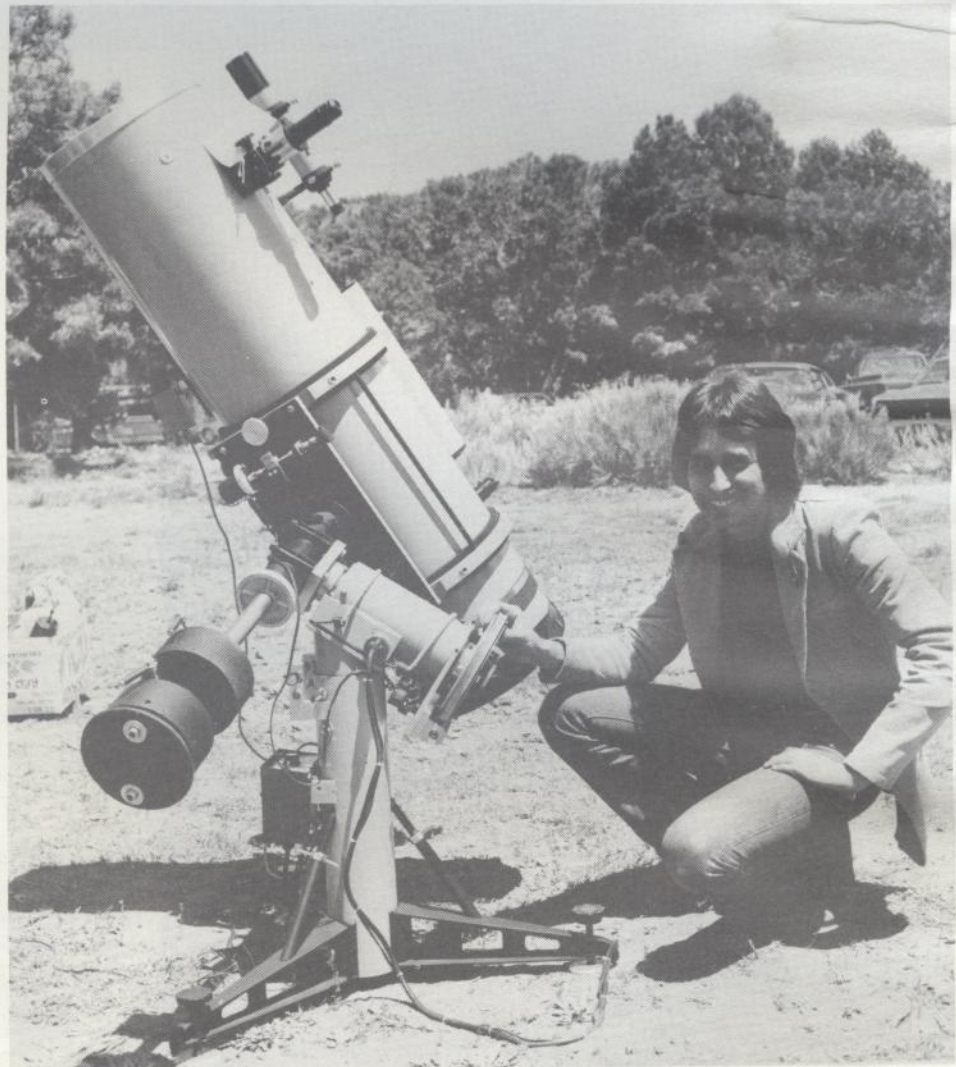
German equatorials have long been popular among amateur telescope-makers. Telescope by Bob Webb.
