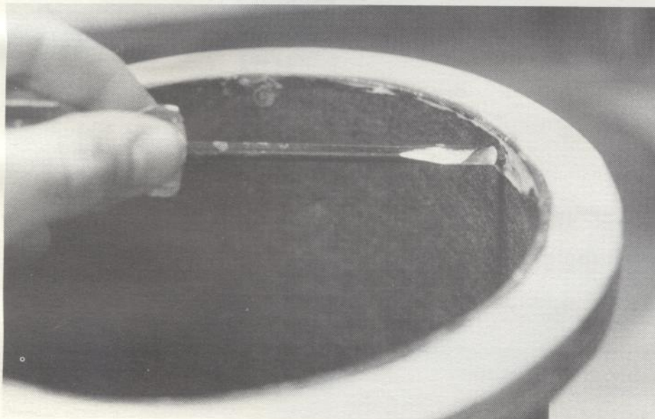
Small wood screws and glue secure tube end rings.
