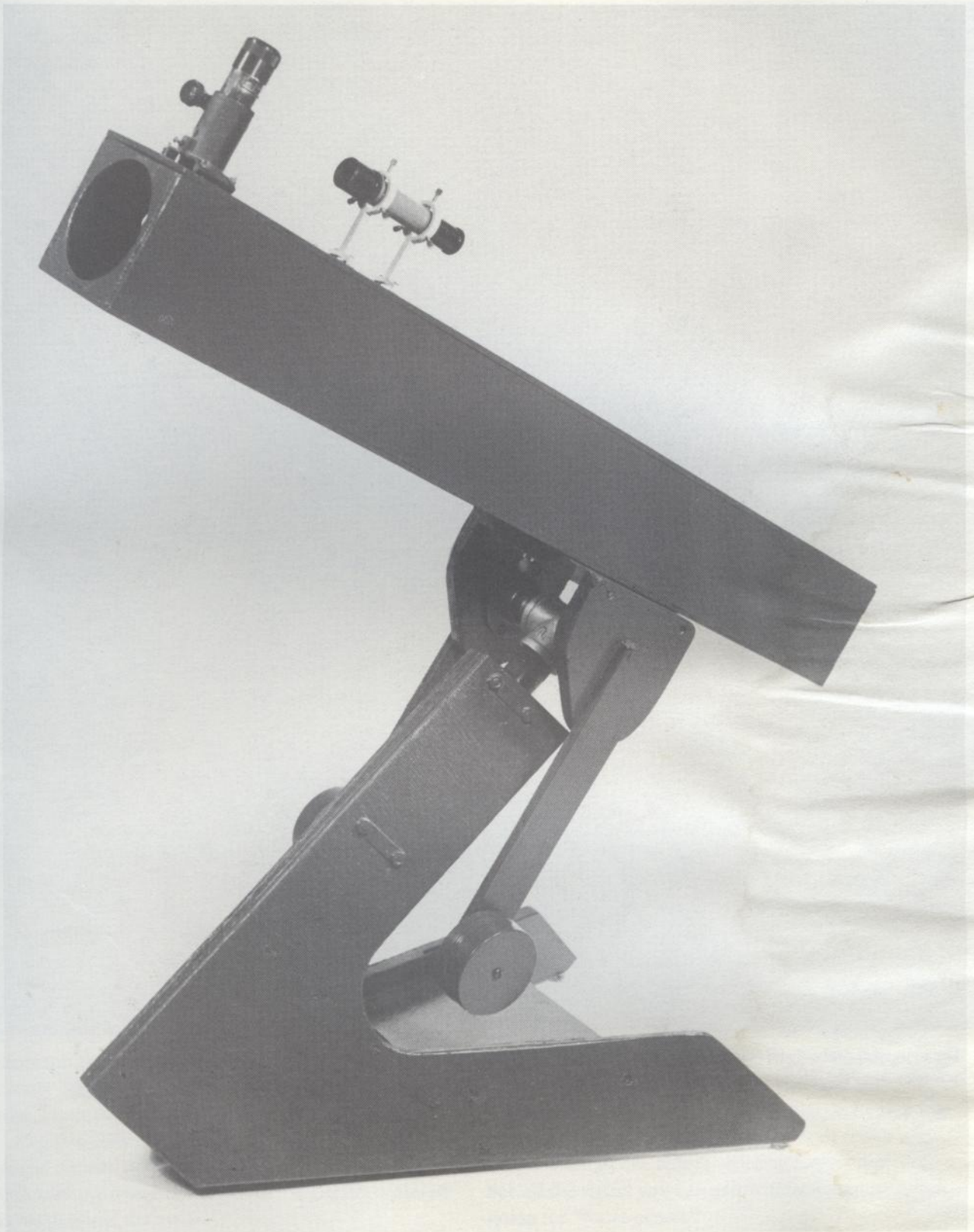
Attach the finder to a convenient spot on the fourth side of the tube.
