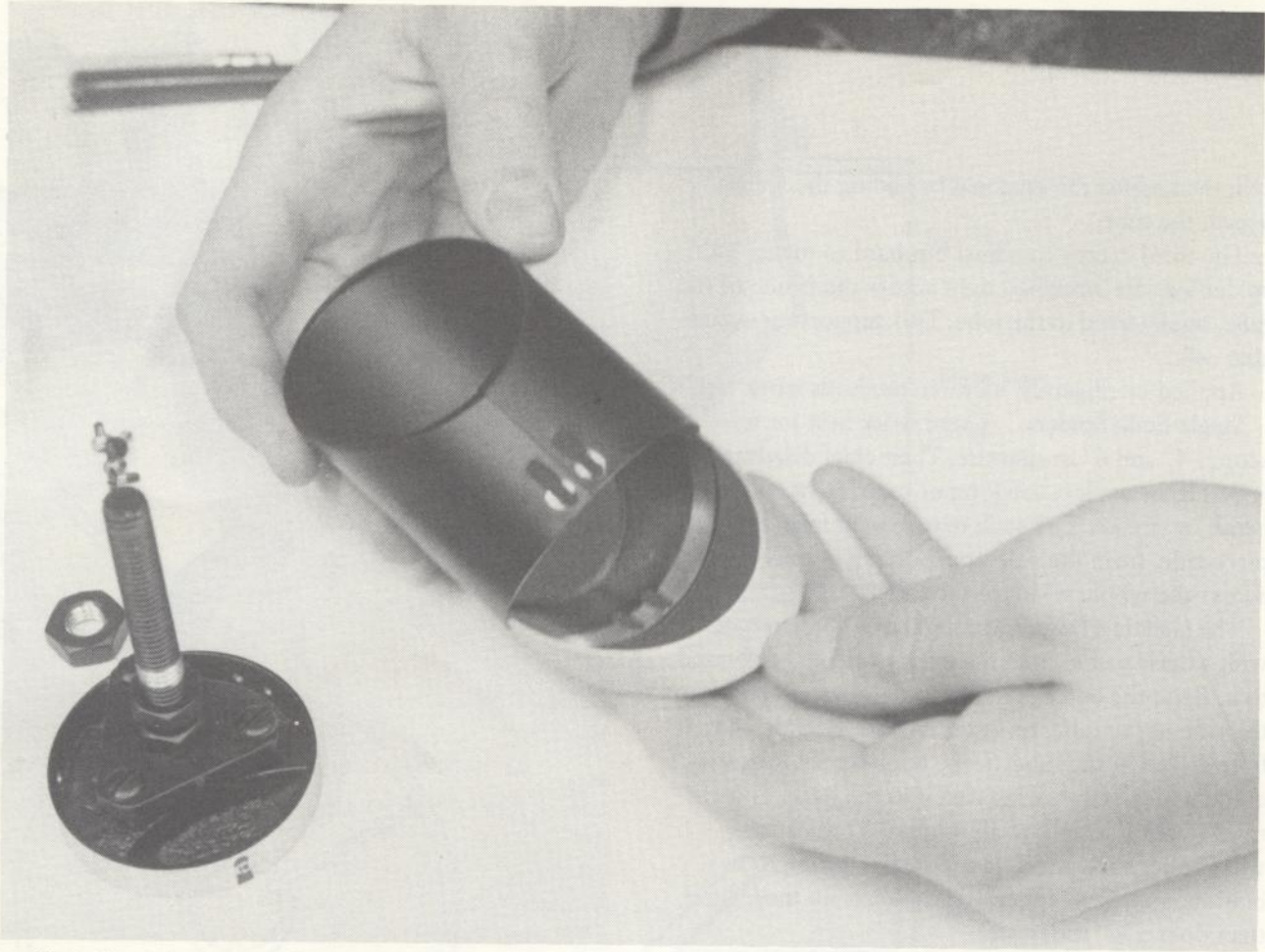
Installing a diagonal mirror in a commercially made adjustable holder; cotton batting presses the diagonal against the front of the holder.
