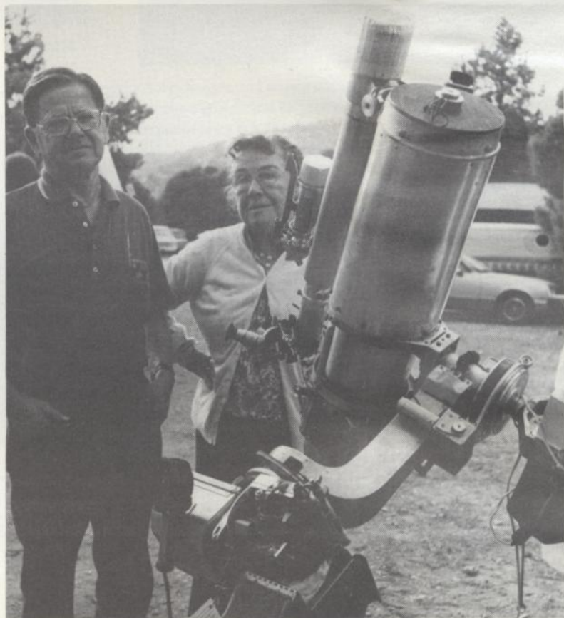
One-armed fork mounts of the asymmetric equatorial class require machining skills to build. Telescope by Orien Ernest.
