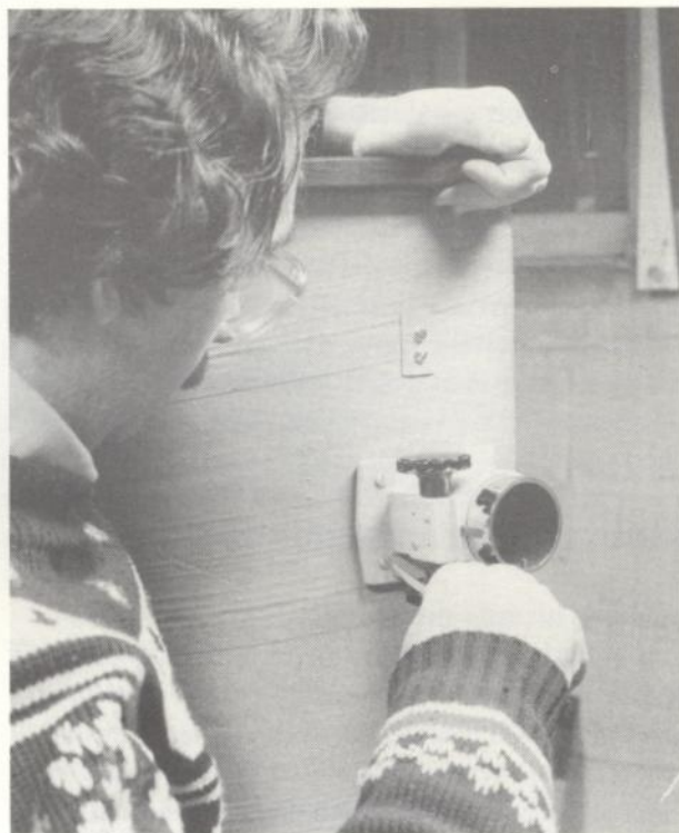
Four bolts hold the focuser to the tube.
