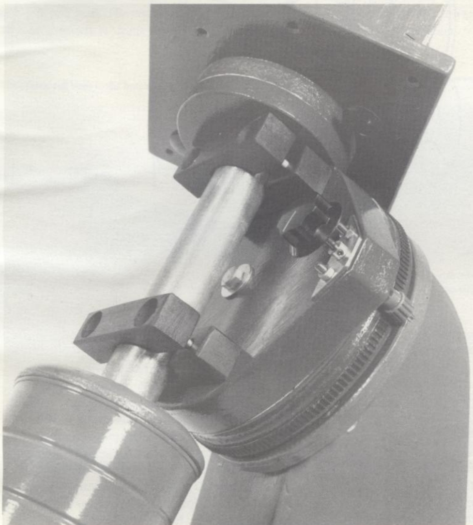
Close-up showing optional right ascension slow motion installed on the polar disk.
