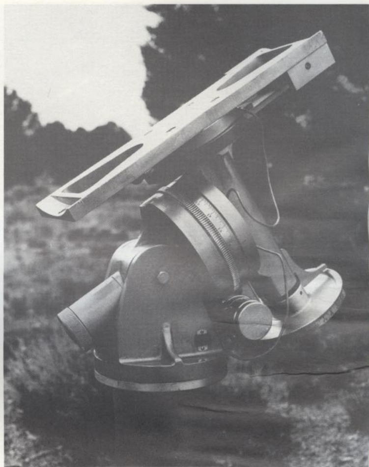
A clock drive and setting circles enhance the usefulness of an equatorial mount for prolonged observing sessions. German equatorial by Bill Shaefer.
