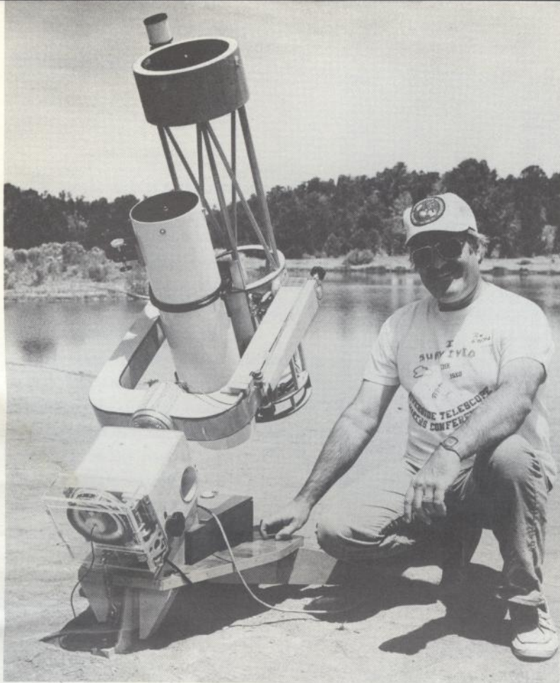
Fork mounts are suitable for relatively light home-built telescopes. Telescope by Tom Greska.
