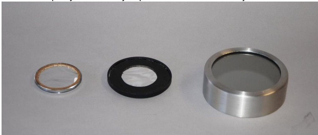
Figure 7-13 DIY solar filters for telephoto lens and telescope
