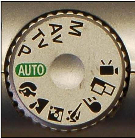
Figure 3-2 Control dial for Canon A70
