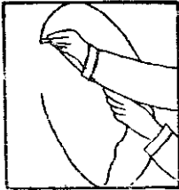
A PAIR OF COMPASSES FOR DRAWING CIRCLES MADE OF ROPE FIG.1
