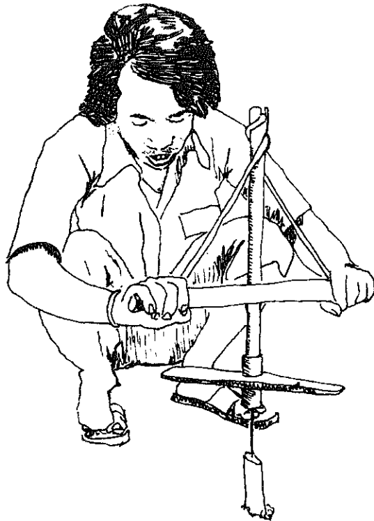
Drilling a buffalo horn knife handle.
