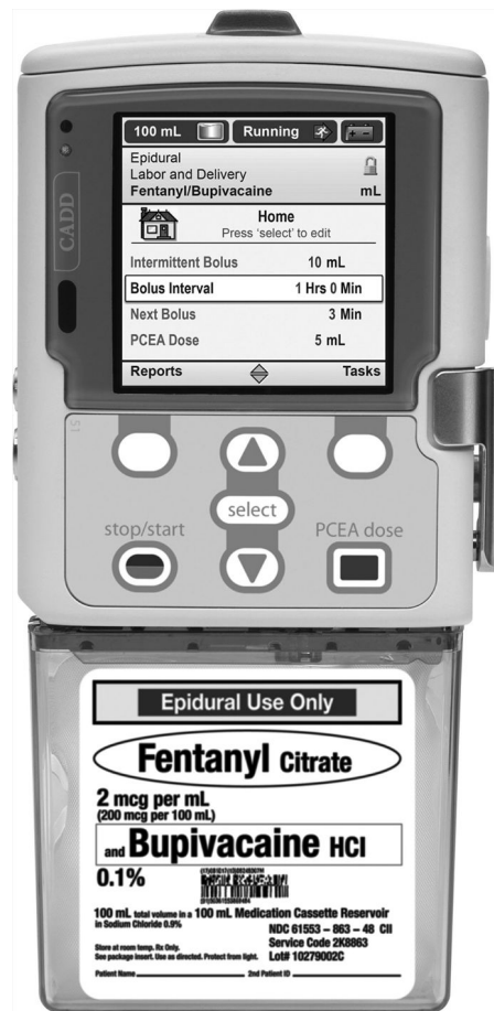
Figure 15.4 A modern smart epidural pump capable of delivering boluses in a patient-controlled epidural analgesia/programmed intermittent epidural bolus mode.
