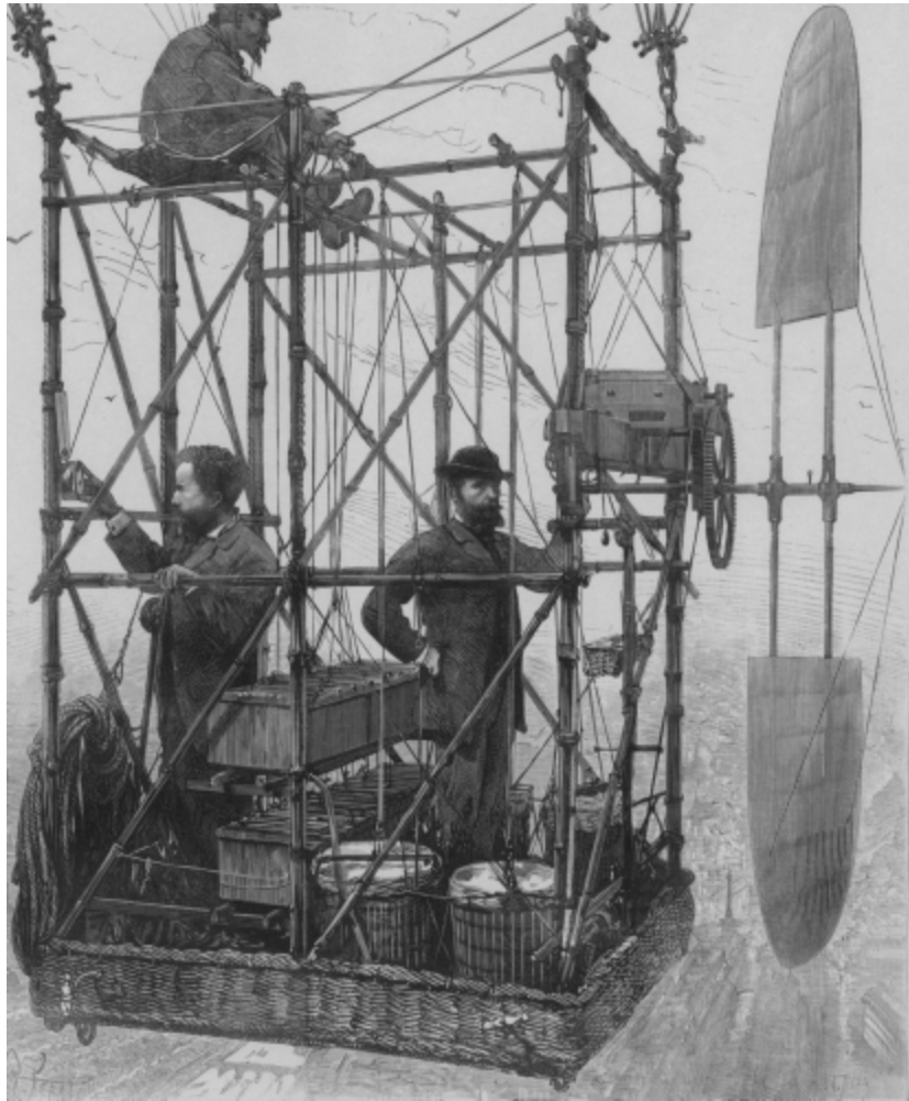
In 1883, the French Tissandier brothers were the first to power a dirigible by electricity. Albert Tissandier (left), Gaston Tissandier (right) and an unidentified man in the basket demonstrate an electric navigational system featuring a propeller. (Library of Congress)
