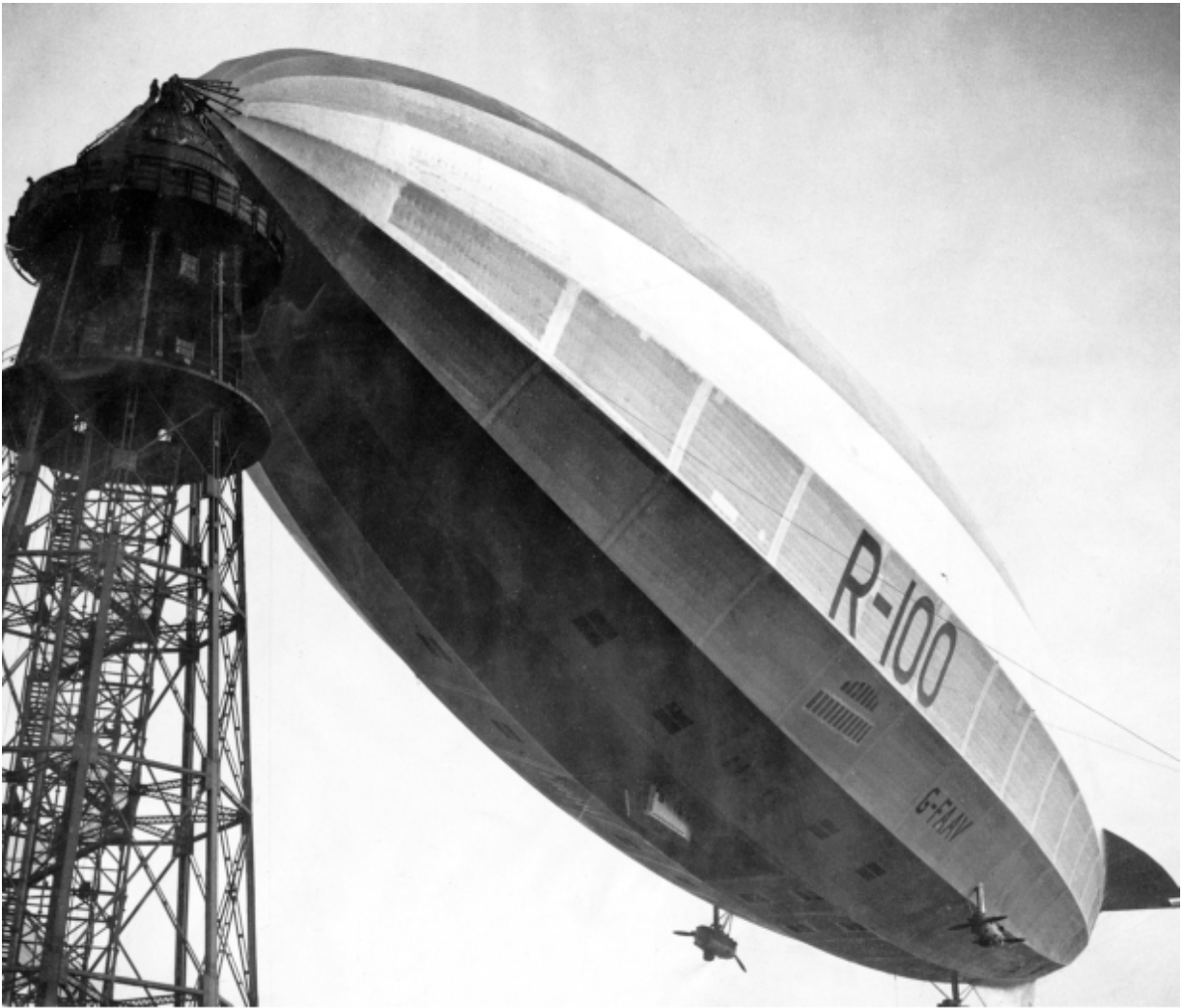
The R100 had five million cubic feet of hydrogen and was fitted with reconditioned Rolls Royce Condor petrol engines. She made her maiden voyage in December 1929 from Howden to Cardington, from where she sailed to Canada in July 1930. (Cody Images)
