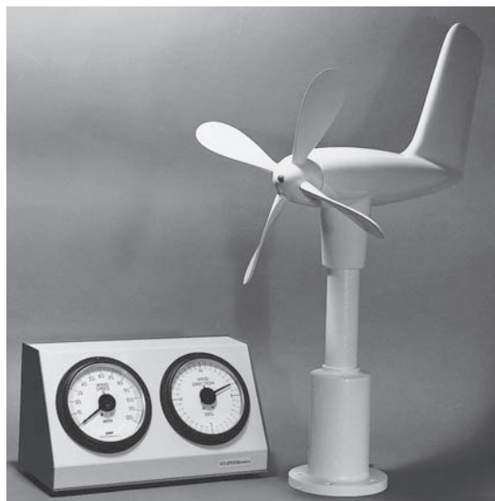
Figure 4-5. An analog wind direction and velocity indicator.
