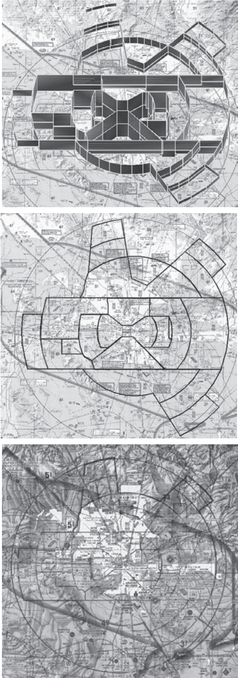
Figure 3–11. Graphic view of Class B airspace and the same airspace as depicted on a sectional chart.
