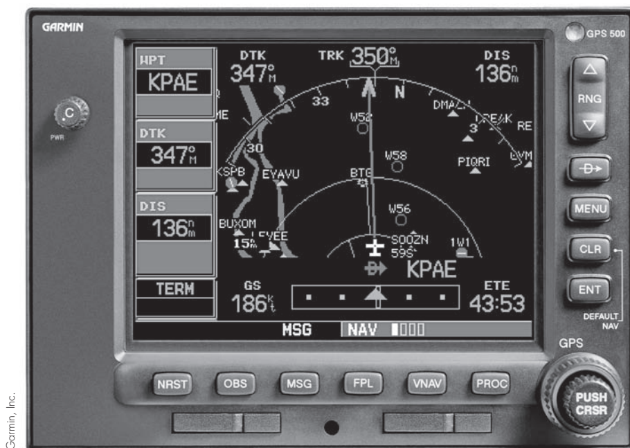
Figure 2–38. Example of a high-end, panel-mounted GPS unit.
