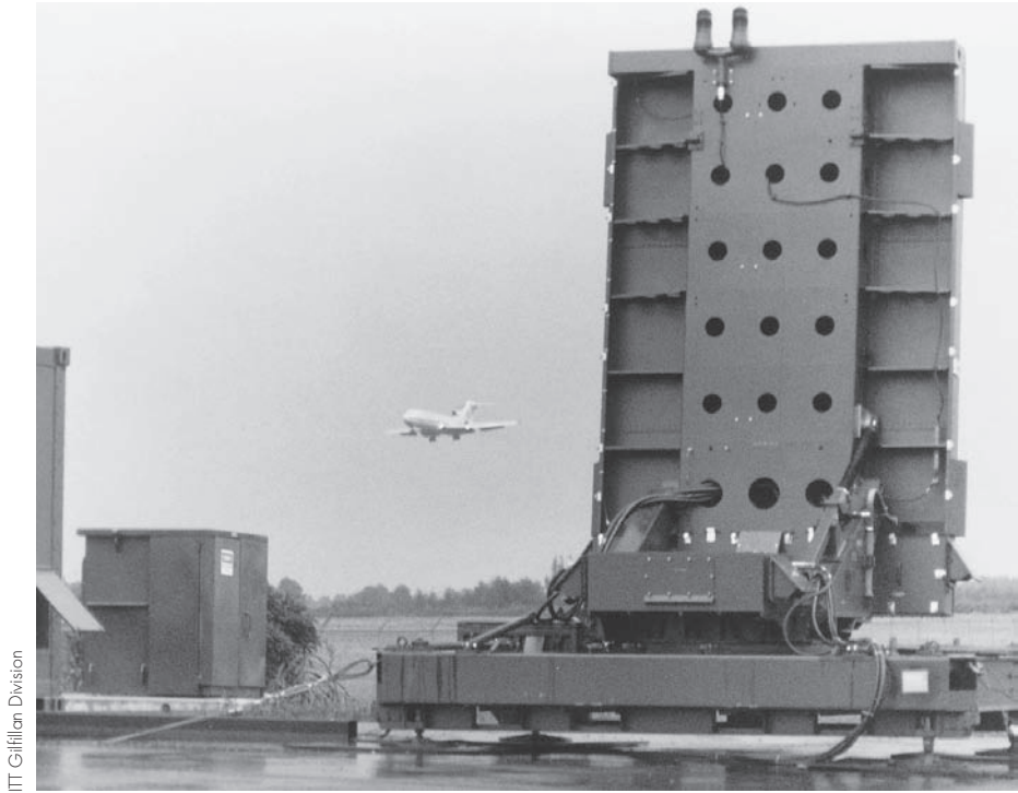
Figure 8–17. Precision approach and automatic landing radar.
