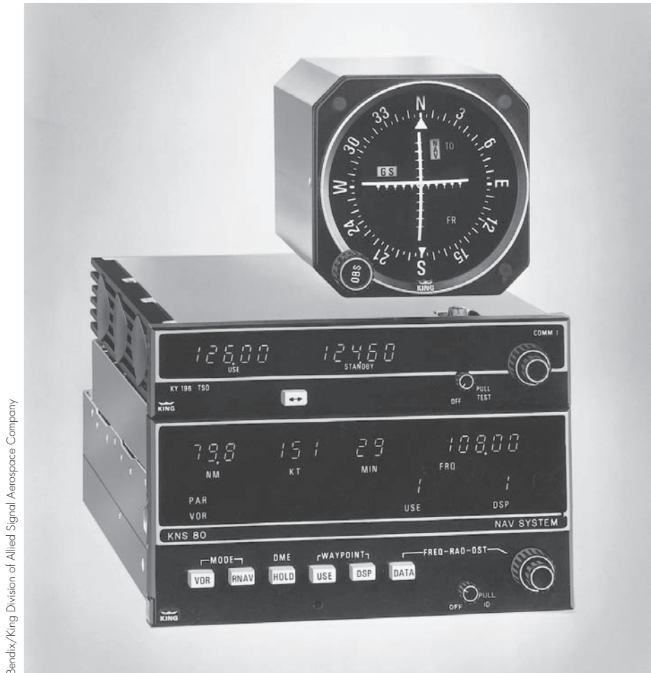
Figure 2–31. A typical light aircraft RNAV system.
