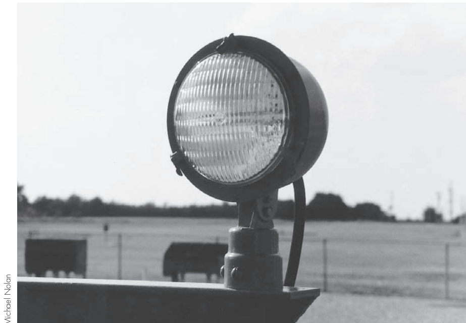
Figure 2–68. A typical high-intensity approach light.
