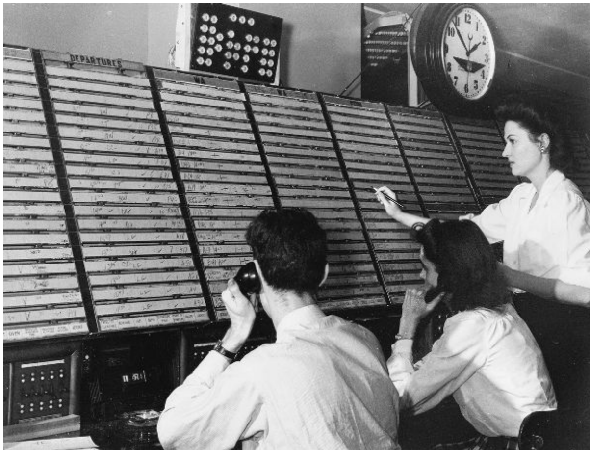
Figure 8: Women controllers, who replaced men during the war, sequencing en route traffic with flight progress strips, replacing blackboards, early 1940s FAA History Office/National Archives (237-G-65-34)
