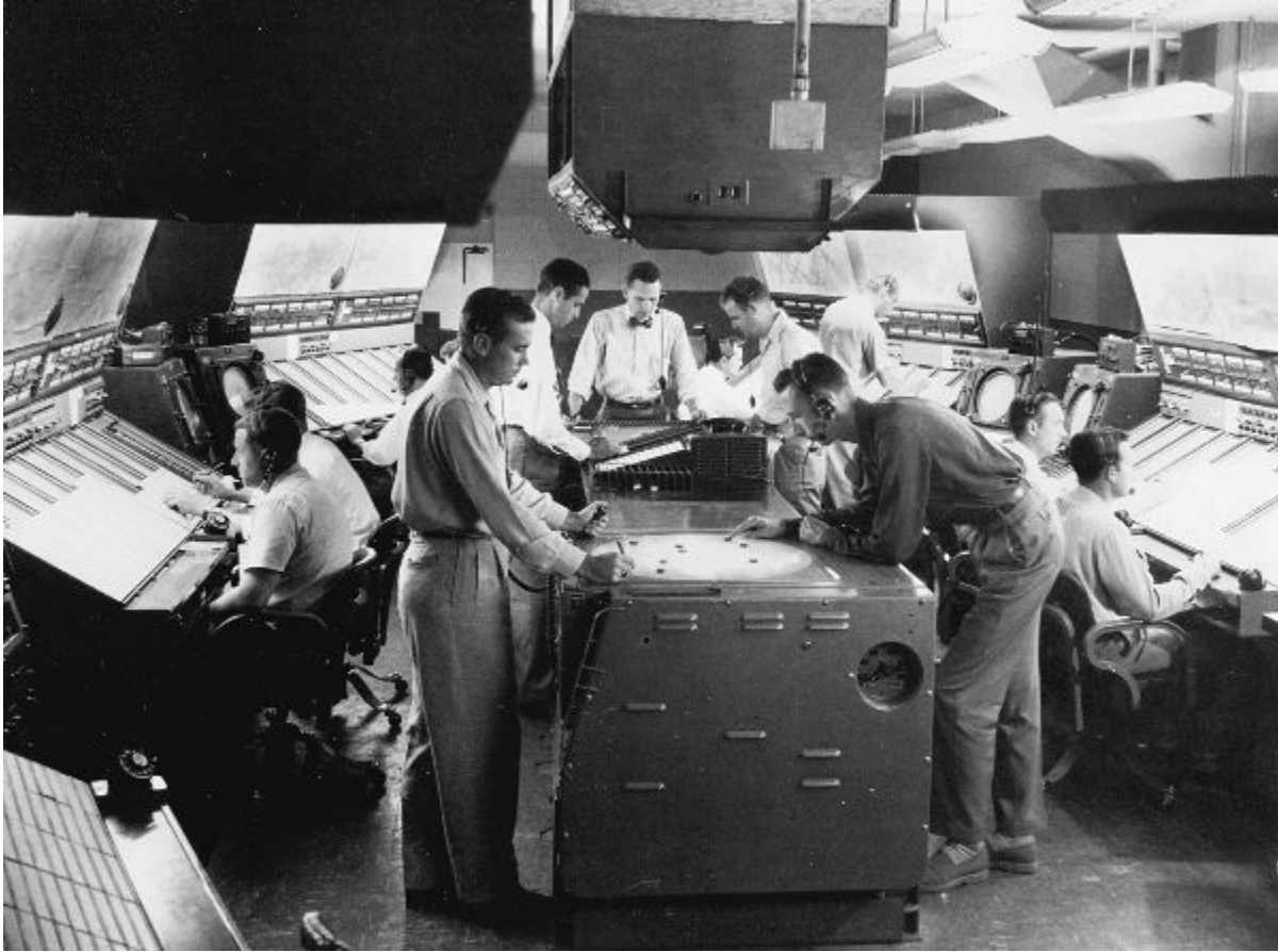
Figure 10: Controllers use flight progress strips to sequence en route traffic and move shrimp boats on flat radar, Washington Air Route Traffic Control Center, 1955 FAA History Office/National Archives (237-G-65-42)
