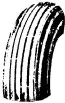
Normal, grooved tire, wear-resistant and having good characteristics on wet runways
