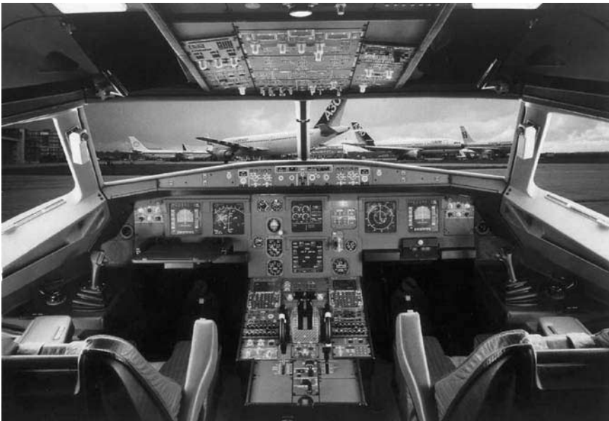
FIGURE 11.49 Airbus cockpit, with lateral side-sticks.
