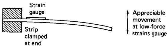
FIGURE 6.34 Strain gauge on flexible strip.
