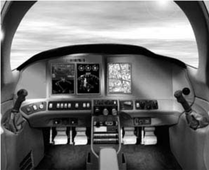
FIGURE 1.10 NASA 507, a certified Lancair Columbia 300 general aviation aircraft, has state-of-the-art avionics, color moving map/GPS, and side-arm control stick.
