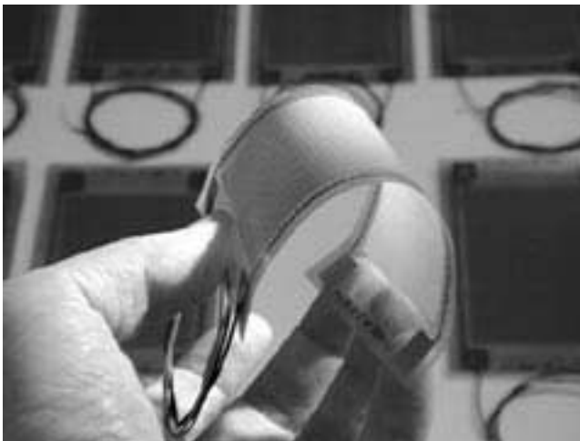
FIGURE 1.11 The Langley Macro-Fiber Composite (LaRC-MFC) is a high performance, low-cost, flexible piezoceramic actuator developed at NASA-Langley Research Center. The solid-state LaRC-MFC is being used to control deflections and vibrations on advanced composite helicopter rotor blades, fixed-wing aircraft control surfaces, and ultralightweight spacecraft components.
