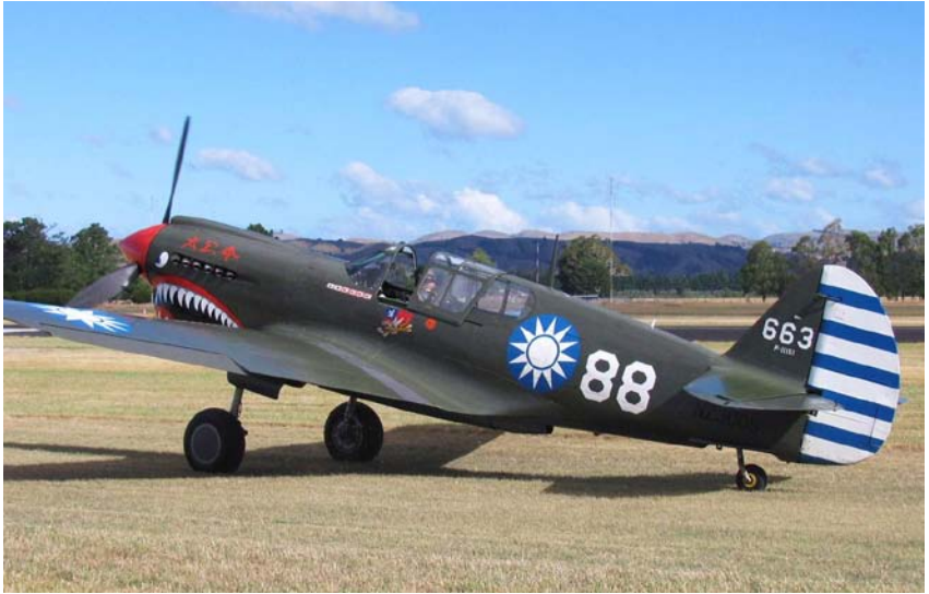
The Curtiss P-40 was equipped with an Allison V-1710 engine powering a Curtiss Electric, three-blade prop.
