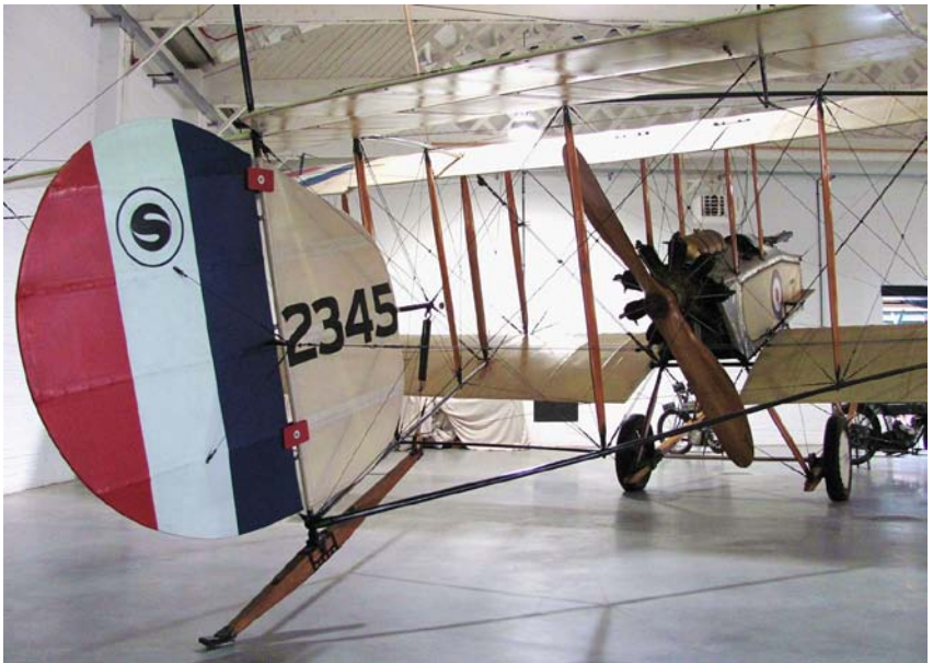
Aircraft from the WW I era used pusher props to leave the front end of the fuselage open for the gunner. This Vickers F.B.5 Gunbus is located in the RAF Hendon Museum, London.
