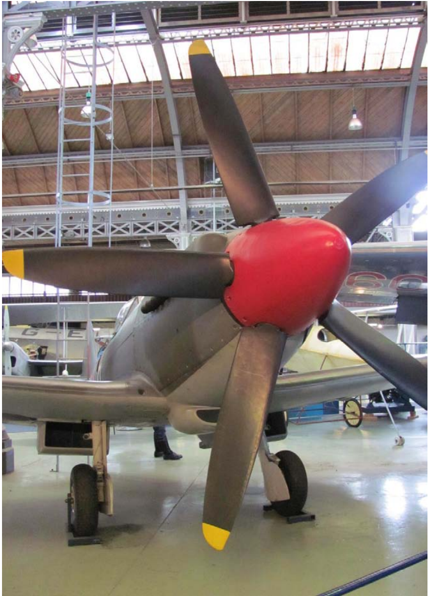
The Supermarine Spitfire FR XIVe has a five-bladed propeller. Manchester Air Museum, England, is the home to this aircraft.
