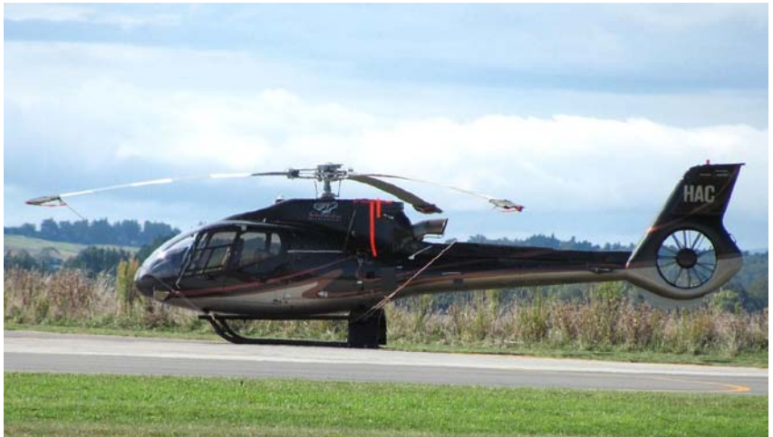
The Eurocopter EC 130 with a tail rotor Fenestron, which reduces tail rotor noise by 50% due to its unevenly spaced blades.
