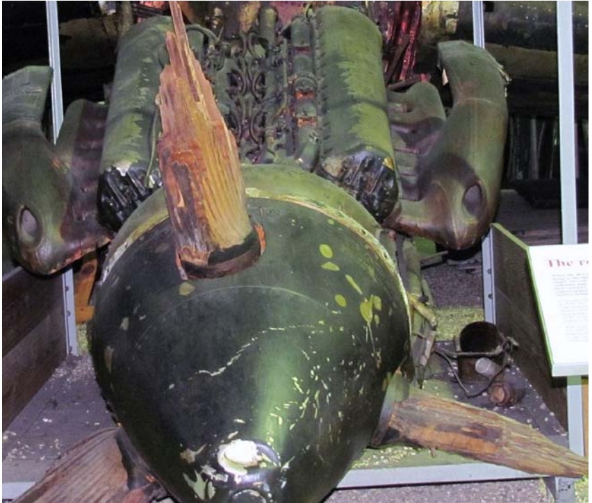
The wooden prop blades on this Handley-Page Halifax II bomber were sheared off during its war time crash-landing. The Halifax is displayed as recovered in the RAF Hendon Museum, London.
