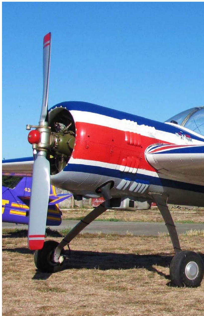
A wide chord prop with squared off tips adorns this Yak-55M aerobatic aircraft.
