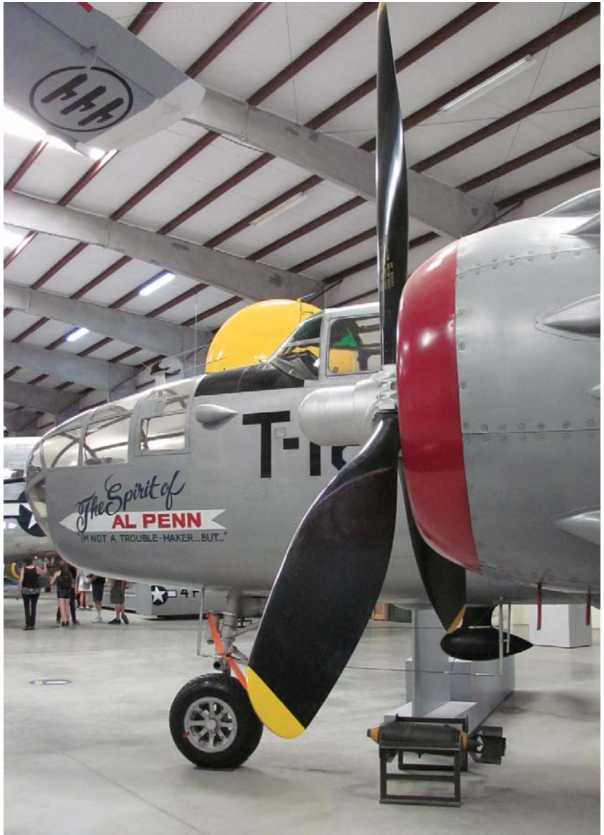
The North American B-25J Mitchell bomber has rounded prop tips, typical of many aircraft until the 1960s when square tips became common. Pima Air & Space Museum, Tucson, Ar, is home to this aircraft.
