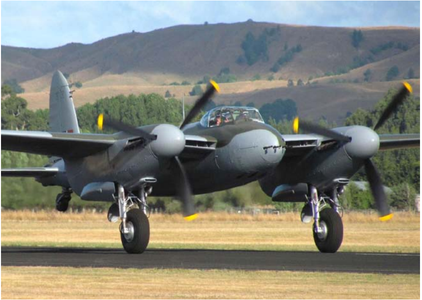
A DeHavilland DH.98 Mosquito on take-off with both props in fine/flat pitch. This is the World's only airworthy Mosquito in 2014.
