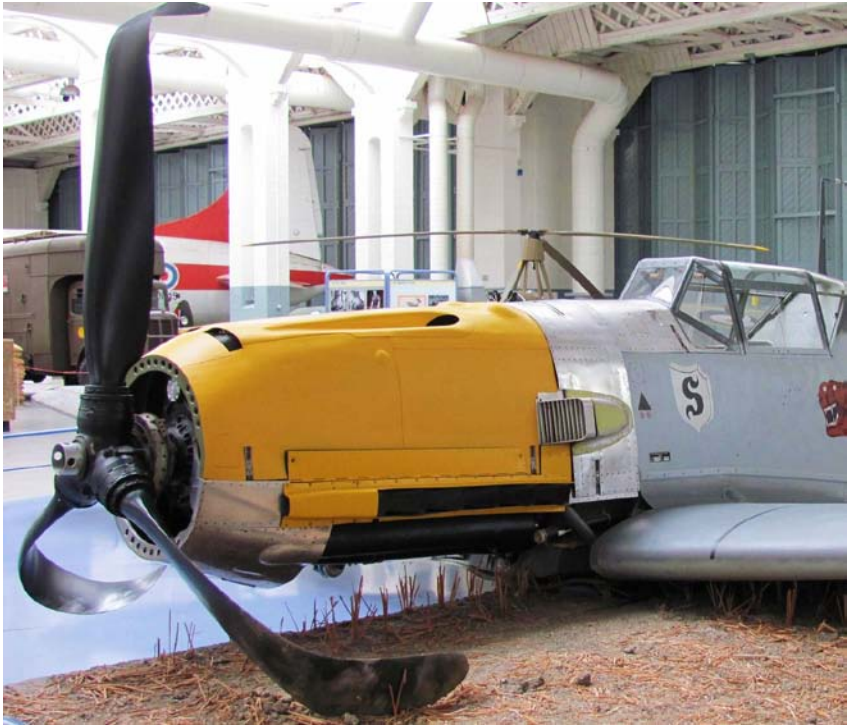
This Messerschmitt Bf 109e received prop damage in the crash-landing after being shot down in England, in 1940. This aircraft is on display in the Imperial war Museum, Duxford, UK.
