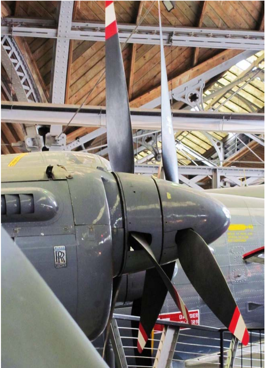
Four sets of contra-props power the Avro Shackleton AEW.2 maritime patrol aircraft. This aircraft resides in the Museum of Science & Industry, Manchester, England.
