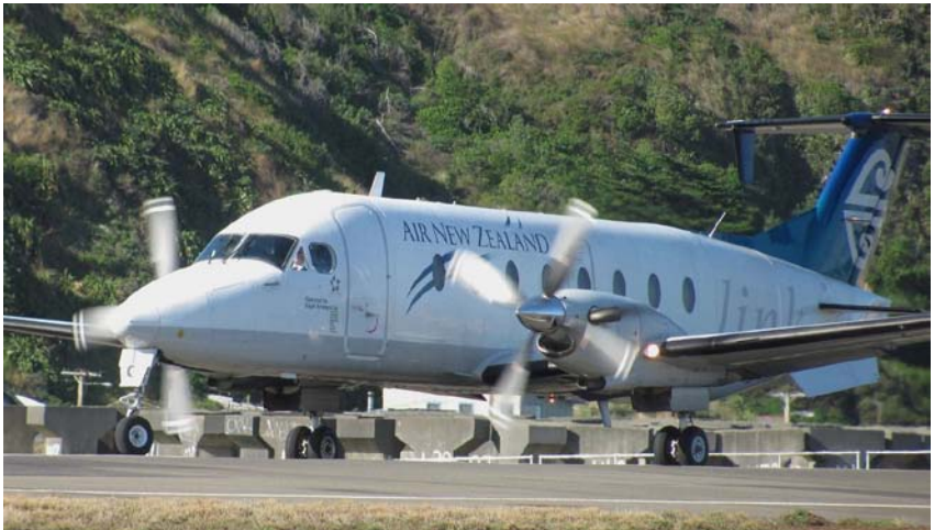
The Beech 1900D commuter airliner has two PT6A-67 free-shaft turboprop engines rated at 1279 SHP each.
