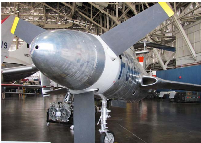
The Republic Thunderstreak XF-84H used to flight-test the three-blade Aero Products supersonic propeller. The research aircraft is now housed in the National Museum of the USAF in Dayton, Ohio.
