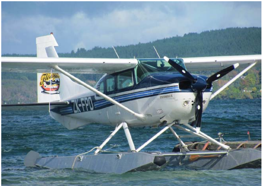
This Cessna 206 Stationair floatplane is powered by a three-blade McCauley propeller.
