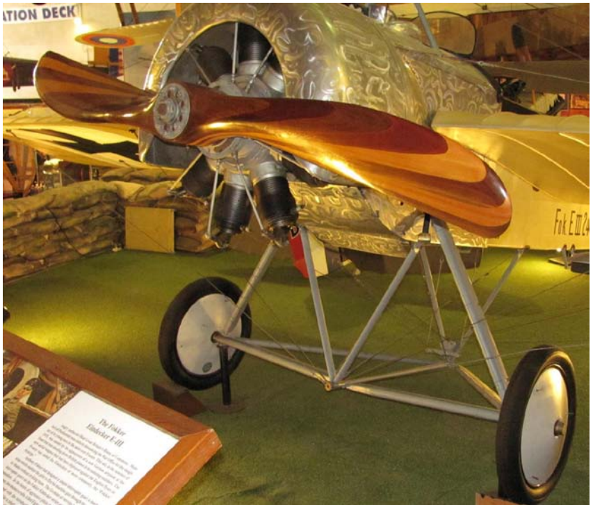
A Fokker E-III Eindecker of WW I era with a carved, laminated and scimitar shaped propeller. This aircraft is located in the Air & Space Museum, San Diego, Calif.
