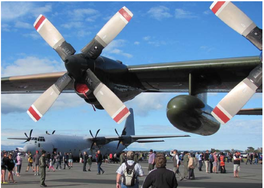
The Lockheed C-130J with six-blade scimitar props in the distance, is overshadowed by the older Lockheed C-130H with four-blade, square-tip propellers.
