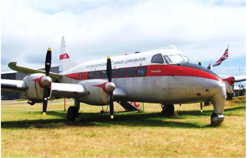
The DeHavilland Mark 1 Heron was the world's smallest airliner with four prop/engines.
