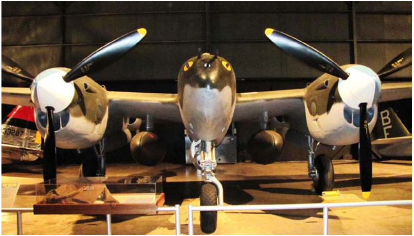
A front-end view of a Lockheed P-38 Lightning showing its counter-rotating propellers. This aircraft is located in the National Museum of the USAF, Dayton, Ohio.
