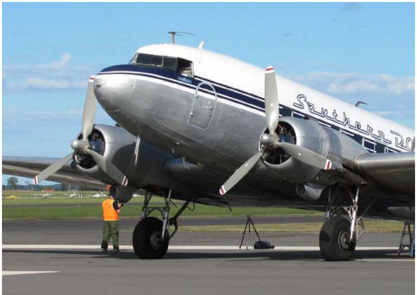
The Douglas DC-3 uses Hydromatic double-acting and feathering propellers.
