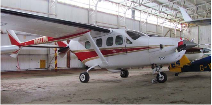
The Cessna 336/337 Skymaster has centreline mounted engines mounted at each end of the fuselage.
