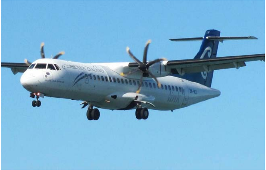
The Aerospatiale ATR-72 turbo prop aircraft have modern six-blade scimitar shaped props.
