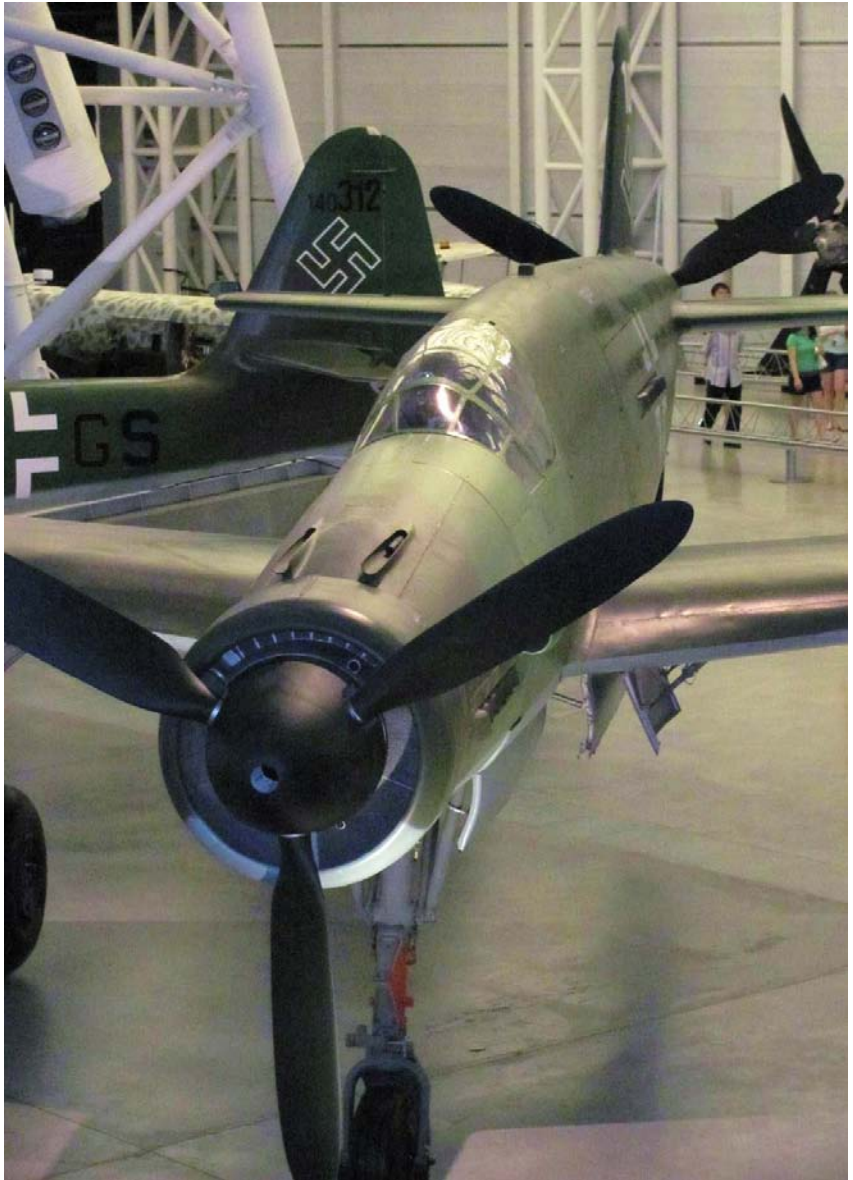
The Dornier Do-335 Pheil is a WW II centre-line thrust aircraft. Two Daimler-Benz V-12 piston engines of 1750 BHP each drive three-blade feathering props. This sole example is located in the Udvar-Hazy Centre, Chantilly, Virginia, USA.
