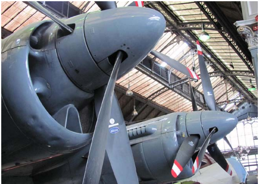
The Avro Shackleton bomber has four engines each powering a set of contra-props. This aircraft is in the Manchester Air Museum, England.
