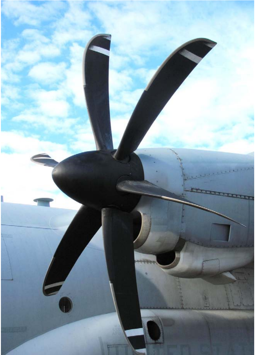
A close up view of the six-blade scimitar propellers of the Lockheed C-130J Hercules.
