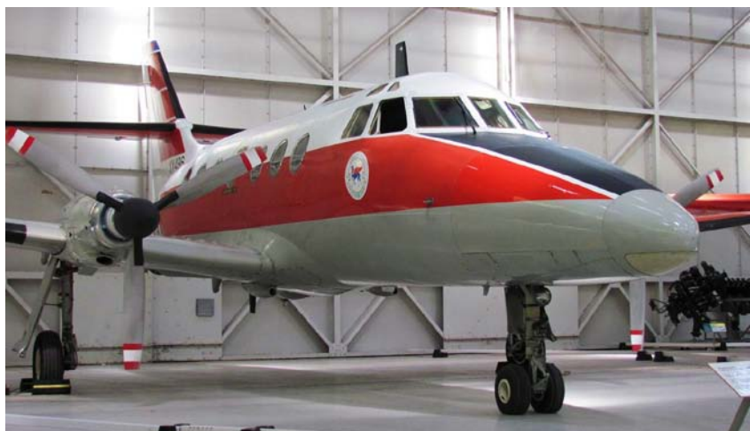
The Scottish Aviation Jetstream 1 is powered by twin Turbomeca Astazou fixed-shaft turboprop engines. This aircraft is located in the RAF Museum Cosford, England.
