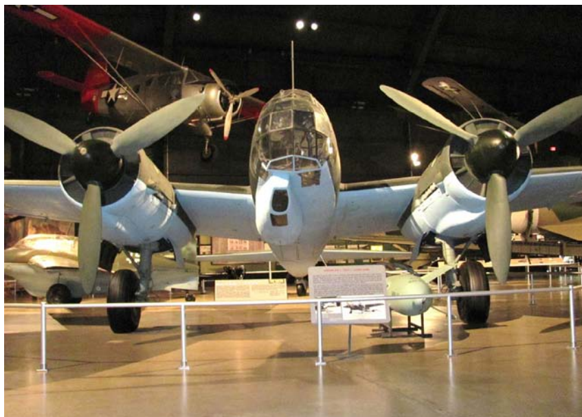
The Junkers JU-88 bomber with three-blade, wooden propellers. The National Museum of the USAF, Dayton, Ohio, is the home for this aircraft.
