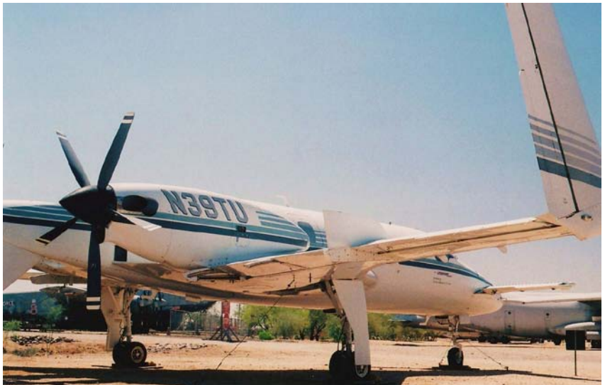
The Beech 200 Starship with twin five-blade pusher props, located at the Pima Air & Space Museum, Tucson, Ar.
