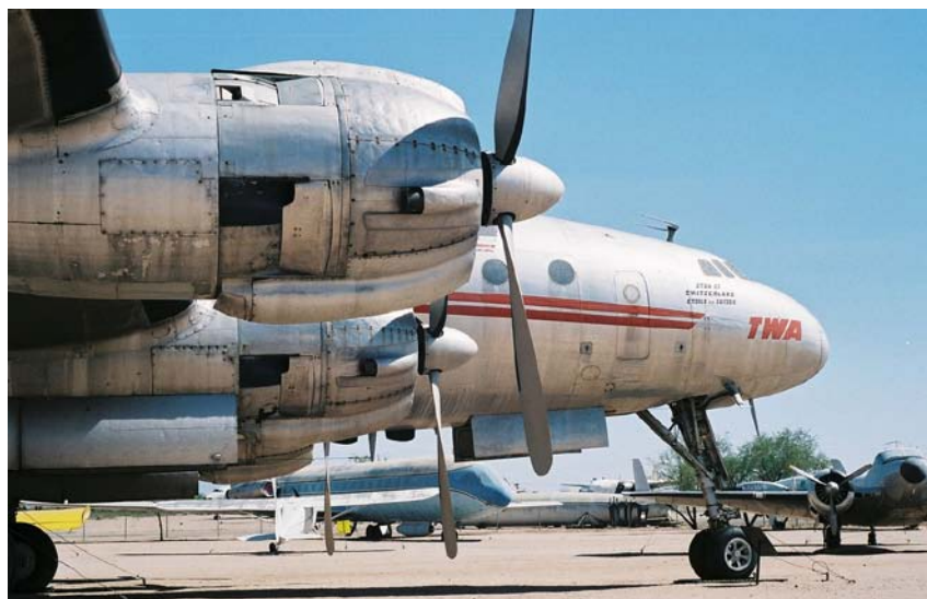
The Lockheed (L-1049) Constellation was the last of the piston/prop airliners to be built. It has four Wright R-3350 radial engines of 2200 BHP each, driving Hamilton Standard or Curtiss Electric constant-speed propellers. This aircraft is located in the Pima Air & Space Museum, Tucson, Arizona.
