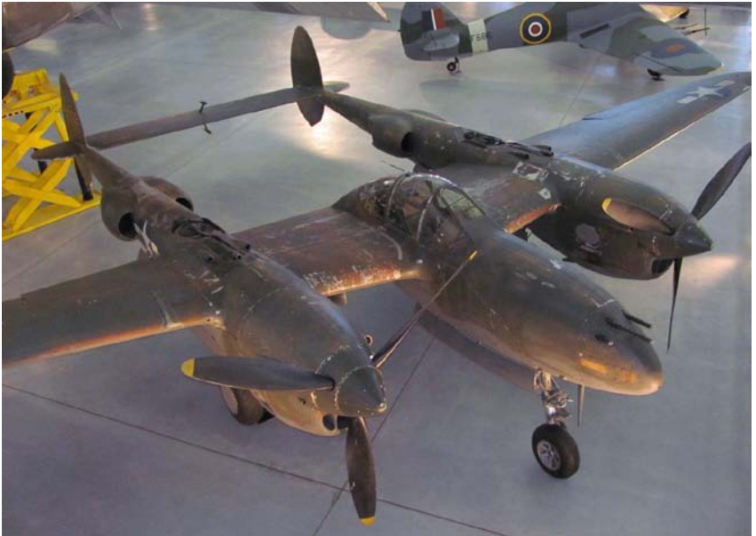
The counter-rotating propellers on this Lockheed P-38 Lightning are clearly visible. This aircraft is located in the Udvar-Hazy Center, near Washington D.C.
