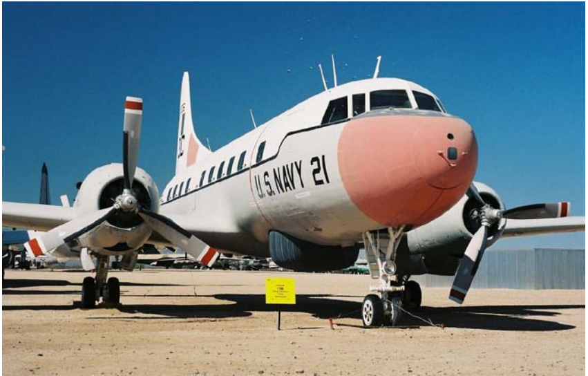
A USAF Convair T-29B Flying Classroom with square prop tips and de-icing boots on the props leading edges. This aircraft is stored at the Pima Air & Space Museum, Tucson, Ar.
