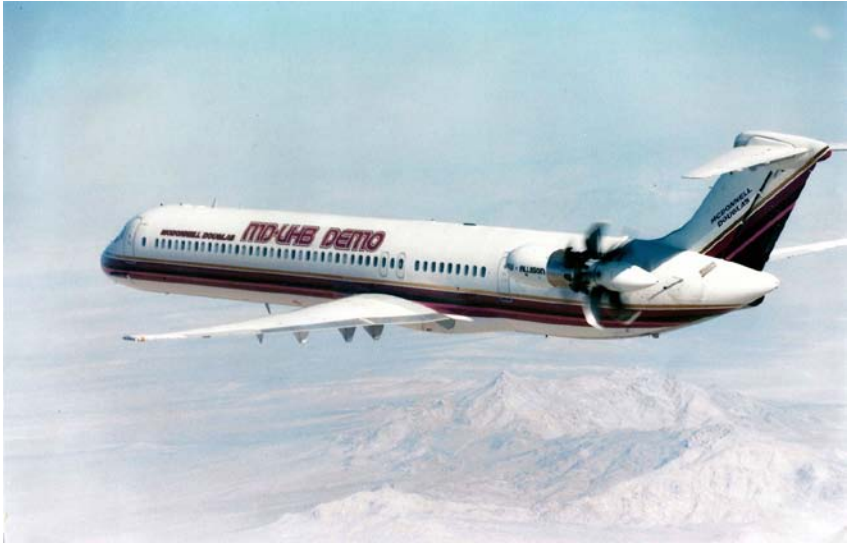
The McDonnell Douglas MD-80 flight-testing the P & W Allison Model 578-DX Propfan. Photo courtesy Hamilton Standard, Connecticut, USA.
