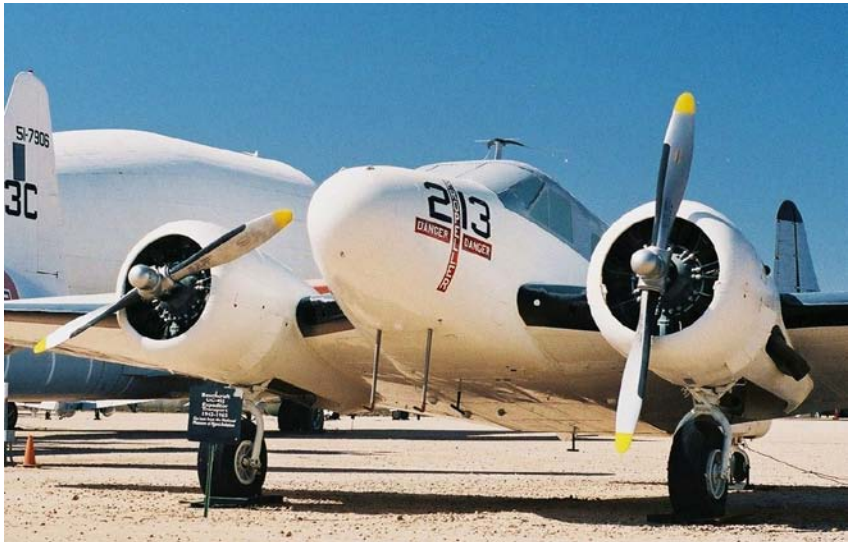
The Beech UC-45J Navigator has a pair of Hamilton Standard variable-pitch props each powered by a P&W Wasp 450 BHP engine. The Pima Air & Space Museum in Tucson, Arizona is home to this aircraft.
