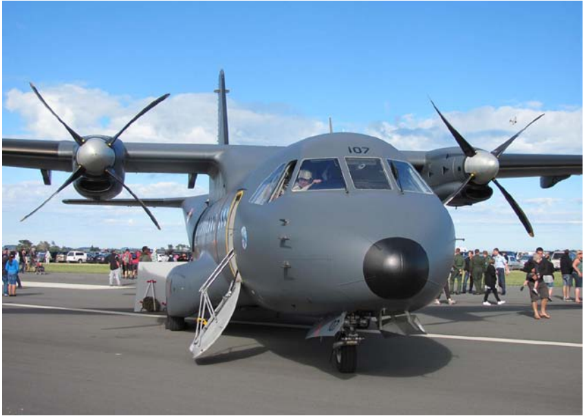
A CASA CN 235 transport parked with the props in the ground feathered position.
