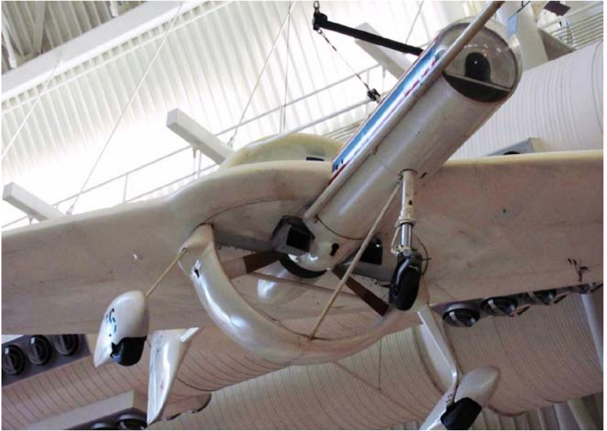
An Unmanned Aerial Vehicle (Drone) powered by a Ducted Fan. This UAV resides in the Udvar-Hazy Centre, Chantilly, Va.
