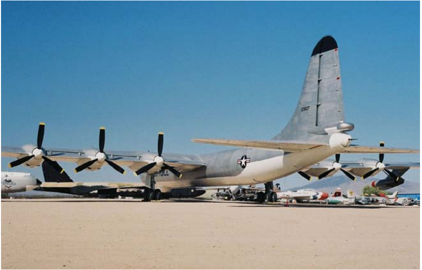
The Convair B-36J Peacemaker, the world's largest aircraft with pusher props. It has six P&W piston engines and four jet engines! The B-36 in this photo was the last one built, in 1956. It is on show at the Pima Air & Space Museum, Tucson, Ar.
