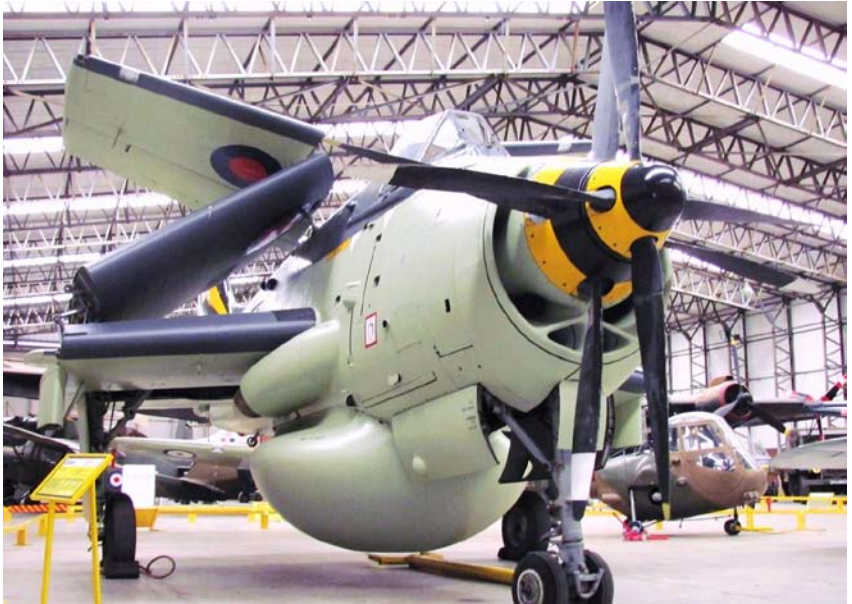
Contra-props mounted on the Fairey Gannett AEW3 in the Yorkshire Air Museum, Elvington, England.
