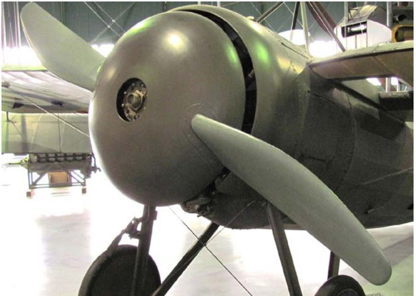
The Bristol M1c Bullet has a giant-size prop spinner looking very much like a doorbell. This aircraft is located in the RAF Hendon Museum, London.
