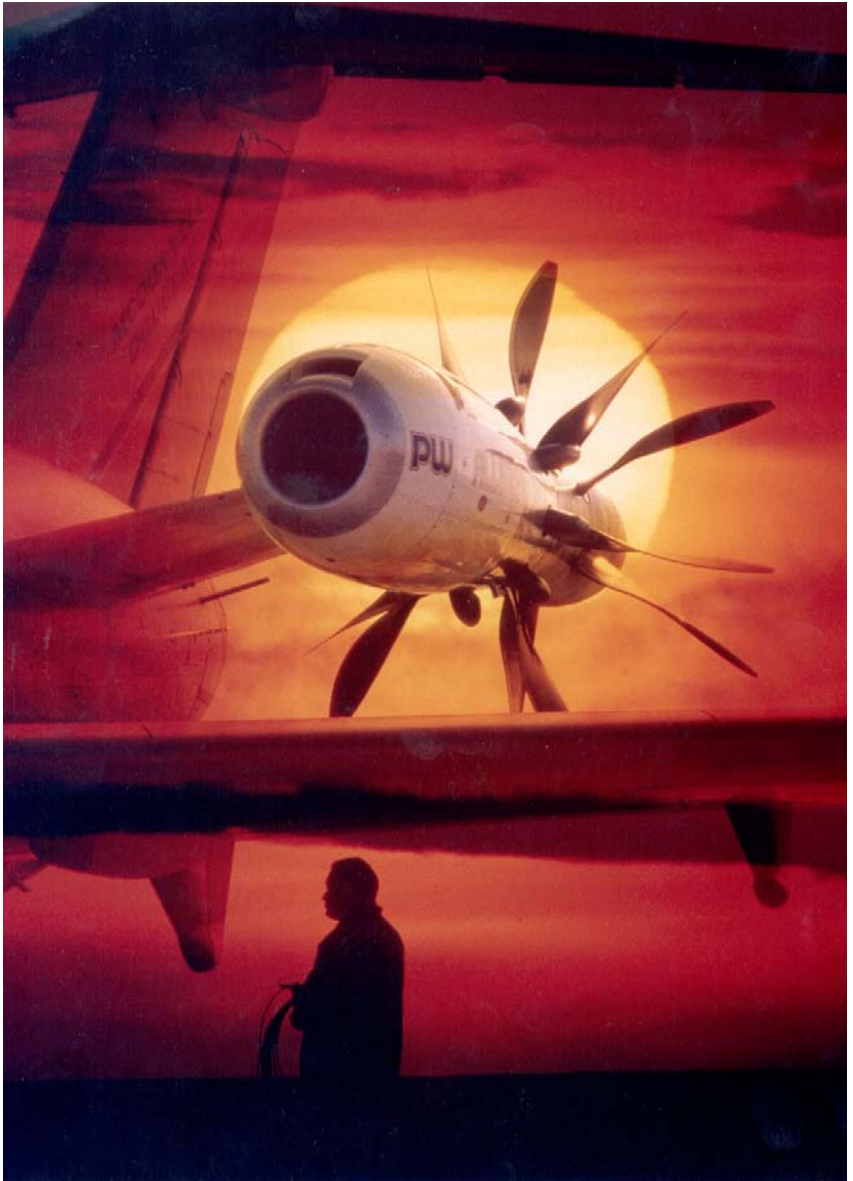
A dramatic double-exposure of the McDonnell Douglas MD-80 test-bed with the P&W Allison Model 578-DX Propfan, at sunset. Photo courtesy Hamilton Standard, Connecticut, USA.
