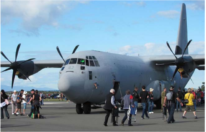
The Lockheed Hercules C130J with six-blade composite propellers. The Original C130A model had three-blade props.
