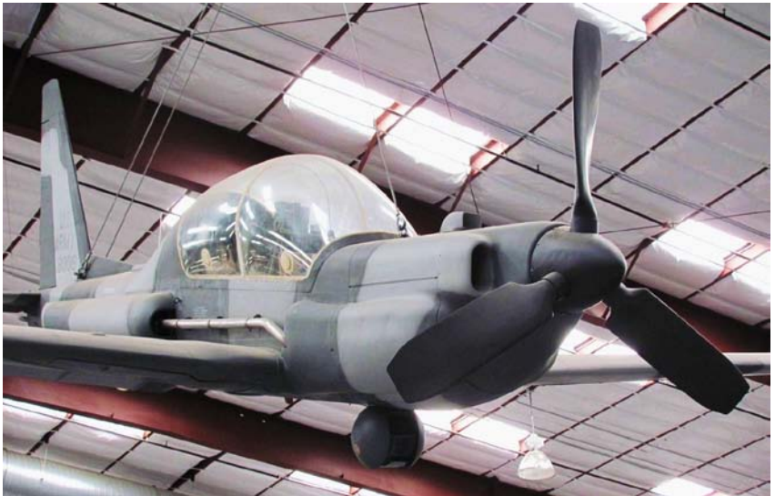
A Lockheed YO-3 Quiet Star observation aircraft, with a three-blade, wide chord prop. This is one of the quietest planes built due to the very quiet propeller and other features. It is housed in the Pima Air & Space Museum, Tucson, Ar.
