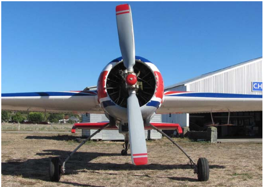
The Yak aerobatic aircraft fleet use centrifugal weights attached to the propeller to assist prop pitch change. This is a YAK 55m model.
