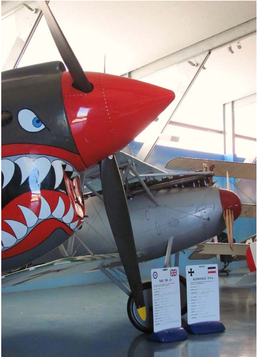
The pointed spinner of the Curtiss P-40 Kittyhawk contrasts with the blunt spinner on the Albatross DV.a.
