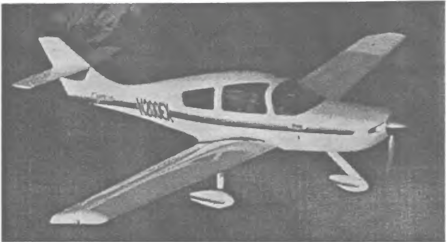
Figure E-1. The Wheeler Express is a sleek, all composite aircraft which is being built by a large number of homebuilders. The empennage flutter analysis is used as an example.
