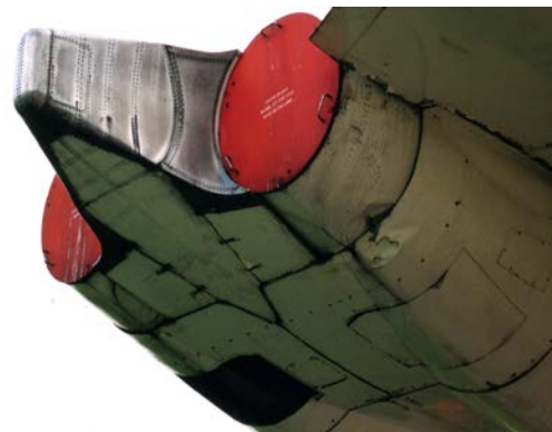
Figure 5.18 Modified Exhaust Configuration (Courtesy J. Hieminga)
