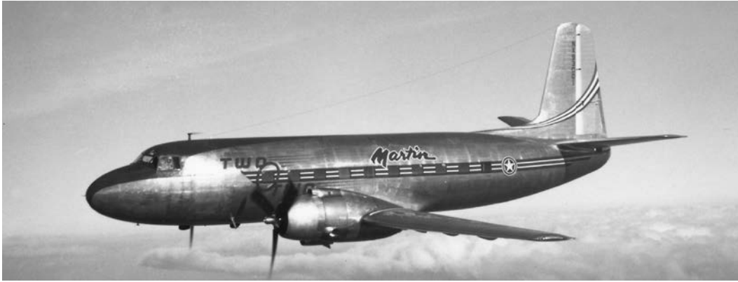
Figure 3.2 Martin 202, Before Dihedral Modification (Not accident aircraft, Courtesy Stan Piet)
