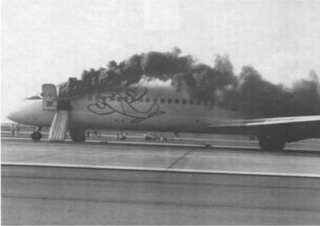
Figure 5.28 DC-9-32 after Uncontained Engine Failure (Courtesy NTSB)
