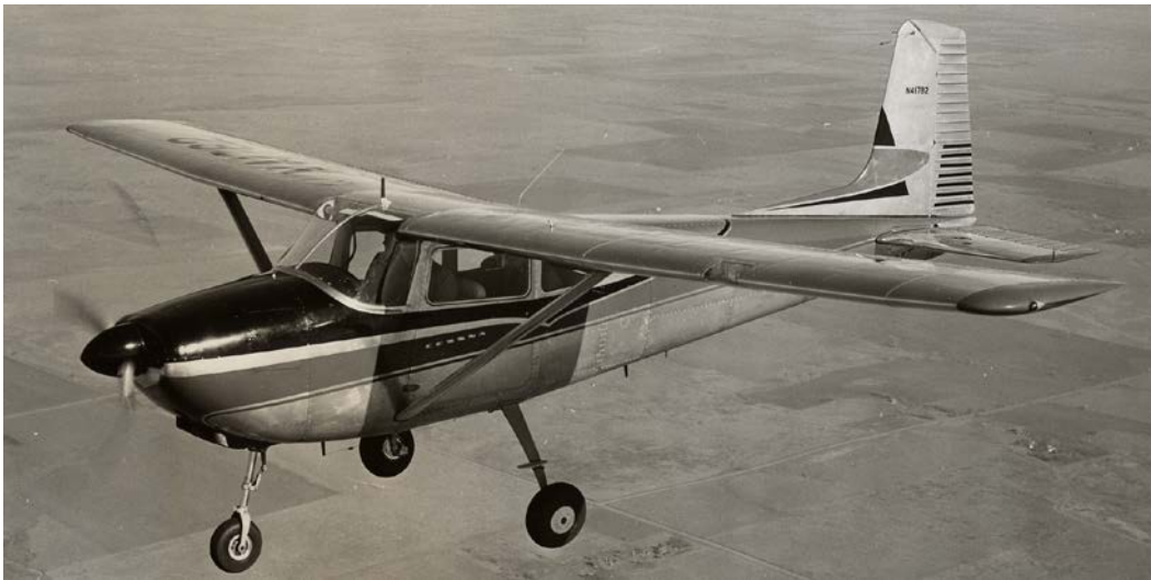
Figure 8.20 Cessna 172 with Unswept Vertical Tail (Courtesy Cessna)
