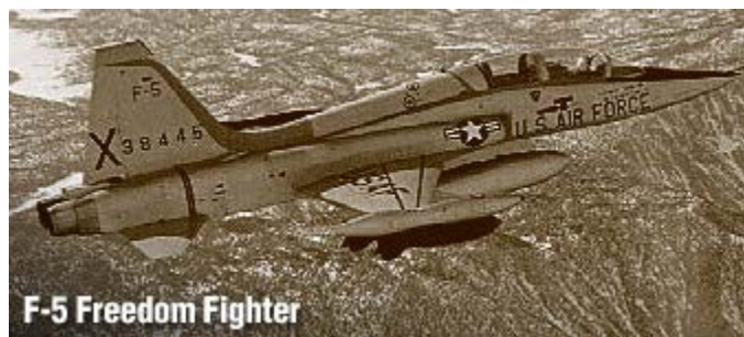
Figure 8.52 Northrop F-5 with Local Tip-tank-to-wing Area Ruling (Courtesy U.S. Air Force)
