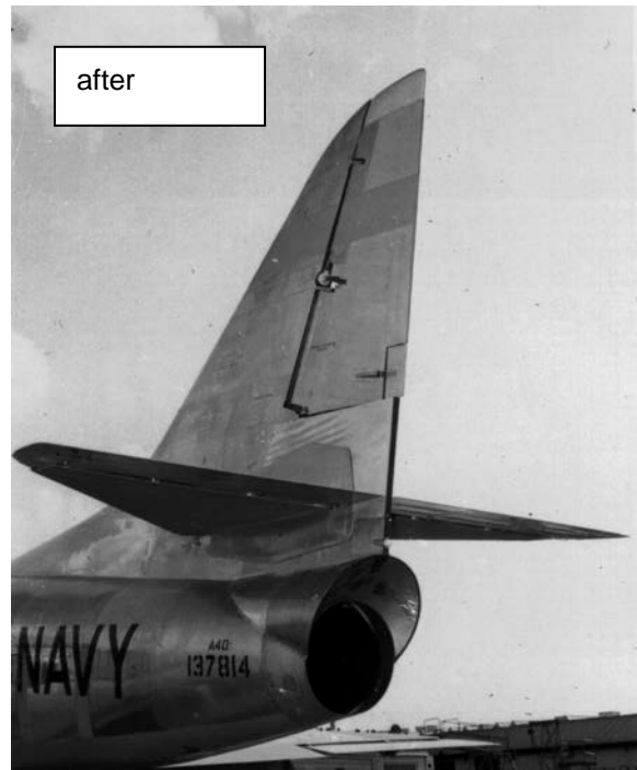
Figure 5.7 Sugar-scoop fairing as installed on the Douglas A4D Skyhawk (Courtesy San Diego Aerospace Museum)
