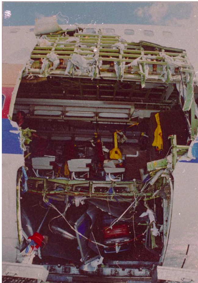
Figure 3.30 Damage Done by a Cargo Door Opening in Flight (Courtesy NTSB)
