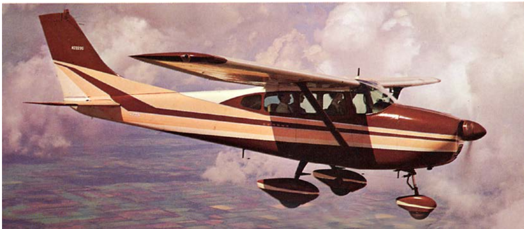
Figure 8.23 Cessna 172 with Swept Vertical Tail (Courtesy Cessna)
