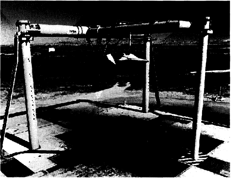
Figure CS2.26 ASTOVL Large Scale Powered Model (LSPM)—Hover Test at NASA Ames.
