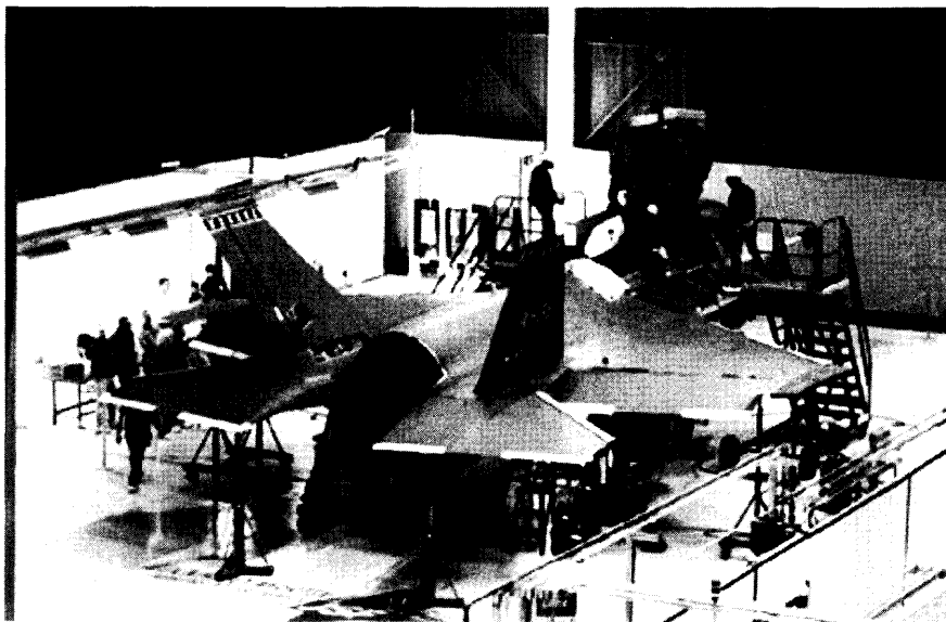
Figure CS2.41 The X-35A undergoing reconfiguration to the X-35B.
