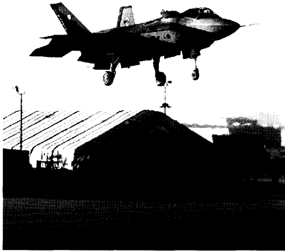
Figure CS2.43 First press up of ship 301 (STOVL) off the hover pit in Palmdale.
