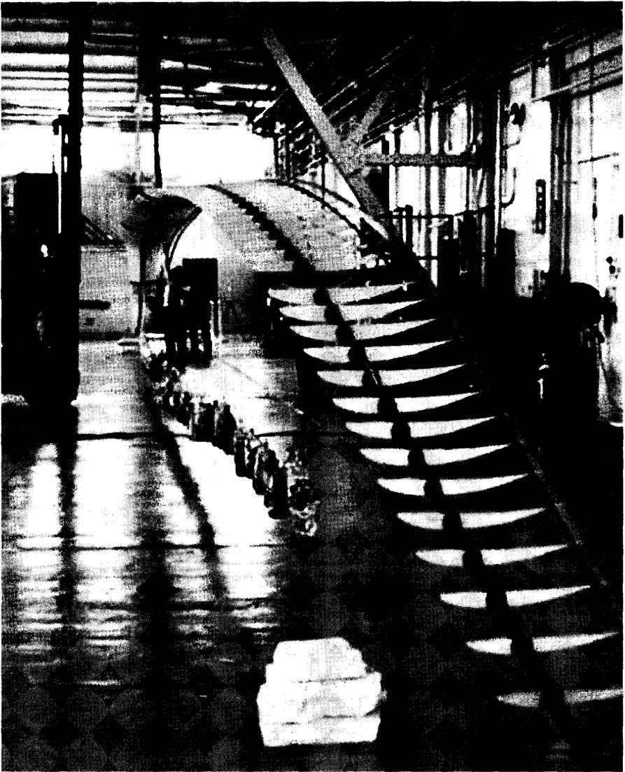
Figure CS6.25 Proof test for Daedalus wing structure in the hangar at Hanscom Field, MA. (Photo by Peggy Scott, 1987.)
