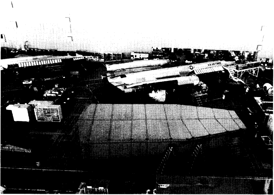
Figure CS1.14 A-12 production line; shipping container in foreground. (Lockheed Martin)
