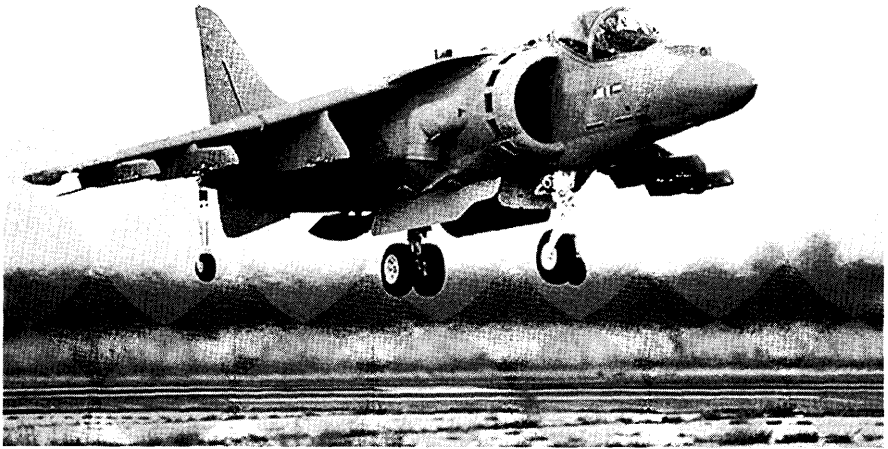
Figure CS2.7 AV-8B in hover showing the thrust vectoring nozzles directed nearly vertically downward.
