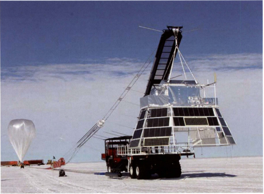
Launch apparatus for a high altitude scientific balloon with its payload module
