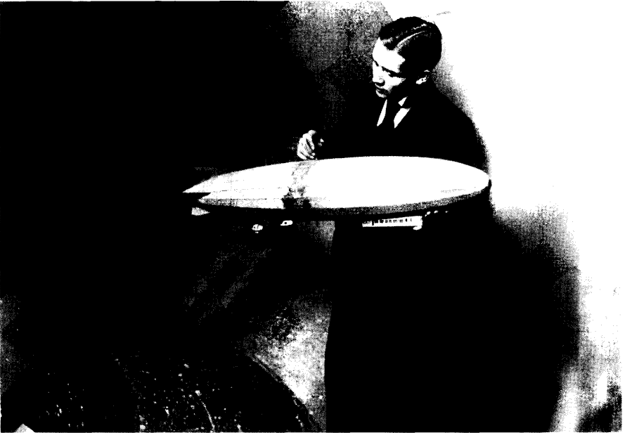
Figure 3.1 Göttingen wind tunnel model of LZ120 Bodensee airship (1918).
