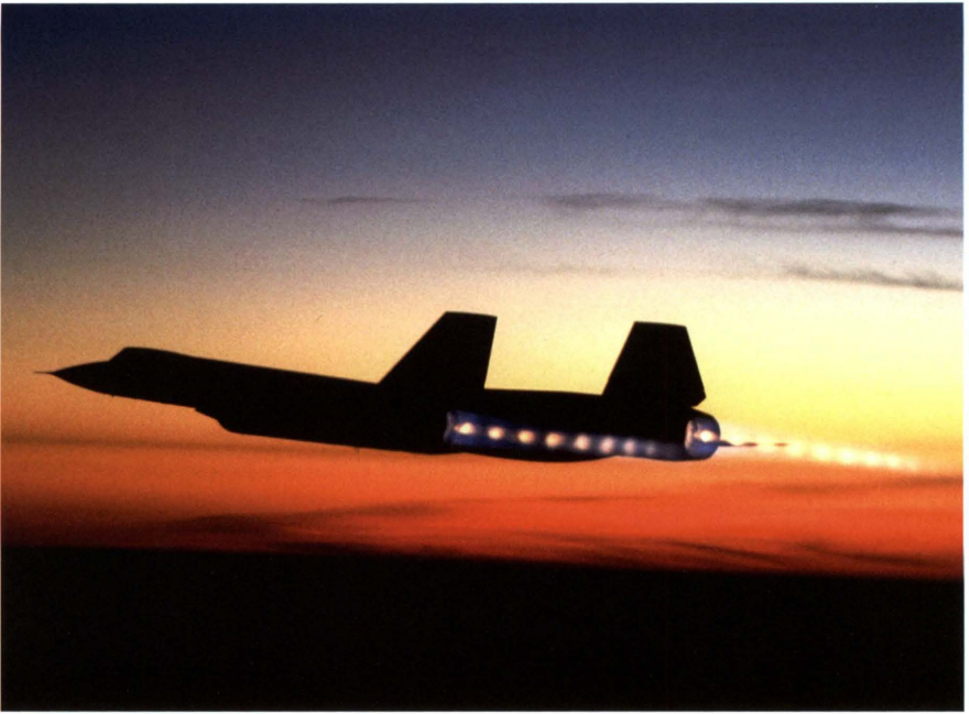
SR-71 showing Mach diamonds from a high power setting
