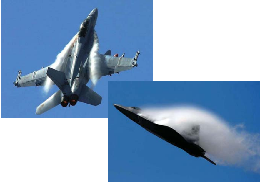
Fig. 2.14 Vortices Shedding from F-18 LEX and F-22 Wing Leading Edge
