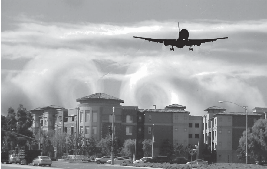
Figure 10.1 B-767 generates a strong trailing vortex system during a landing approach (courtesy of Ray Nicolai).
