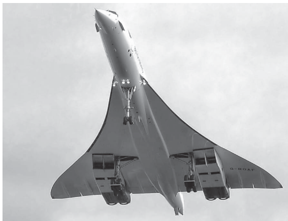
Figure 8.2 Concorde with nose drooped for landing (courtesy of Wikimedia Commons).
