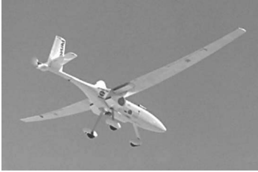
Figure 18.9 The Aurora Flight Systems Perseus UAV developed for NASA high altitude ozone measurements.
