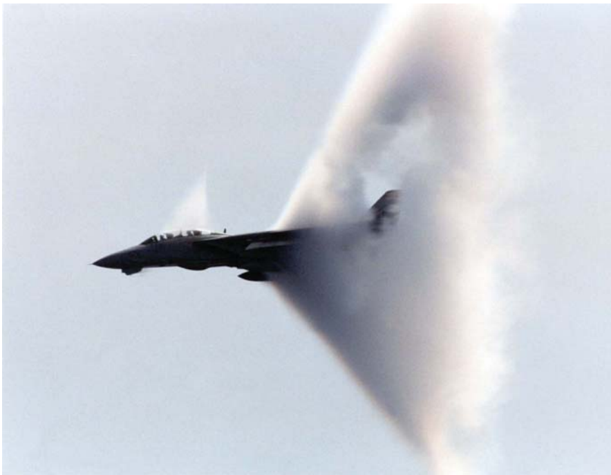
Ch. 2 F-14 with Shock Condensation @ M = 0.9
