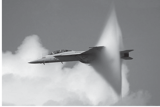
Figure 2.20 F-14 at M \sim 0.95 with condensation at trailing edge normal shock.
