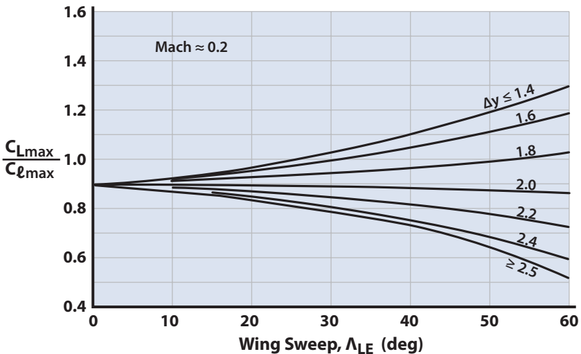
Figure 9.15 Subsonic maximum lift of high-AR wings (adapted [10]).
