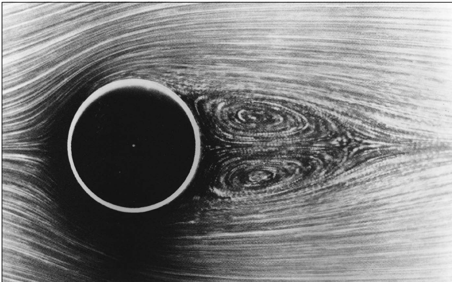
Figure 3.47 Flow over a circular cylinder. Re = 26 . (Source: Photograph by Sadatoshi Taneda, from Van Dyke, Milton, An Album of Fluid Motion , The Parabolic Press, Stanford, Calif., 1982.)
