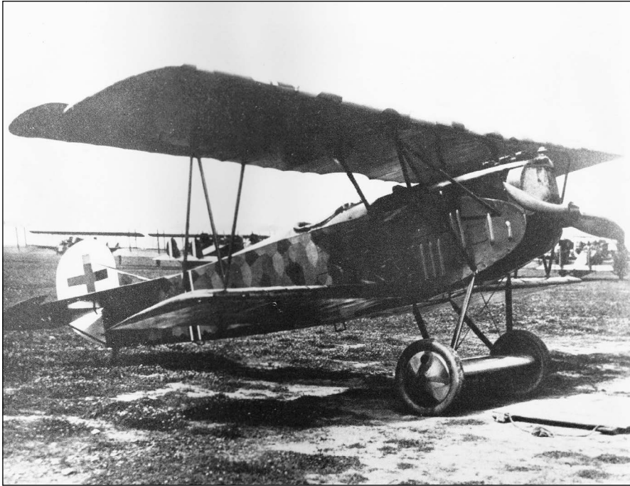
Figure 4.65 The World War I Fokker D-VII, one of the most effective fighters of the war, due in part to its superior aerodynamic performance allowed by a thick airfoil section. (Source: Loftin, Reference 48.)
