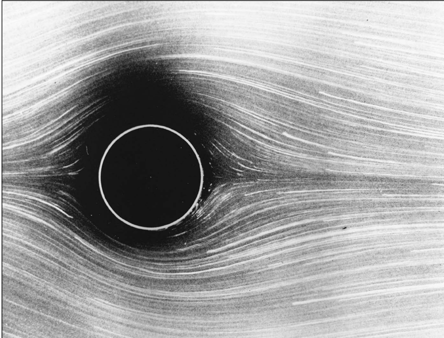
Figure 3.46 Flow over a circular cylinder. Re = 1.54 . (Source: Photograph by Sadatoshi Taneda, from Van Dyke, Milton, An Album of Fluid Motion , The Parabolic Press, Stanford, Calif., 1982.)
