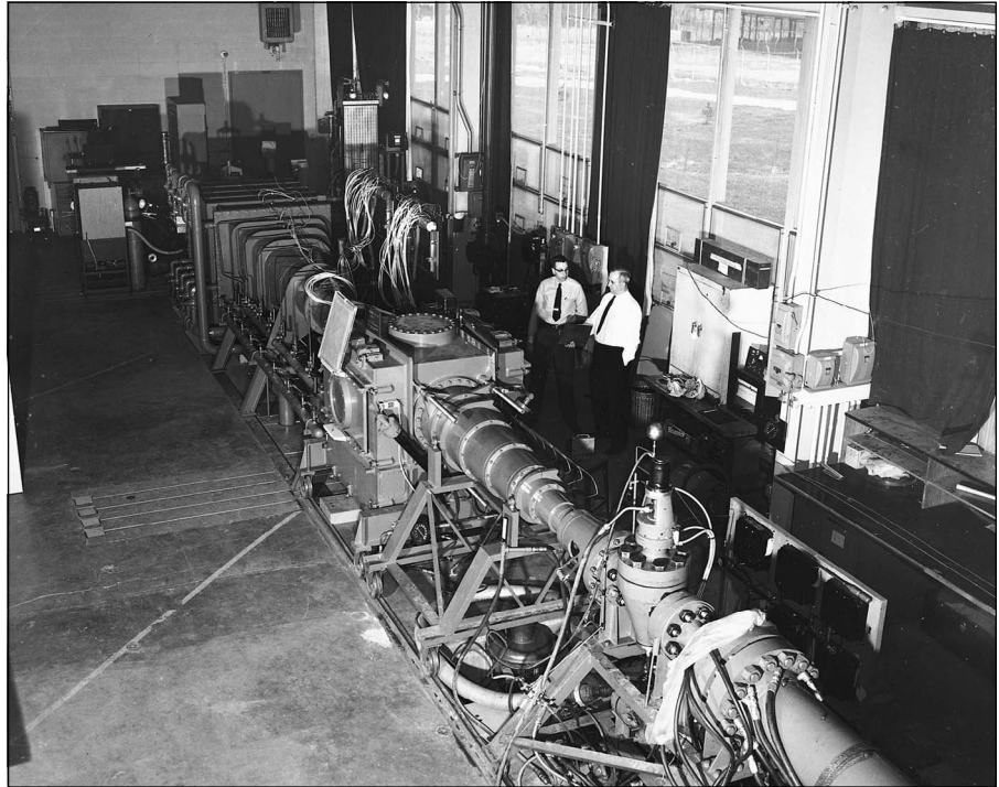
Figure 10.4 A large hypersonic wind tunnel at the U.S. Air Force Wright Aeronautical Laboratory, Dayton, Ohio. (Courtesy of the U.S. Air Force and the John Anderson Collection.)
