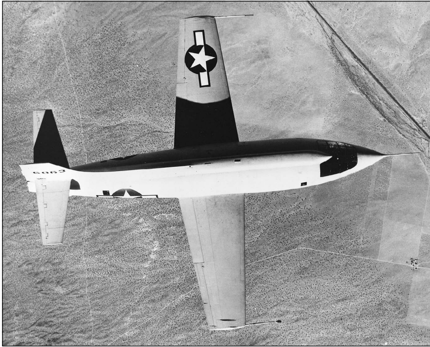
Figure 11.12 The Bell XS-1—the first manned airplane to fly faster than sound, October 14, 1947. (Courtesy of the National Air and Space Museum.)
