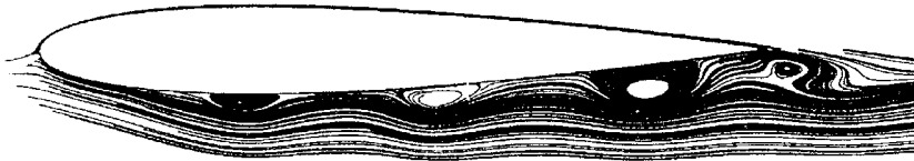
Figure 20.14 Streamline pattern over the bottom of an NACA 0012 airfoil, over which a series of jets is distributed which are alternatively blowing or sucking mass into or out of the flow, with the overall net mass injected into the flow being zero—a zero-mass jet array. (Data Source: Hassan and JanakiRam, Reference 91.)
