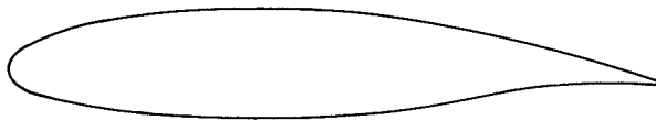
Figure 4.36 Profile for the NASA LS(1)-0417 airfoil. When first introduced, this airfoil was labeled the GA(W)-1 airfoil, a nomenclature which has now been superseded. (From Reference 16.)
