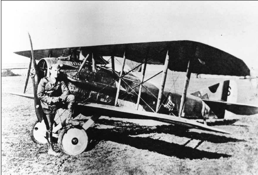
Figure 3.50 The French SPAD XIII, an example of a strut-and-wire biplane from World War I. Captain Eddie Rickenbacker is shown at the front of the airplane. (Courtesy of U.S. Air Force.)
