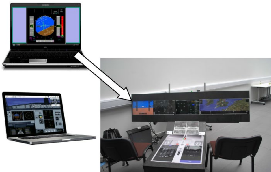
Figure 7.13 A VAPS model of cockpit displays and controls. VAPS was used to develop the displays for this model built by the Air Vehicle Design group project at Cranfield University (photo: Allan Seabridge).
