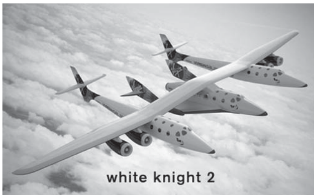
Figure 1.14 White Knight carrying Space Ship Two . Reproduced with permission of Virgin Atlantic.
