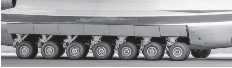
Figure 9.1 Antonov 225 (Mriya) main undercarriage.
