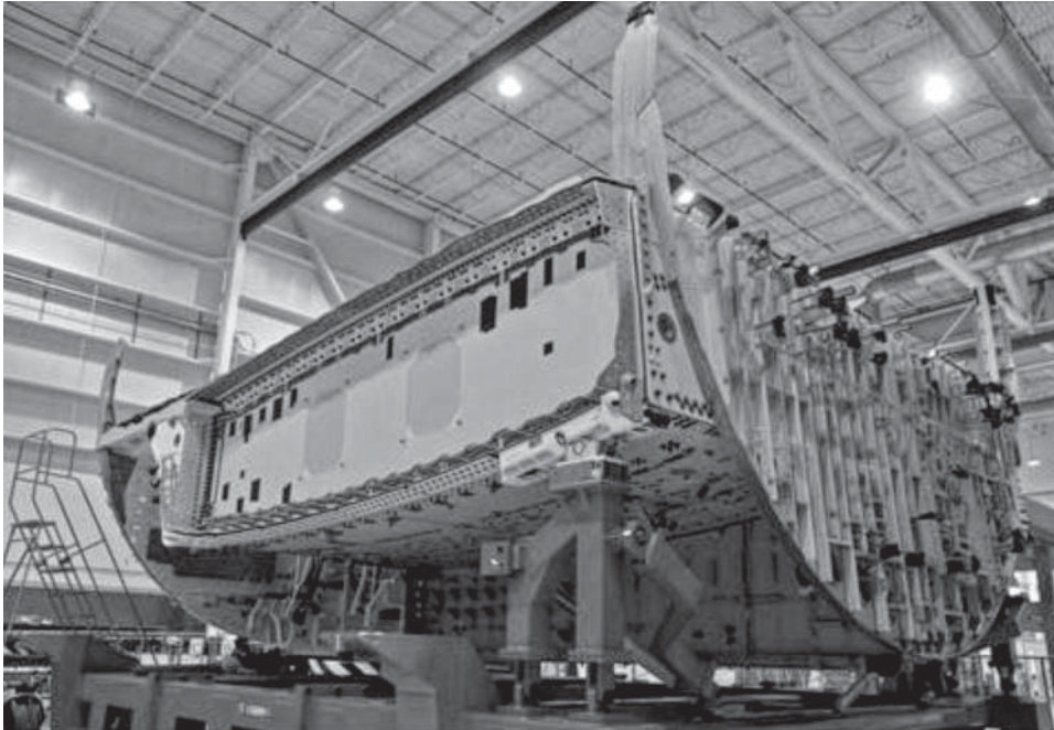
Figure 19.30 B787 wing-box structure. Courtesy Boeing.
