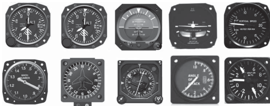
Figure 22.4 True-air data analogue indicating instruments. Top row: Airspeed indicator, altimeter, attitude indicator, turn-slip indicator, vertical speed. Bottom row: Mach meter, heading indicator, H-S indicator, angle of attack, g -meter. Reproduced with permission of Wiley Publisher.
