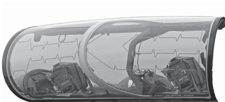
Figure 22.38 Detonation chord laid on canopy glass.
