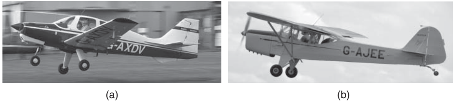
Figure 9.2 Three-point undercarriages. (a) Three-point tricycle (Beagle Pup) type. (b) Three-point tail wheel (Auster Aiglet) type.
