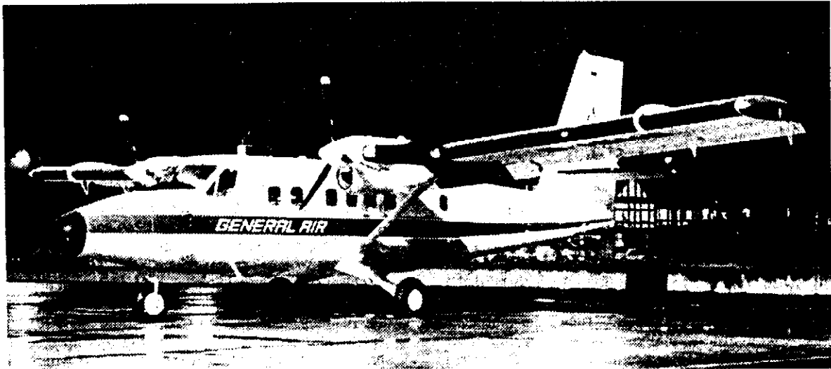
Fig. 8.1.2 Wing with external struts.
