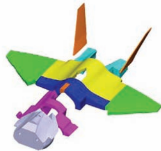
Plate 2 Joint strike fighter fuel tank layout (Courtesy of BAE Systems) (See Figure 3.10)
