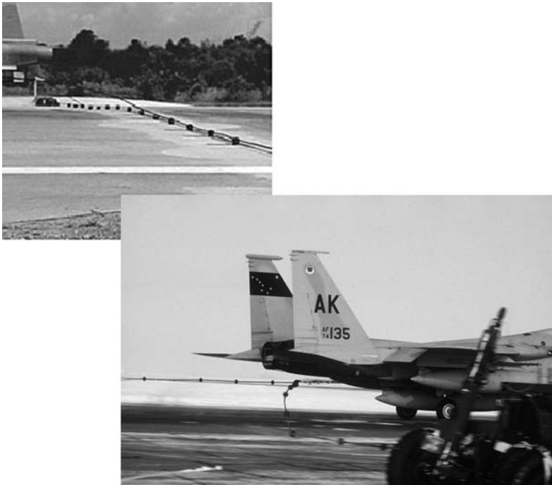
Figure 8.13 F-15 Eagle engaging the arresting system (DoD photo by TSGT Edward Boyce)
