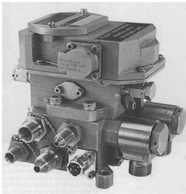
Figure 1.11 'Q' feel unit for GR5/AV8B (Courtesy of Smiths Group - now GE Aviation)
