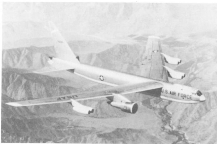
**Fig. 4.47** DC-10/CF6 installation on B-52 flying test bed.
