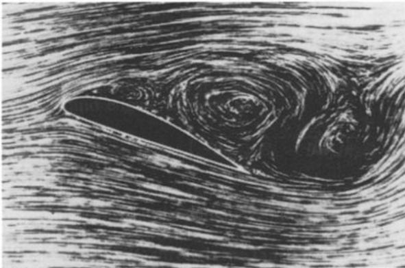
**c) Separated flow about an airfoil (from Prandtl).**
