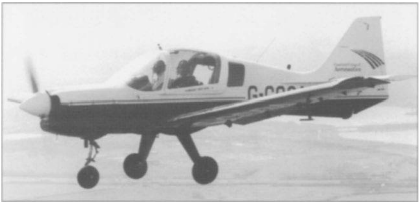
Figure 2.2 Nose powerplant - Scottish Aviation Bulldog
