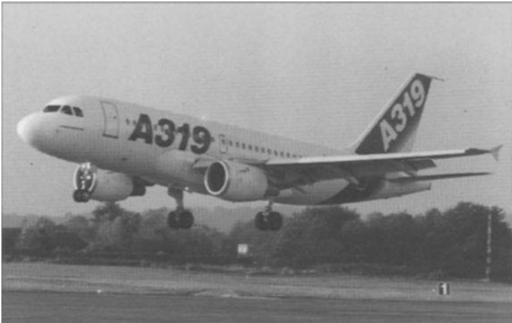
Figure 2.1 Conventional configuration - Airbus A319 Airliner
