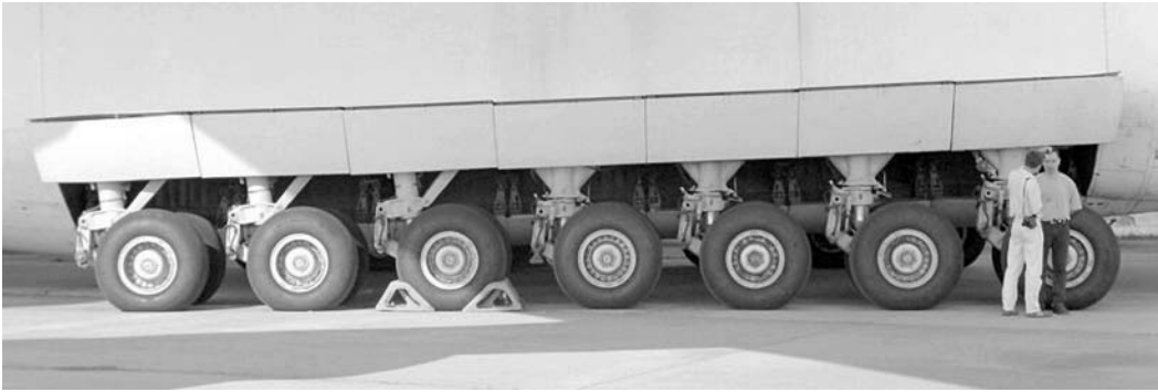
Figure 7.1. Antonov 225 (Mriya) main undercarriage
