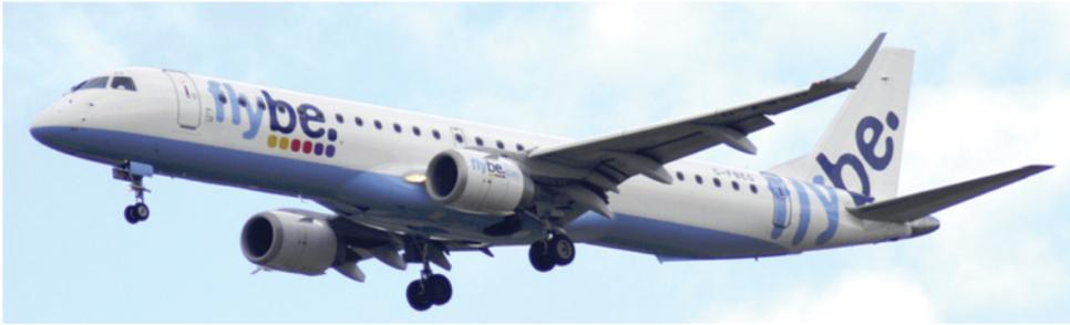
**Figure 9.11** Blended winglets on an Embraer ERJ 190-200LR (photograph by A. Sóbester).
