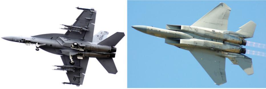
**Figure 8.3** Fighter jet planforms: low aspect ratio wings on the Boeing F/A-18E Super Hornet (left) and on the McDonnell Douglas F-15C Eagle (right). Note also the leading edge extensions on the Hornet (photographs by A. Sóbester).
