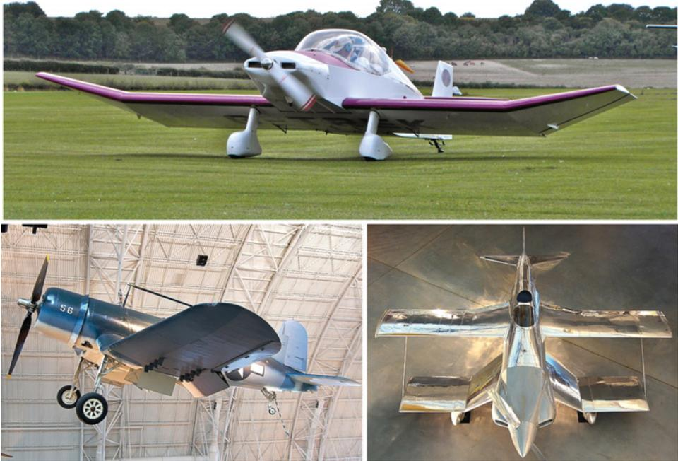
**Figure 9.2** Aircraft with polyhedral wings. Anticlockwise from top: Jodel D18, Vought F4U-1D Corsair and the Mahoney Sorceress, a staggered biplane designed for the Reno Air Races (photographs by A. Sóbester).
