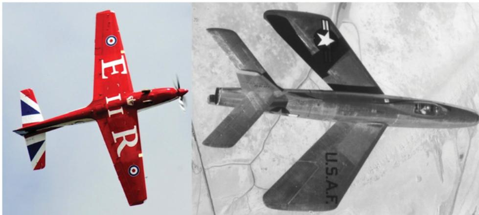
**Figure 8.4** Tapered wings. Sub-unity taper ratio on the Shorts Tucano (left,  $\lambda < 1$ ) and reverse taper ( $\lambda > 1$ ) on the wings of the Republic XF-91 Thunderceptor (photographs by A. Söbester and US Air Force).
