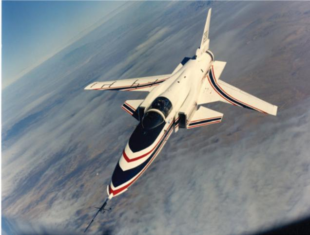
**Figure 8.5** Forward-swept outboard wing segments on the experimental Grumman X-29 (photograph by US Air Force).
