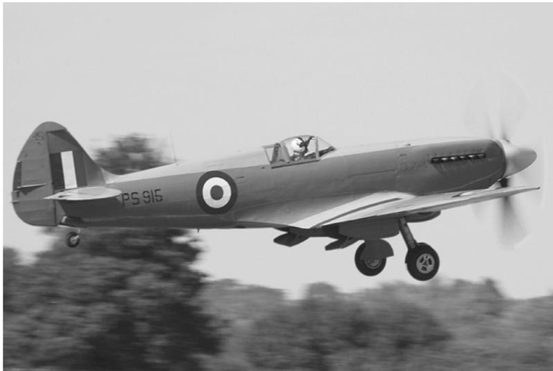
**Figure 6.3** The NACA 2213 was used on the Supermarine Spitfire, including on this Type 389 PR XIX, a late, Rolls-Royce Griffon-powered photo-reconnaissance version of the famous World War II fighter. With a top speed approaching 400 knots and a service ceiling in excess of 40 000 feet, the PR XIX was the highest performance Spitfire ever made (photograph by A. Sóbester).
