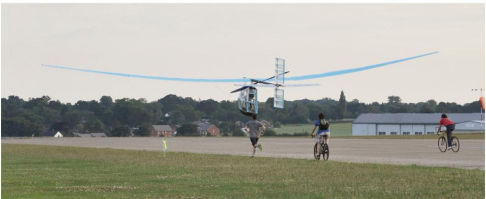
**Figure 12.2** SUHPA in flight. Note the high aspect ratio and low thickness/chord, highlighting the importance of the aero-structural trade-off (piloted by Bill Brooks; power-plant, Guy Martin; photograph by Fred To).
