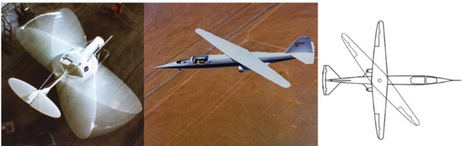
**Figure 8.13** NASA oblique wing aircraft: OWRA (Oblique Wing Research Aircraft) unmanned demonstrator (left) and the AD-1, a subsonic, manned research aircraft from 1979 (NASA images).
