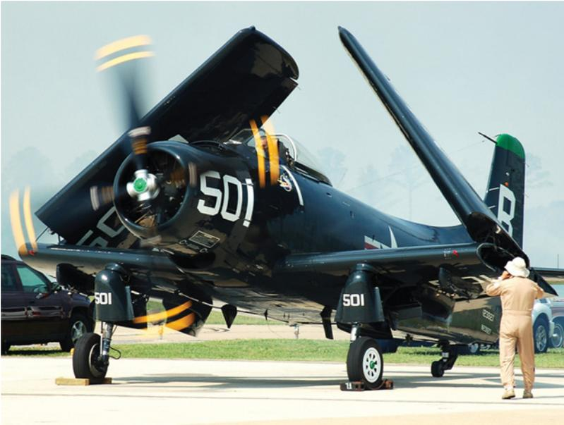
**Figure 6.4** NACA four-digit profiles over Korea and Vietnam. Weighing over 11 t and with a cruise speed of around 170 knots, the Douglas A1-D Skyraider (AD-4) is one of the real ‘bruisers’ of the history of propeller-driven attack aircraft. The folding wing shows off its NACA 2417 root section (photograph by A. Sóbester).
