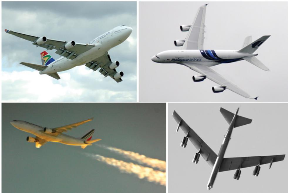
**Figure 8.2** Big jets with high aspect ratio wings. The wings of the Boeing 747-400 (top left, Group V, Code E, span ~55 m) and the Airbus A330 (bottom left, Group V, Code E) are visibly more slender than those of the Airbus A380 (top right, Group VI, Code F, span ~80 m), the latter designed up against the upper boundary of Group VI/Code F. There are fewer geometrical constraints on long-range, strategic bombers, such as the Boeing B-52 (bottom right) (photographs by A. Sóbester).
