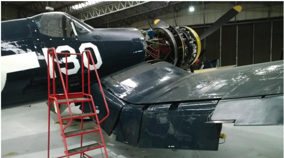
**Figure 9.3** Multisegment flaps on the polyhedral wing of a Vought Corsair (photograph by A. Sóbester).
