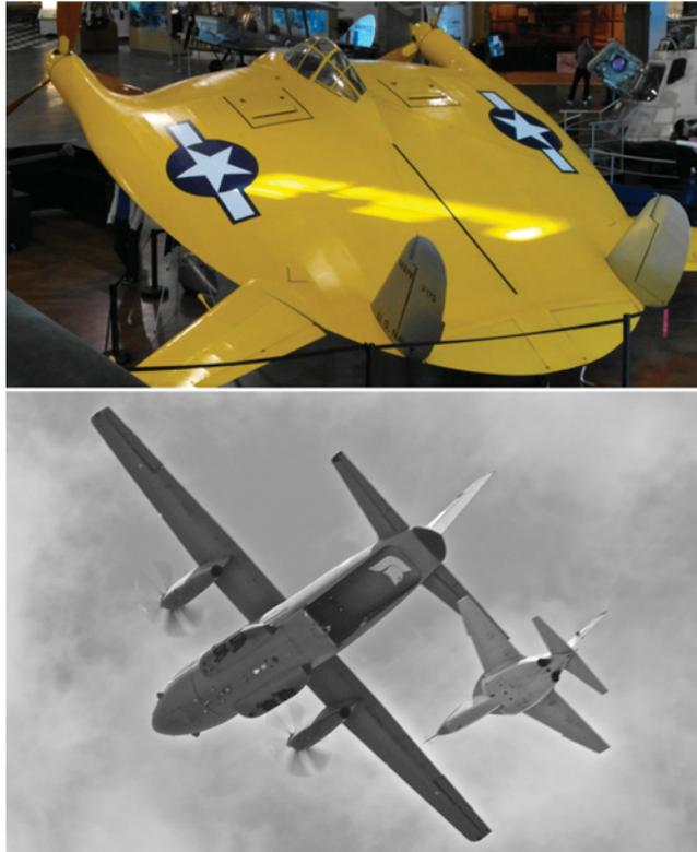
**Figure 8.1** Aspect ratios from the extremely low – the Vought V-173 ‘Flying Pancake’ (just over one!), with wingtip-mounted propellers – to high – the Alenia C-27J Spartan, bottom left – and low – Alenia Aermacchi M-346 Master (photographs by A. Sóbester).
