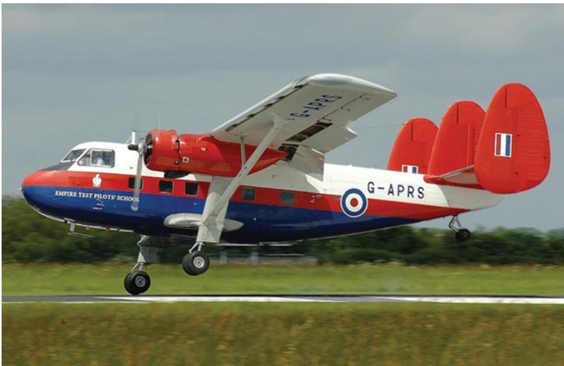
**Figure 6.5** The Scottish Aviation Twin Pioneer, a short take-off and landing transporter designed in the 1950s, had wings featuring NACA 4415 profiles (photograph by A. Sóbester).
