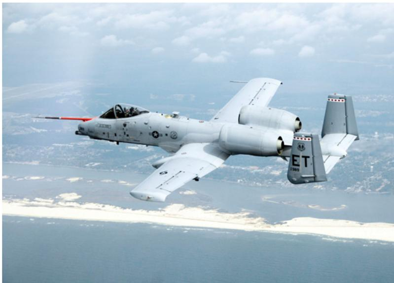
**Figure 6.6** The Fairchild Republic A-10 Thunderbolt II may be the only jet aircraft with wings based on NACA four-digit sections – a NACA 6716 at the root and a NACA 6713 at the tip (photograph courtesy of the US Air Force).
