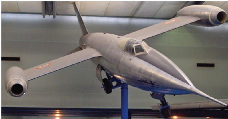
**Figure 8.7** SNCASO Trident I. This 1950s experimental aircraft powered by turbojets and a rocket was able to achieve Mach 1.55 in spite of having zero sweep (photograph by A. Sóbester).
