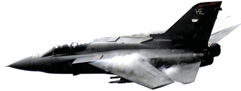
**Figure 8.12** Panavia Tornado ADV (F3), a Mach 2.2 long-range variable-sweep interceptor with its wings at  $\Lambda = 67^\circ$ , their highest sweep setting, the lowest being  $\Lambda = 25^\circ$  (photograph by A. Sóbester).
